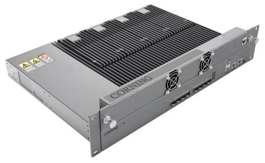
The E62-A3 – Access Unit Chassis is a standard 19-inch 2U rack-mounted shelf (1U fan unit included), which serves as the host for Everon<sup>™</sup> 6200. The E62-A3 provides coupling access to radio signal sources of multi-operator, multi-system, and multi-band, forming digital optical signals and distributing static capacity distribution to fiber-connected other type devices. One A3 supports up to eight optical interfaces connected to E3s (Expansion Unit) or N3RUs (Remote Unit).
