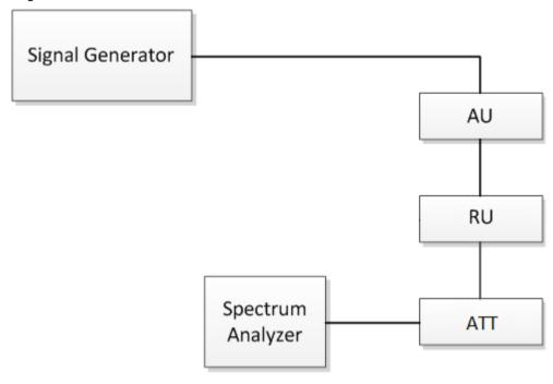
Fig.4. Occupied bandwidth test configuration
