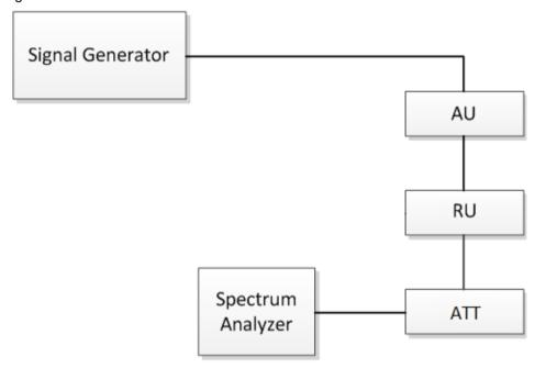
Fig.2. Conducted Spurious Emissions test configuration
