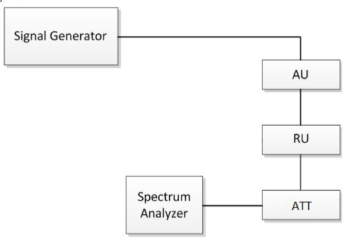
Fig.5. Out of Band rejection test configuration
