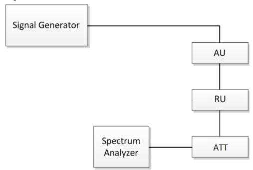
Fig.1 RF Output Power test configuration
