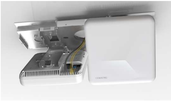
Figure 79. Top Panel of E62-N2RU Exposed
