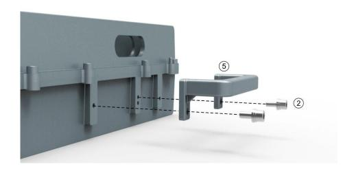
2. Attach and fasten the Bracket I to the left side of M2RU with screws M6×14 using T5 Wrench.
