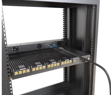
3. Fan DC version has power cable embedded in chassis. Note: Red is for positive; Blue is for negative.
