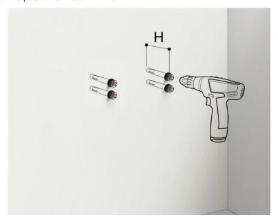
5. Attach the dowels, expansion screws or the like and fasten the Bracket II to the wall.
