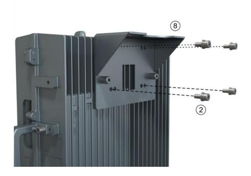
3. Mark the position of the drilling holes in the mounting Bracket II. Note: R = 13 mm.
