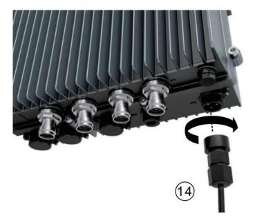
9. Connect and screw the ground cable at the M2RU's left side.
