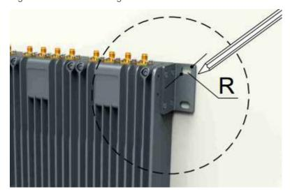
Drill 4 holes at the marked sites using percussion drill and embed 4×10 plastic expansion pipes. 3.
