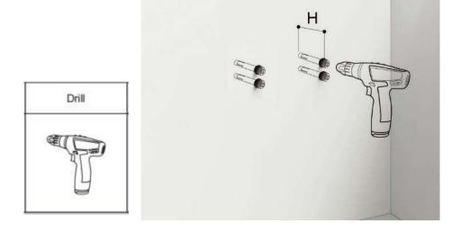
5. Attach the dowels, expansion screws or the like, and fasten the Bracket II to the wall.
