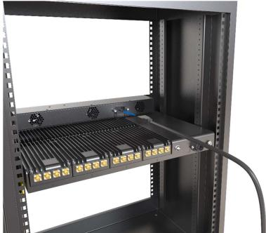
3. Fan DC version has power cable embedded in chassis.
