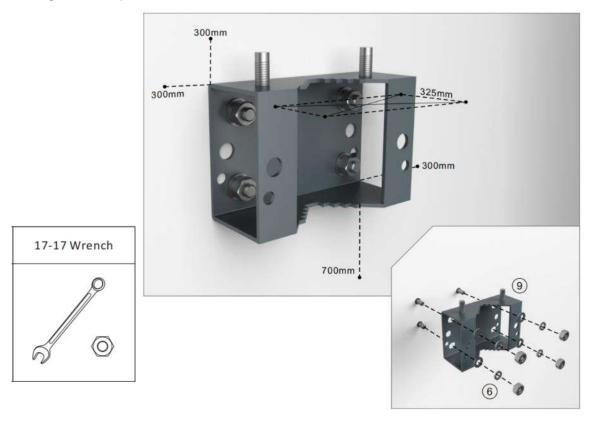
6. Hang the M2RU on the mounting Bracket II and fasten with nuts M10.
