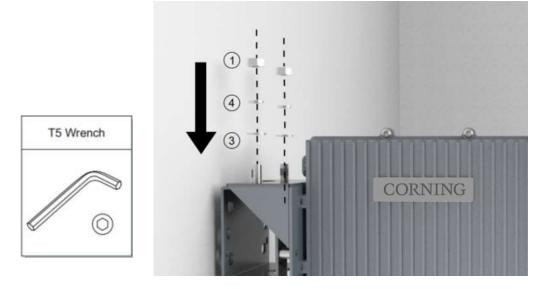
7. Fasten the Bracket I and II with screws M6×14.
