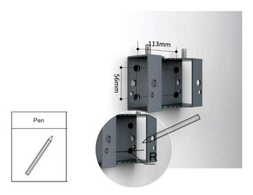
4. Drill 4 holes at the marked positions. Note: H = 70 mm
