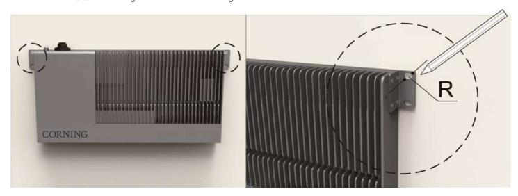
3. Drill 4 holes at the marked sites using percussion drill and embed 4×∅10 plastic expansion pipes. Note: H = 70 mm. Fasten the case with 4×M6 expansion bolt.
