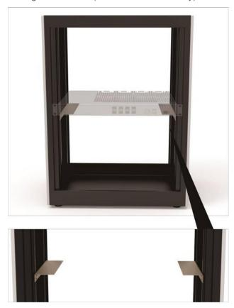
3. Place the AU in the rack and secure the AU using 2 screws M6x16 on both side and the Phillips screwdriver.
