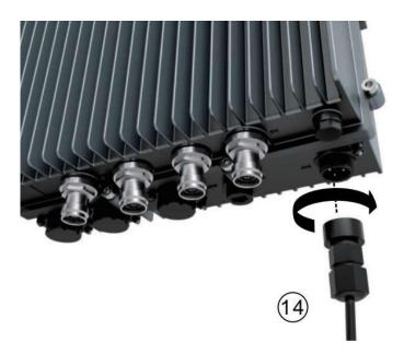
9. Connect and screw the ground cable at the M2RU left side.
