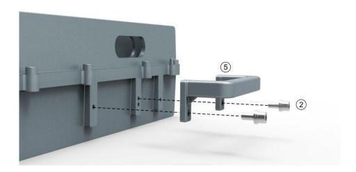
2. Attach and fasten the Bracket I to the back of M2RU with screws M6x14 using T5 Wrench.
