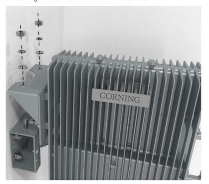
7. Fasten the Bracket I and II with screws M6x14.
