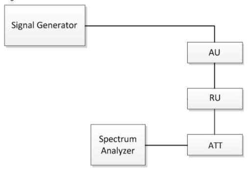
Fig.4. Occupied bandwidth test configuration
