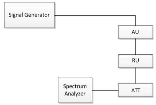
Fig.1. AGC Threshold Level test configuration
