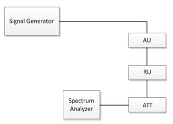
Fig.8. Noise/emission at Antenna Terminal
