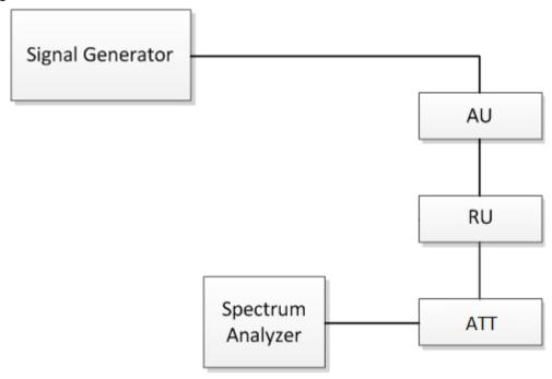
Fig.5. Out of Band rejection test configuration
