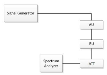
Fig.6. Out-of-band/out-of-block (including intermodulation) Emissions and Spurious
