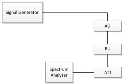
Fig.1 RF Output Power test configuration
