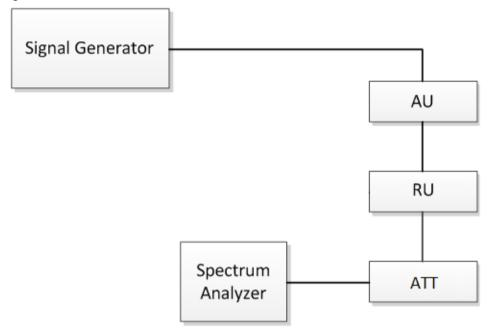
Fig.2. Conducted Spurious Emissions test configuration
