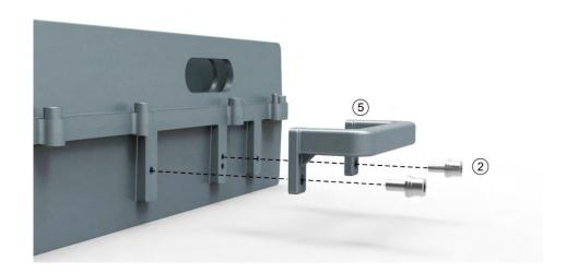
2. Attach and fasten the Bracket I to the left side of HPRU with screws M6×14 using T5 Wrench.
