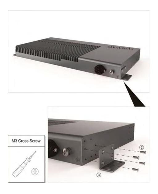
2. Mark 4 x  $\emptyset$ 6.8 mm drilling holes sites for the hanger to be attached to the wall.
