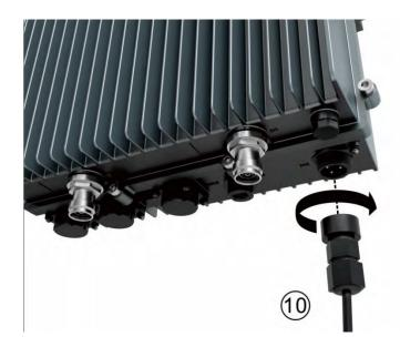
9. Connect and screw the ground cable at the HPRU's left side.
