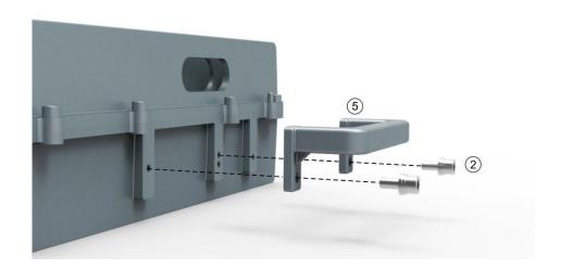
2. Attach and fasten the Bracket I to the back of H2RU with screws M6×14 using T5 Wrench.
