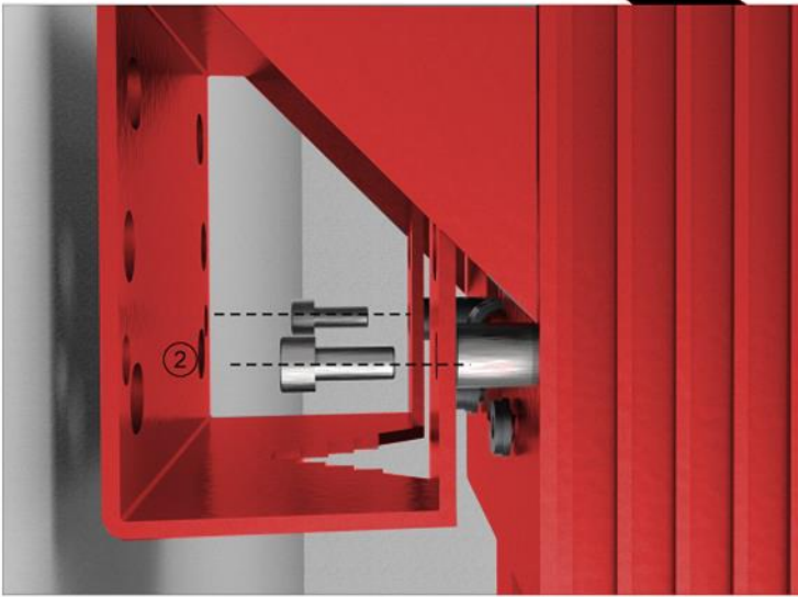
Fasten with 2xM6x14 screws.
