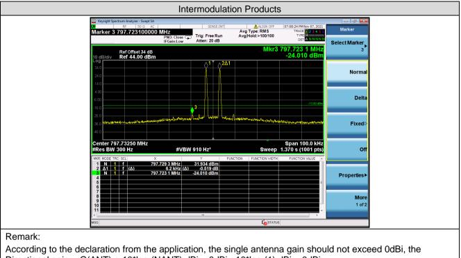
Directional gain =  $G(ANT) + 10^{*}log(NANT) dBi = 0dBi + 10^{*}log(1) dBi = 0dBi.$
