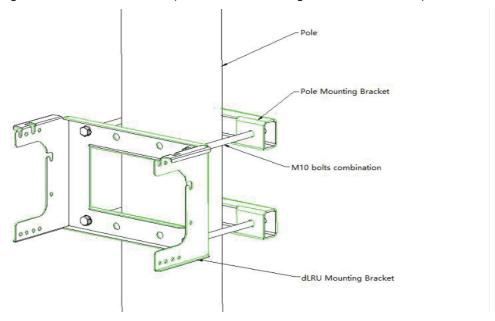
Figure 48. Pole-Mounting Diagram
