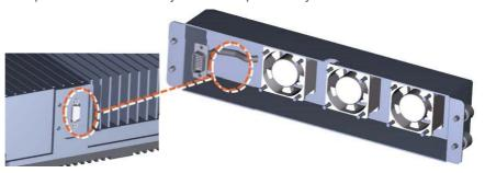
Figure 68. Fan Connection with DB15
