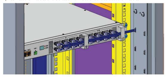
Figure 26. RIU Rack Installation with Cables
