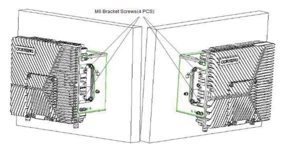
Figure 46. M6 Bracket Screw Holes
