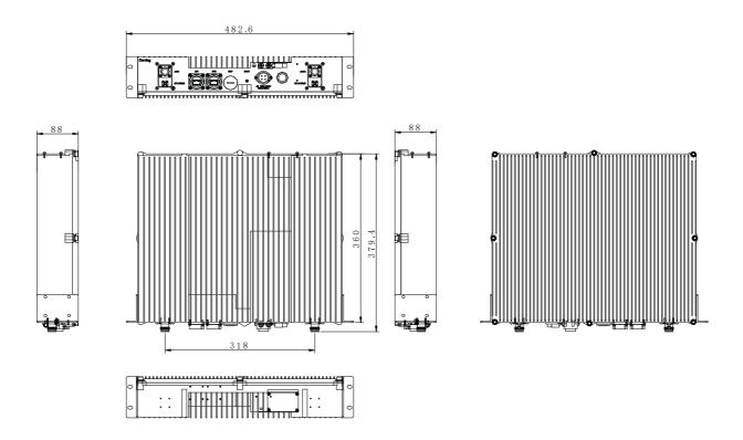
Figure 61. DMRU Dimensions - Without a Fan
