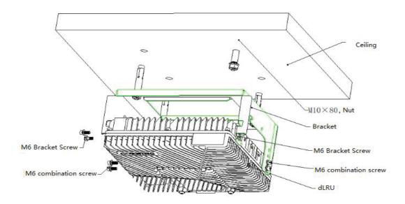
Figure 40. Single Unit Ceiling Installation
