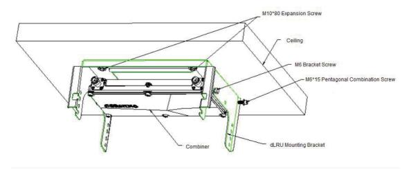
Figure 44. Combiner Installation Diagram
