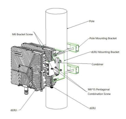
Figure 52. Dual Unit Installation Diagram
