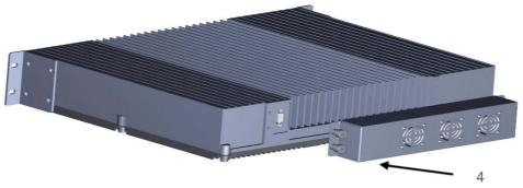
Figure 69. Fan Installation
