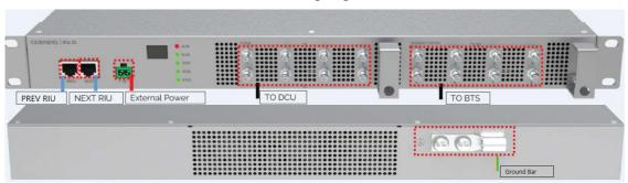
Figure 27. RIU Cable Connection
