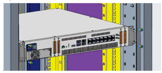
Figure 29. Installation Diagram of DCU in the Rack
