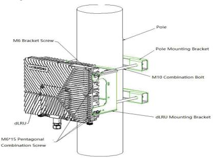
Figure 49. Diagram of Pole Installation for Single Unit
