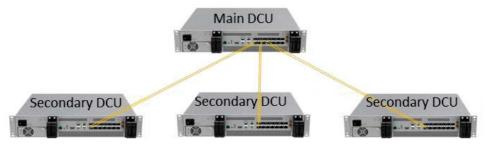
Figure 10. DCU Star Connection
