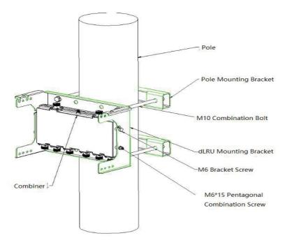
Figure 50. Installation Diagram of the Combiner
