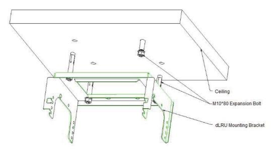
Figure 43. Mounting Bracket Installation Diagram
