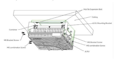
Figure 45. Low-Band dLRU Installation
