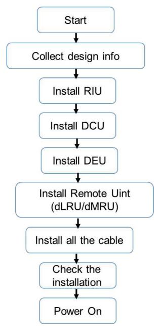
Figure 23. The Installation Process
