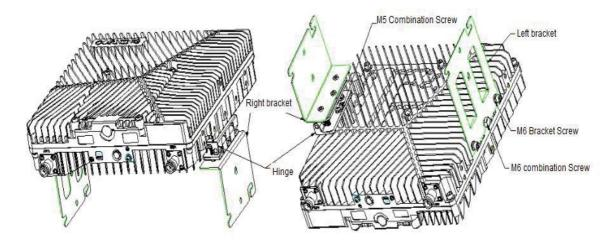
Figure 42. Installation of the Left and Right Brackets and Device Bracket
