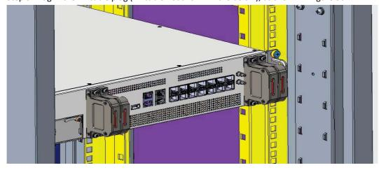
Figure 30. DCU RF Cable Plug Installation
