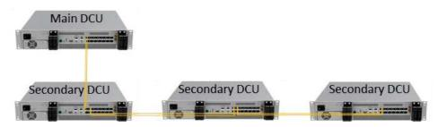
Figure 11.DCU Daisy Connection
