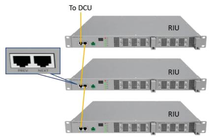
Figure 6. RIU Monitoring Diagram
