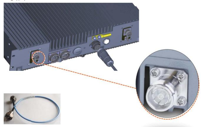
Figure 72. Antenna Connection
