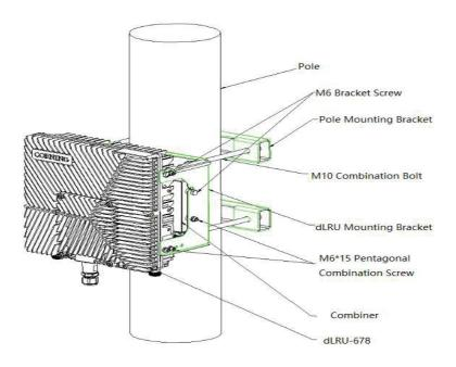
Figure 51. Installation Diagram of dLRU Pole
