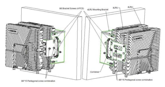
Figure 47. dLRU Installation Diagram
