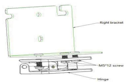
Figure 41. Right Bracket and Hinge Installation
