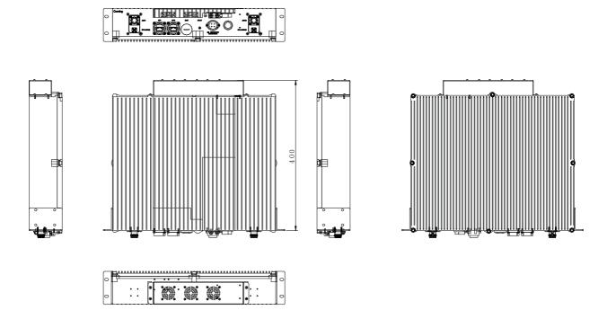
Figure 62. DMRU Dimensions - with Fan
