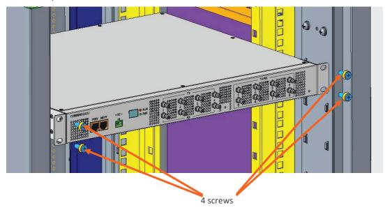
Figure 22. RIU Rack Installation
