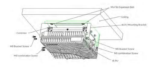
Figure 46 Low band dLRU installation
