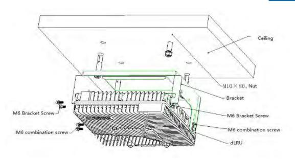
Figure 41 Single unit ceiling installation
