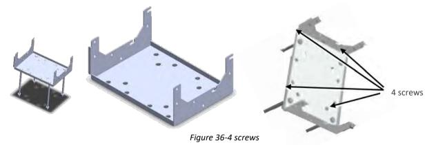
2) mount the LRU on the bracket with 4 screws.
