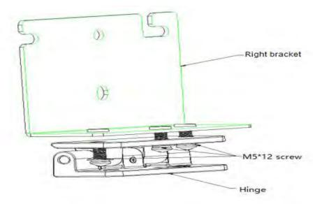
Figure 42 Right bracket and hinge installation
