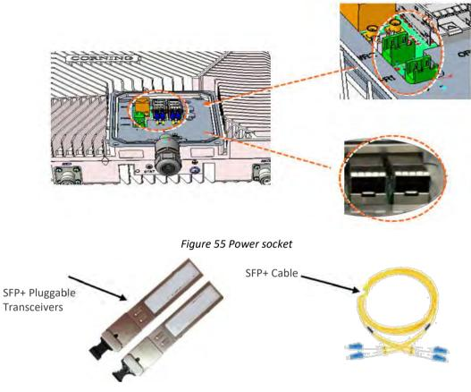
Figure 56 Remove rubber plug from the port and insert the SFP+ Pluggable Transceivers (hot-pluggable optical transceiver module) into it.
