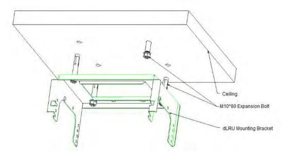
Figure 44 Mounting bracket installation diagram
