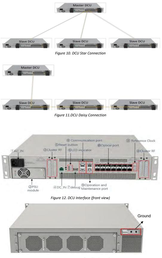
Figure 13. DCU interface (back view)
