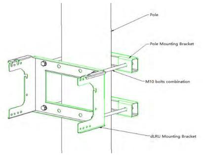
Figure 49 Pole mounting diagram
