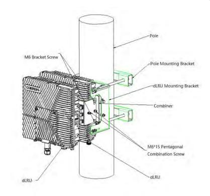
Figure 53 Dual unit installation diagram
