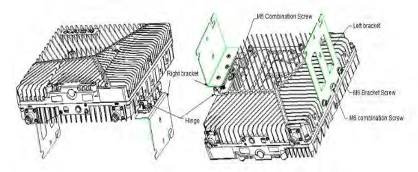
Figure 43 Installation of the left and right brackets and device bracket
