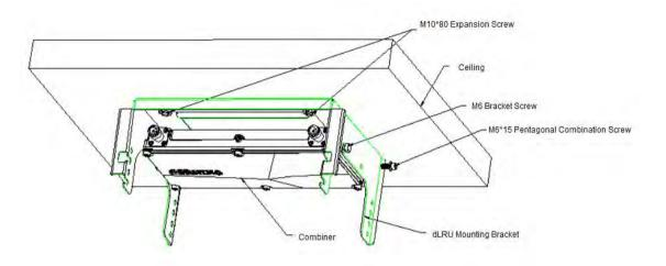
Figure 45 Combiner installation diagram
