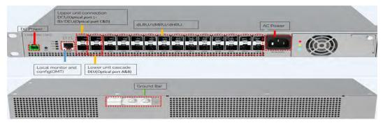
Figure 35 DEU cable connection
