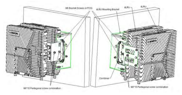
Figure 48 dLRU installation diagram
