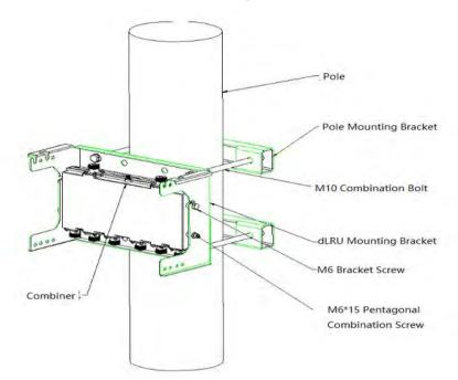
Figure 51 Installation diagram of the combiner
