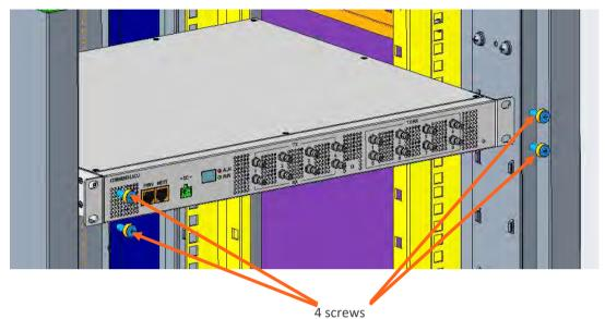
Figure 26. RIU rack Installation
