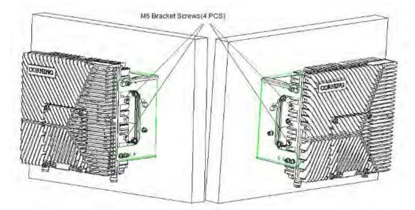
Figure 47 M6 bracket screw holes
