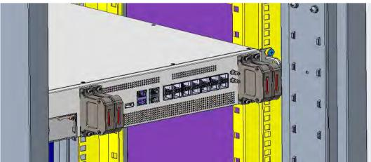
Figure 31 DCU RF cable plug installation
