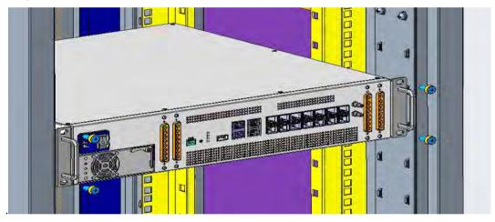
Figure 30 Installation diagram of DCU in the Rack
