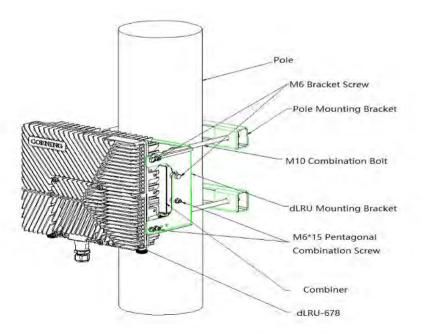
Figure 52 Installation diagram of dLRU pole
