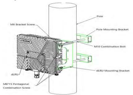
Figure 50 Diagram of pole installation for single unit
