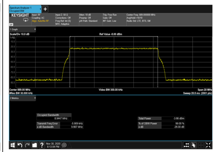
Figure 339: 64QAM 10MHz; 889.0MHz Input 4G
