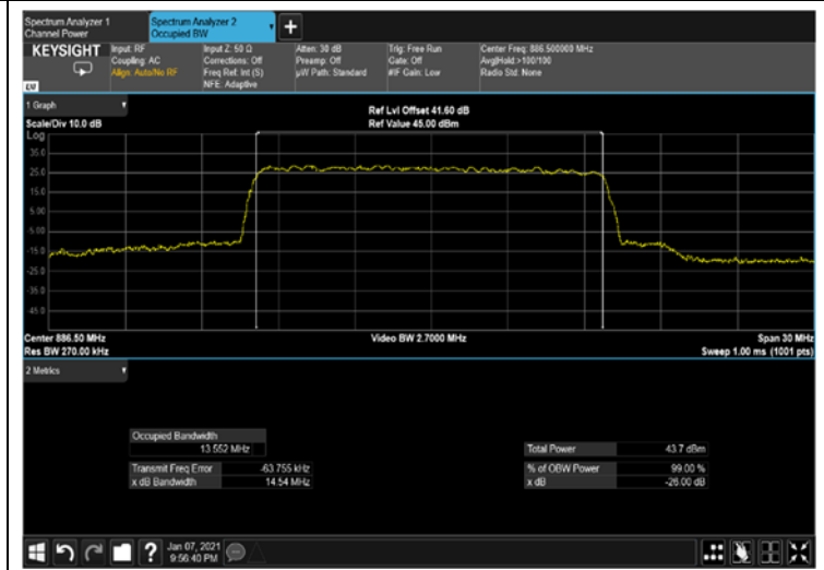
Figure 303: 256QAM 15MHz B.W.; 886.5MHz, 30kHz OUTPUT
