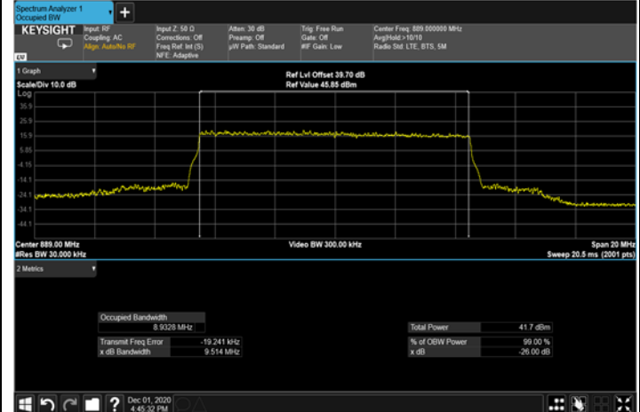
Figure 360: 16QAM 10MHz; 889.0MHz Output 4G
