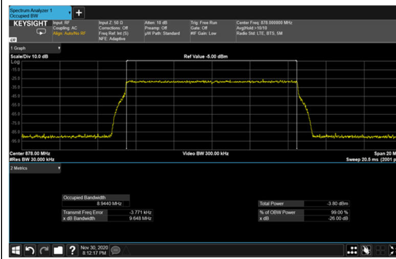
Figure 338: 64QAM 10MHz; 878.0MHz Input 4G
