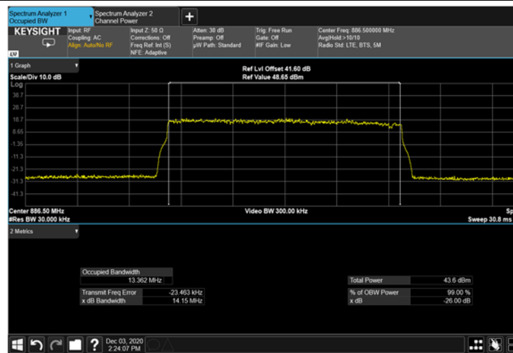
Figure 363: 16QAM 15MHz B.W.; 886.5MHz Output 4G
