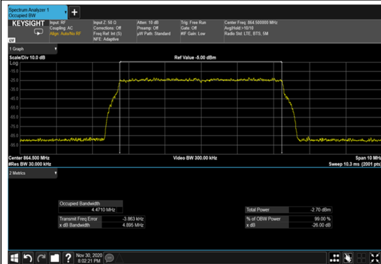
Figure 325: 16QAM 5MHz B.W.; 864.5MHz Input 4G
