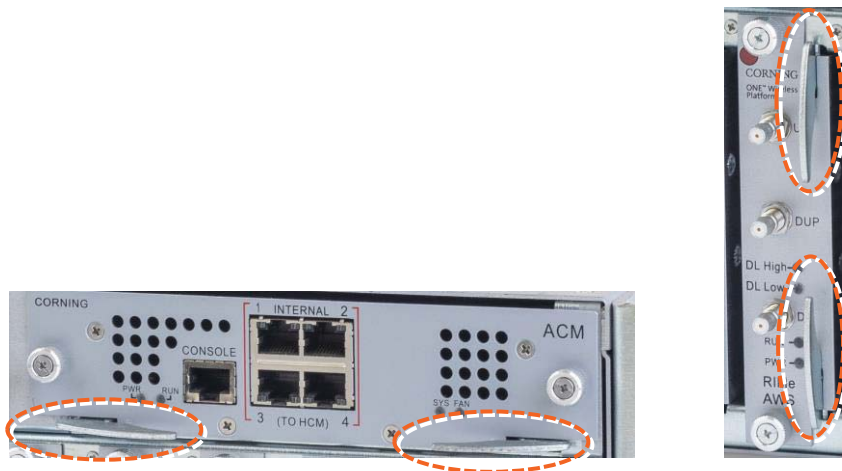
Figure 8: Module Captive Screws and Ejectors
