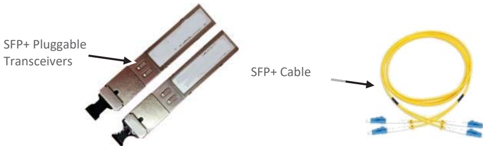
Figure 10 Remove rubber stopper from port and from SFP+ Pluggable Transceiver and insert the SFP+ Pluggable Transceivers (hot-pluggable optical transceiver module) into the port.
