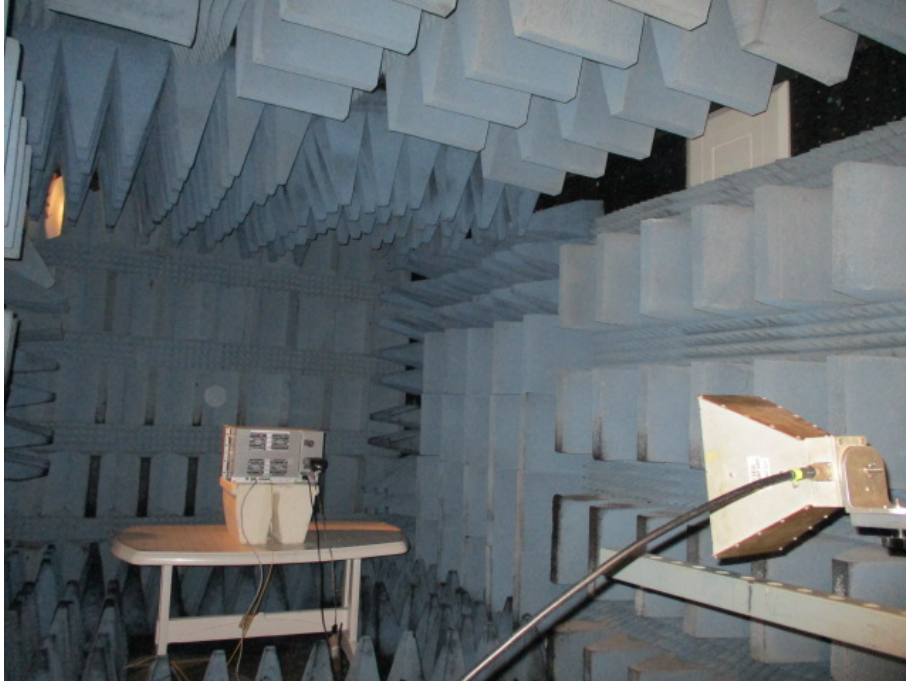
Figure 7. Radiated Emission Test 1.0 - 8.0GHz
