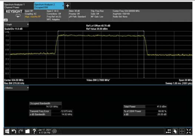
Figure 417: 256QAM 10MHz B.W; 634.5MHz, 30kHz Output
