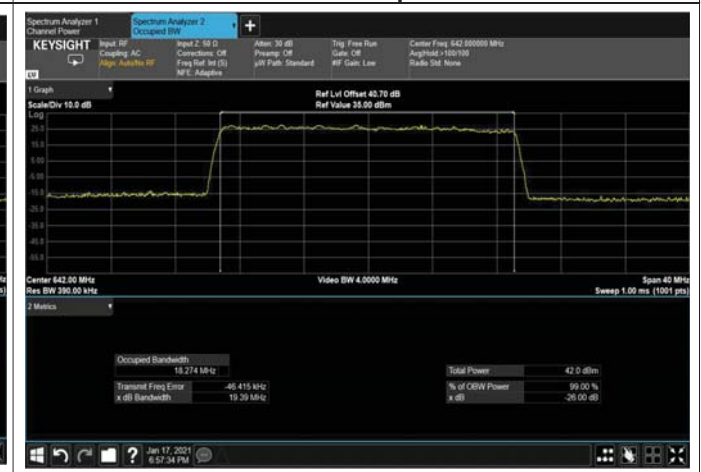
Figure 401: 64QAM 15MHz B.W; 644.5MHz, 60kHz Output
