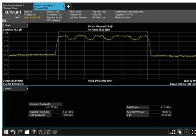
Figure 446: QPSK 15MHz B.W; 634.5MHz, 15kHz Output
