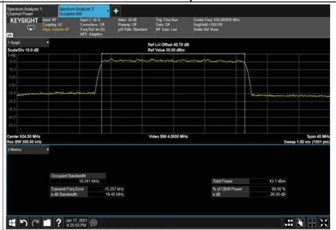
Figure 429: 256QAM 20MHz B.W; 634.5MHz, 30kHz Output
