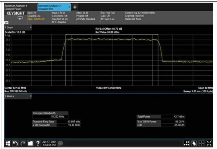
Figure 427: 256QAM 20MHz B.W; 627.0MHz, 30kHz Output
