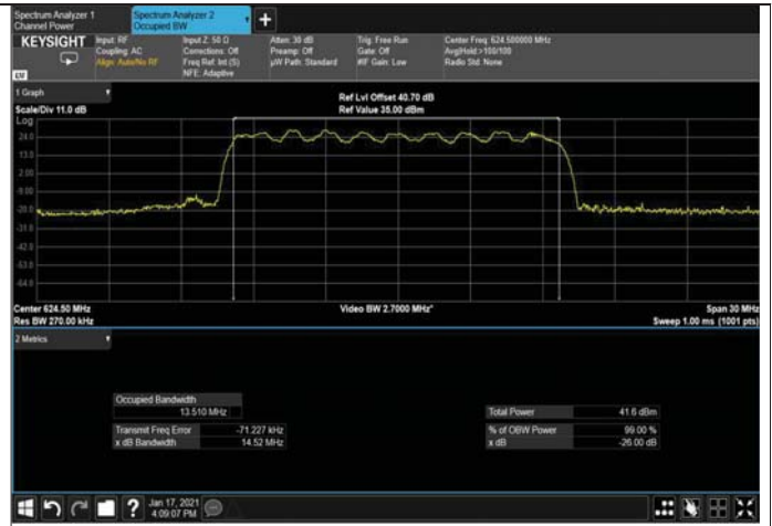
Figure 373: 16QAM 15MHz B.W; 624.5MHz, 30kHz Output
