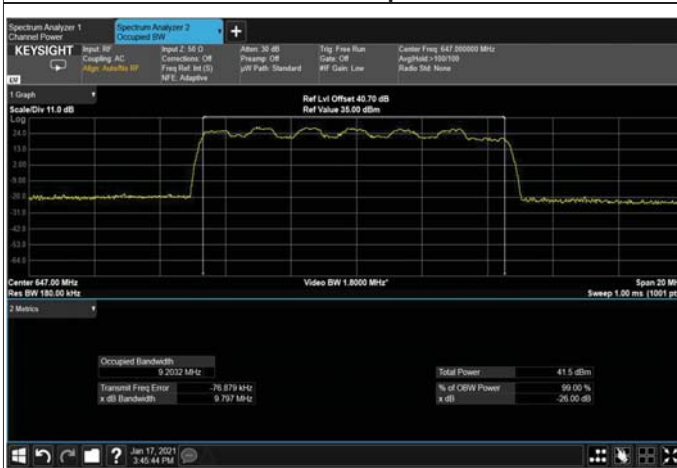
Figure 370: 16QAM 10MHz B.W; 647MHz, 15kHz Output
