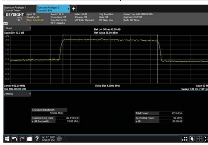
Figure 400: 64QAM 15MHz B.W; 644.5MHz, 30kHz Output
