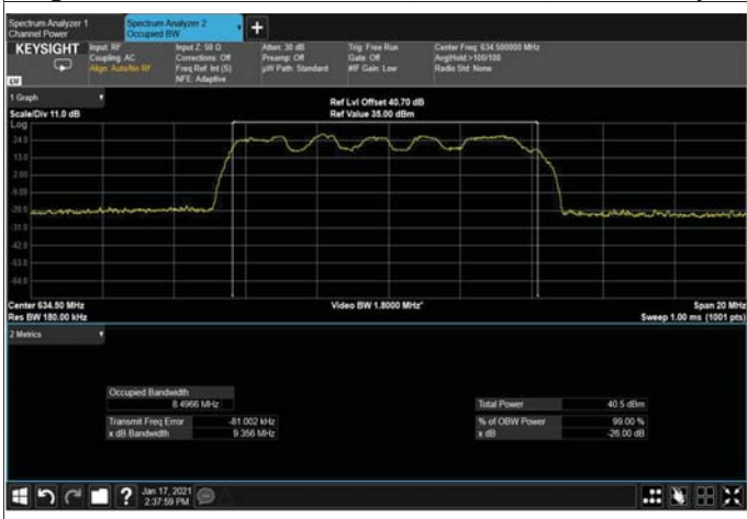
Figure 440: QPSK 10MHz B.W; 634.5MHz, 15kHz Output
