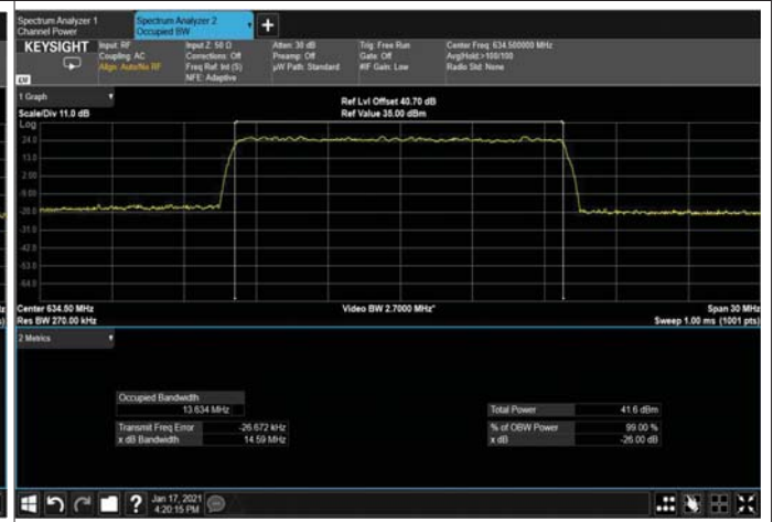
Figure 399: 64QAM 15MHz B.W; 634.5MHz, 30kHz Output
