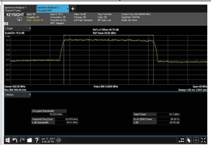
Figure 431: 256QAM 20MHz B.W; 642.0MHz, 30kHz Output
