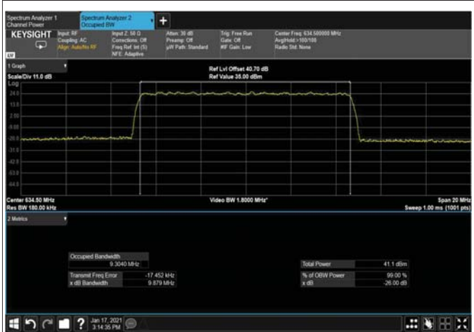
Figure 416: 256QAM 10MHz B.W; 634.5MHz, 15kHz Output
