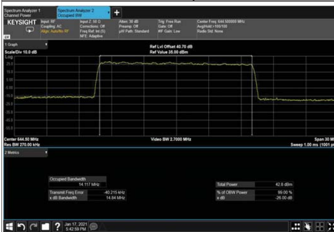
Figure 424: 256QAM 15MHz B.W; 644.5MHz, 15kHz Output
