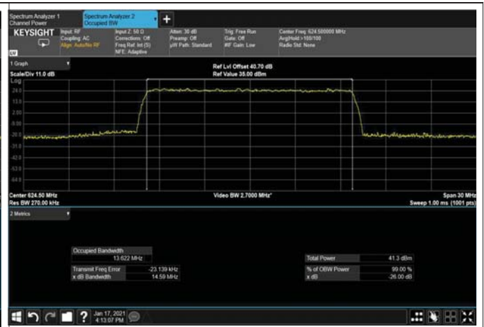
Figure 397: 64QAM 15MHz B.W; 624.5MHz, 30kHz Output
