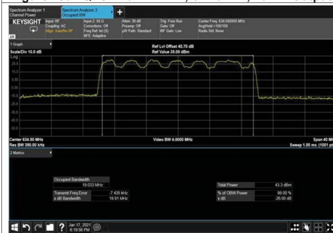
Figure 452: QPSK 20MHz B.W; 634.5MHz, 15kHz Output
