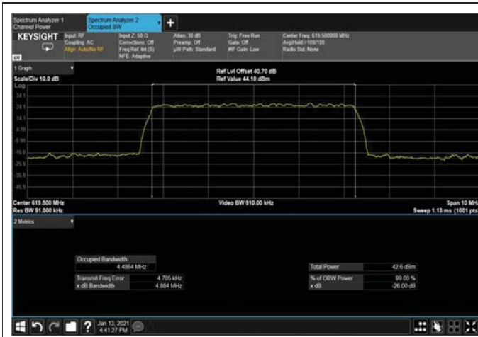
Figure 408: 256QAM 5MHz B.W; 619.5MHz, 15kHz Output
