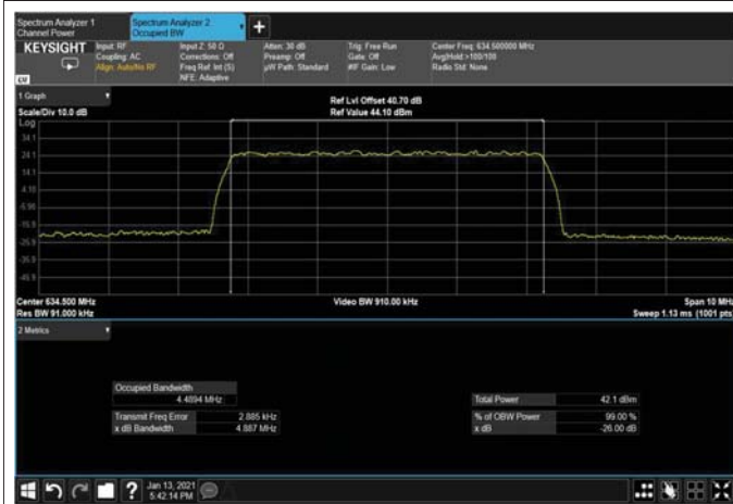
Figure 410: 256QAM 5MHz B.W; 634.5MHz, 15kHz Output
