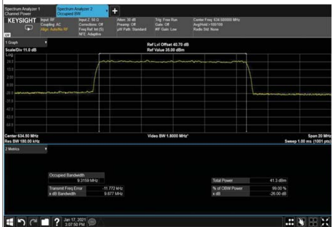
Figure 392: 64QAM 10MHz B.W; 634.5MHz, 15kHz Output
