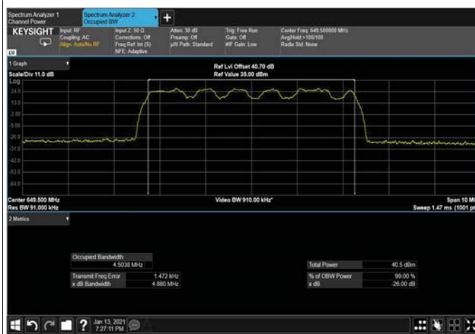
Figure 436: QPSK 5MHz B.W; 649.5MHz, 15kHz Output
