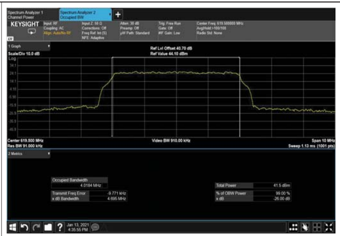
Figure 409: 256QAM 5MHz B.W; 619.5MHz, 30kHz Output
