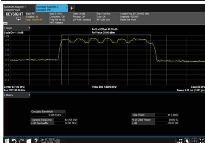
Figure 442: QPSK 10MHz B.W; 647.0MHz, 15kHz Output
