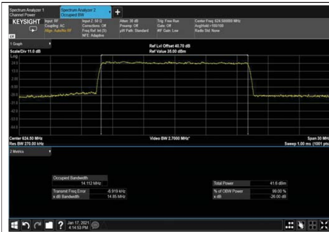
Figure 420: 256QAM 15MHz B.W; 624.5MHz, 15kHz Output
