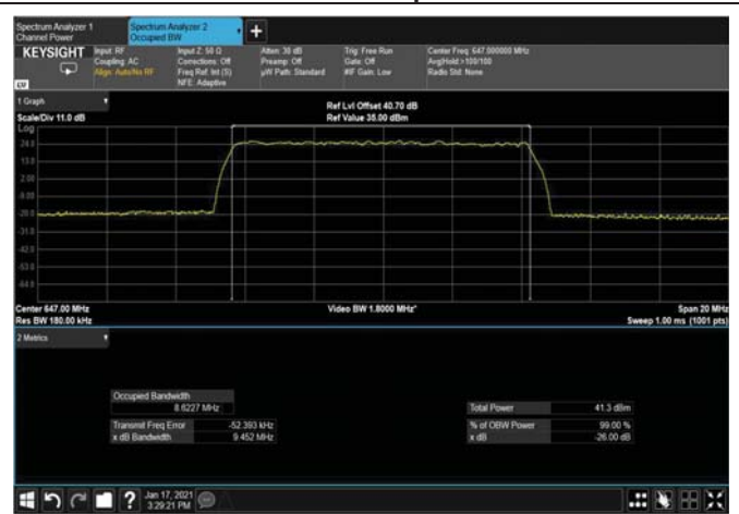
Figure 419: 256QAM 10MHz B.W; 647.0MHz, 30kHz Output
