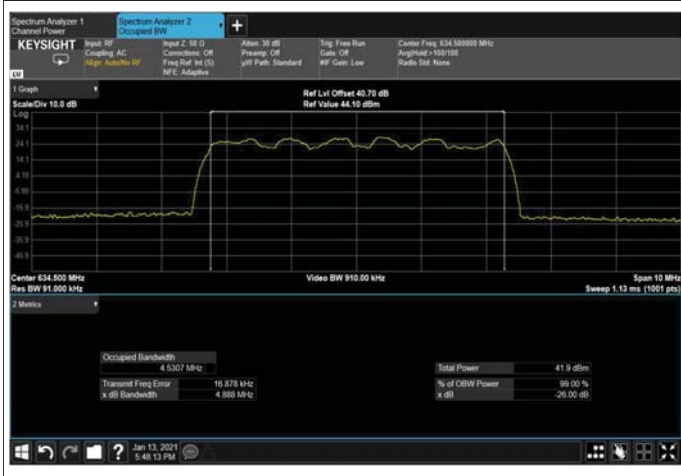
Figure 386: 64QAM 5MHz B.W; 634.5MHz, 15kHz Output
