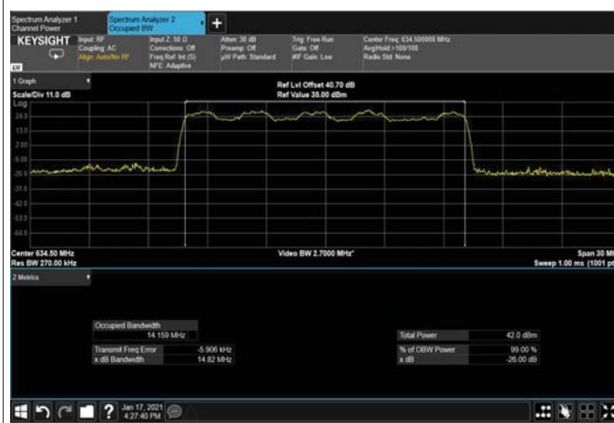
Figure 374: 16QAM 15MHz B.W; 634.5MHz, 15kHz Output
