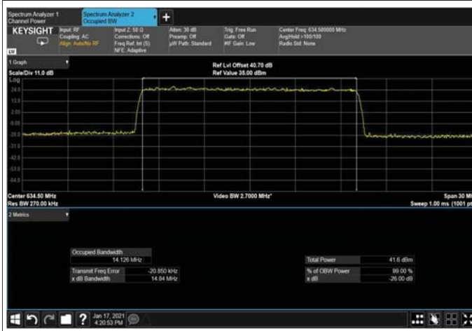
Figure 398: 64QAM 15MHz B.W; 634.5MHz, 15kHz Output
