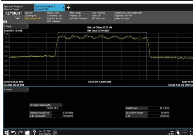
Figure 380: 16QAM 20MHz B.W; 634.5MHz, 15kHz Output
