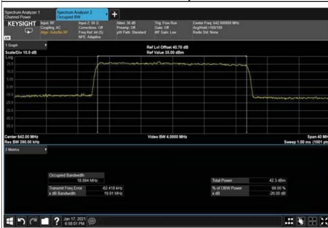
Figure 406: 64QAM 20MHz B.W; 642.5MHz, 15kHz Output
