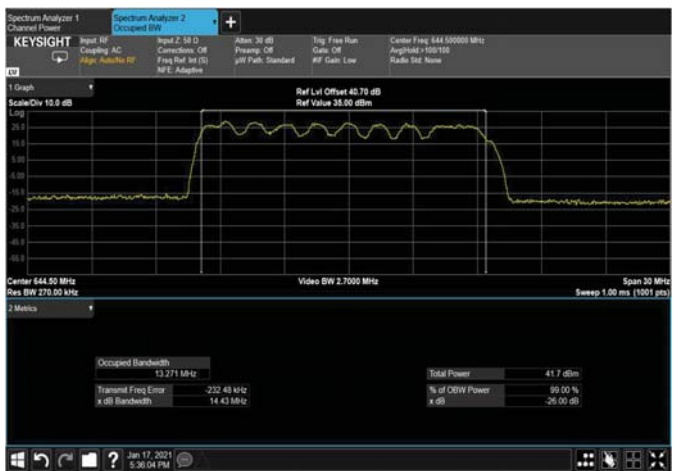
Figure 449: QPSK 15MHz B.W; 644.5MHz, 30kHz Output
