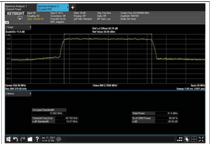
Figure 421: 256QAM 15MHz B.W; 624.5MHz, 30kHz Output
