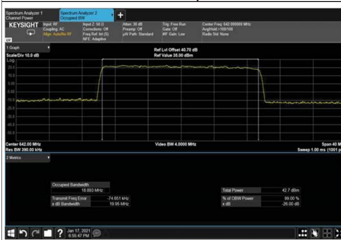
Figure 430: 256QAM 20MHz B.W; 642.0MHz, 15kHz Output
