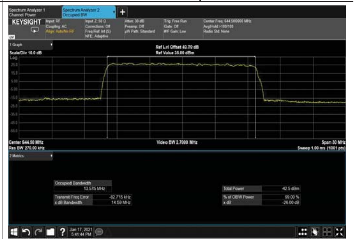
Figure 425: 256QAM 15MHz B.W; 644.5MHz, 30kHz Output
