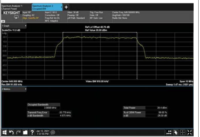
Figure 389: 64QAM 5MHz B.W; 649.5MHz, 30kHz Output
