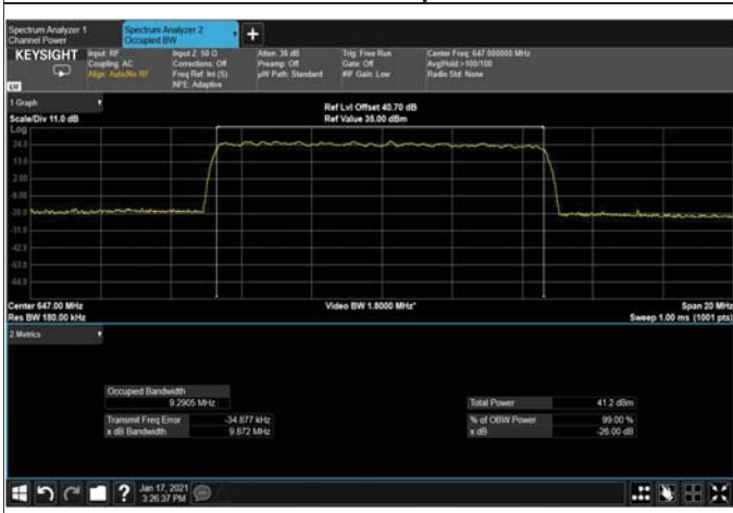
Figure 418: 256QAM 10MHz B.W; 647.0MHz, 15kHz Output
