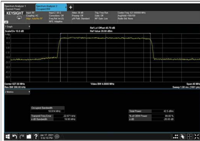
Figure 426: 256QAM 20MHz B.W; 627.0MHz, 15kHz Output
