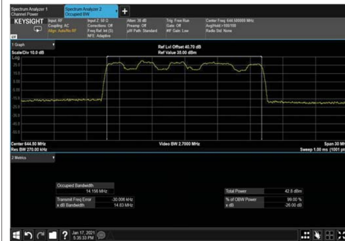
Figure 448: QPSK 15MHz B.W; 644.5MHz, 15kHz Output
