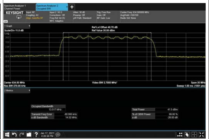
Figure 375: 16QAM 15MHz B.W; 634.5MHz, 30 kHz Output
