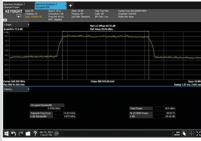
Figure 388: 64QAM 5MHz B.W; 649.5MHz, 15kHz Output
