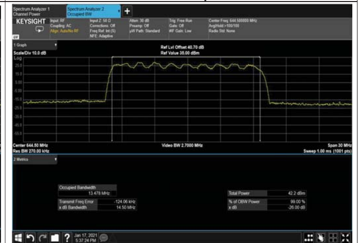
Figure 377: 16QAM 15MHz B.W; 644.5MHz, 30kHz Output
