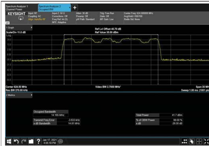
Figure 444: QPSK 15MHz B.W; 624.5MHz, 15kHz Output
