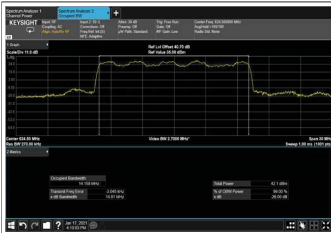
Figure 372: 16QAM 15MHz B.W; 624.5MHz, 15kHz Output
