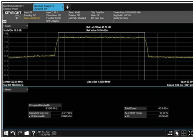
Figure 390: 64QAM 10MHz B.W; 622MHz, 15kHz Output
