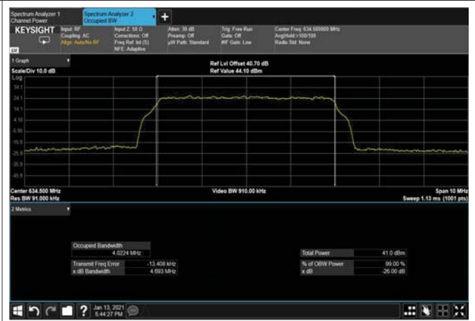
Figure 411: 256QAM 5MHz B.W; 634.5MHz, 30kHz Output
