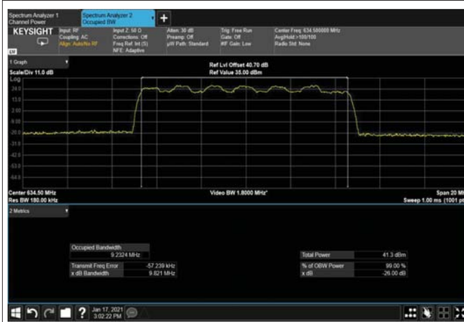
Figure 368: 16QAM 10MHz B.W; 634.5MHz, 15kHz Output
