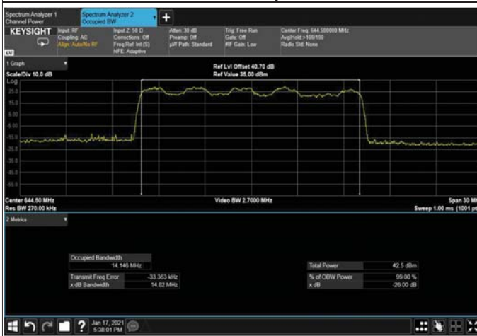
Figure 376: 16QAM 15MHz B.W; 644.5MHz, 15kHz Output
