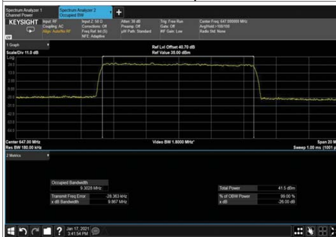
Figure 394: 64QAM 10MHz B.W; 647.0MHz, 15kHz Output
