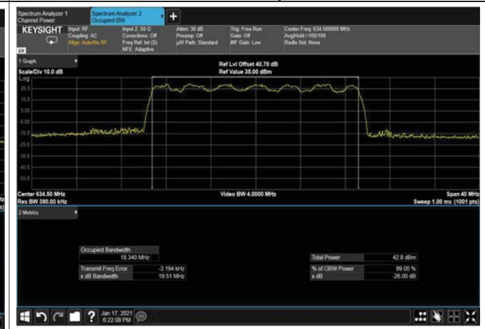
Figure 381: 16QAM 20MHz B.W; 634.5MHz, 15kHz Output
