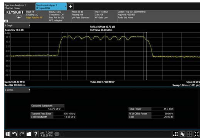
Figure 447: QPSK 15MHz B.W; 634.5MHz, 30kHz Output
