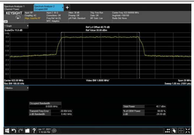
Figure 415: 256QAM 10MHz B.W; 622.0MHz, 30kHz Output
