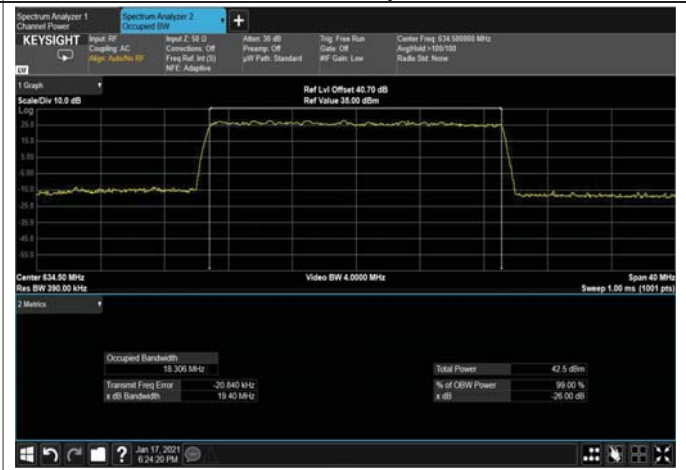
Figure 405: 64QAM 20MHz B.W; 634.5MHz, 30kHz Output
