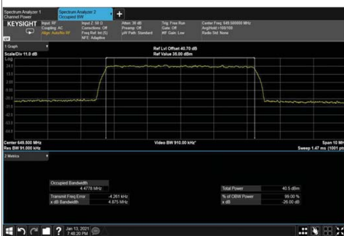
Figure 412: 256QAM 5MHz B.W; 649.5MHz, 15kHz Output
