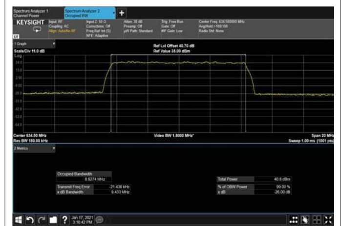
Figure 393: 64QAM 10MHz B.W; 634.5MHz, 30kHz Output
