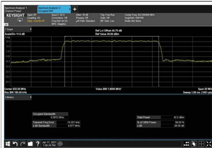
Figure 414: 256QAM 10MHz B.W; 622.0MHz, 15kHz Output
