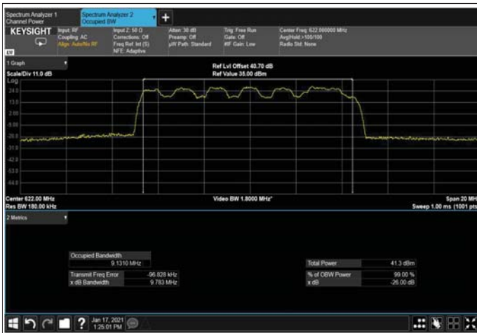
Figure 438: QPSK 10MHz B.W; 622.0MHz, 15kHz Output
