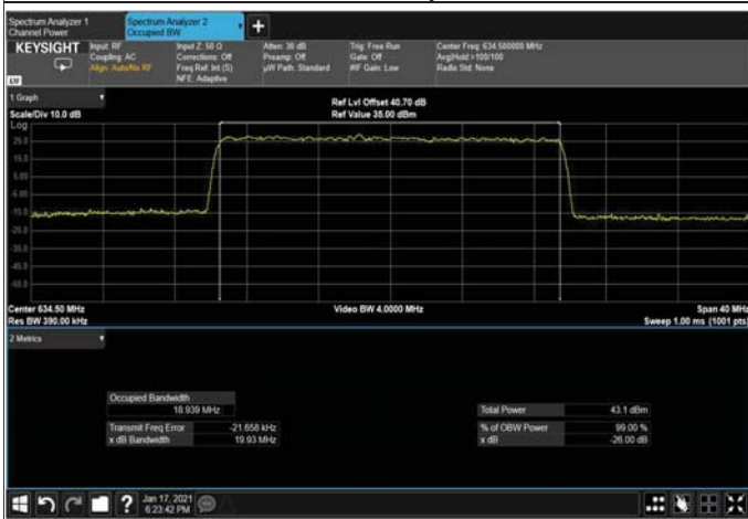
Figure 404: 64QAM 20MHz B.W; 634.5MHz, 15kHz Output
