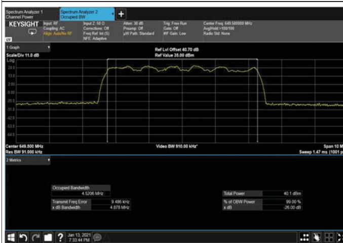
Figure 364: 16QAM 5MHz B.W; 649.5MHz, 15kHz Output
