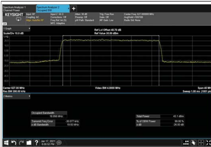
Figure 402: 64QAM 20MHz B.W; 627.0MHz, 15kHz Output
