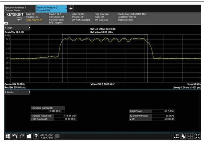
Figure 445: QPSK 15MHz B.W; 624.5MHz, 30kHz Output
