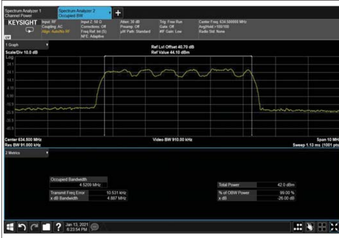
Figure 434: QPSK 5MHz B.W; 634.5MHz, 15kHz Output
