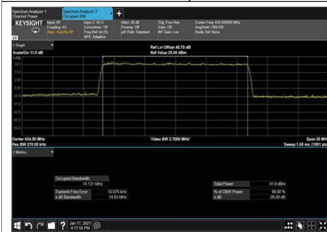
Figure 422: 256QAM 15MHz B.W; 634.5MHz, 15kHz Output
