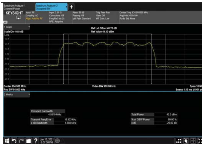
Figure 362: 16QAM 5MHz B.W; 634.5MHz, 15kHz Output
