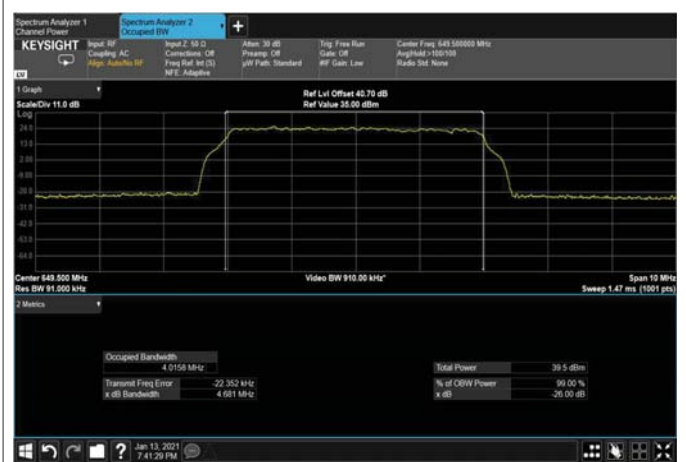
Figure 413: 256QAM 5MHz B.W; 649.5MHz, 30kHz Output
