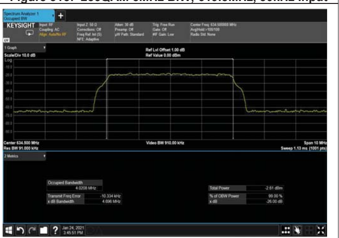
Figure 315: 256QAM 5MHz B.W; 634.5MHz, 30kHz Input
