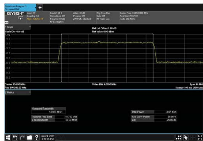
Figure 308: 64QAM 20MHz B.W; 634.5MHz, 15kHz Input
