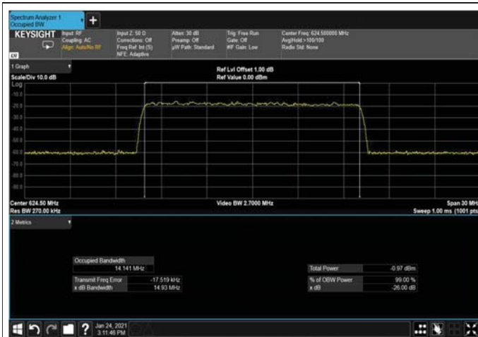
Figure 300: 64QAM 15MHz B.W; 624.5MHz, 15kHz Input
