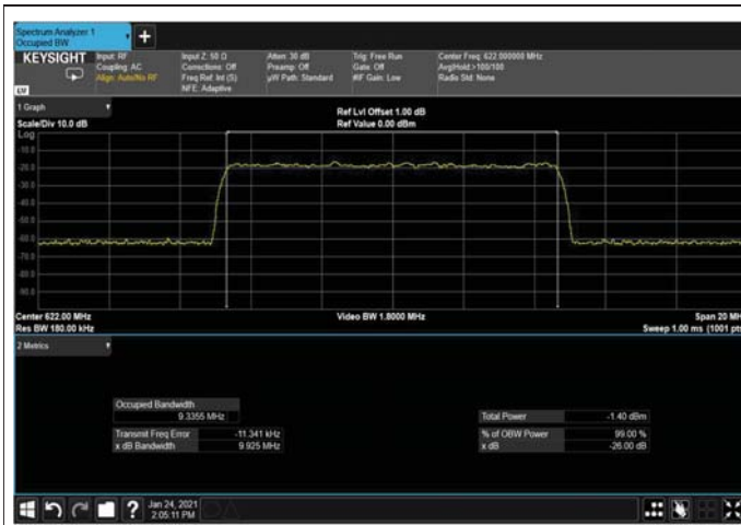
Figure 294: 64QAM 5MHz B.W; 622.0MHz, 15kHz Input
