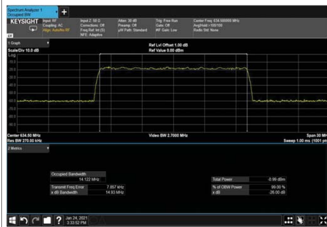
Figure 326: 256QAM 15MHz B.W; 634.5MHz, 15kHz Input
