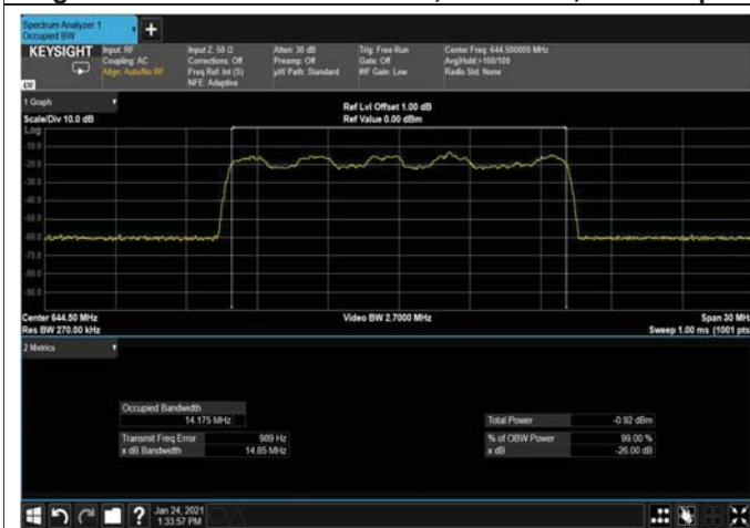
Figure 280: 16QAM 15MHz B.W; 644.5MHz, 15kHz Input
