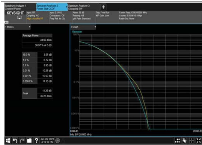
Figure 180: 16QAM 15MHz B.W; 624.5MHz, 15kHz
