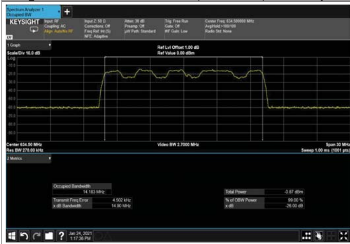
Figure 350: QPSK 15MHz B.W; 634.5MHz, 15kHz Input
