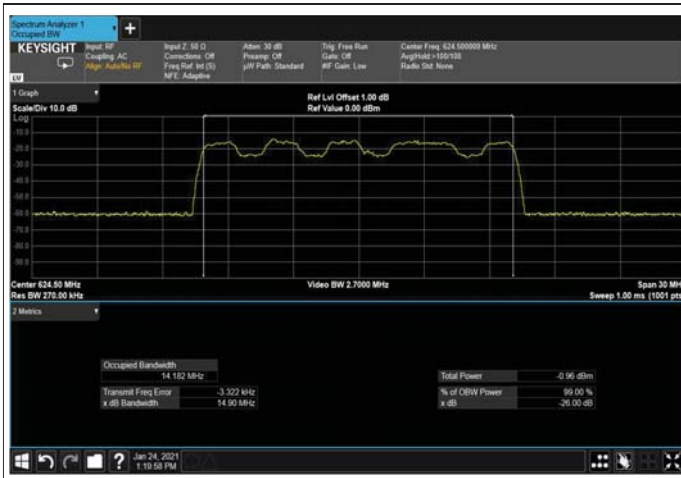
Figure 348: QPSK 15MHz B.W; 624.5MHz, 15kHz Input
