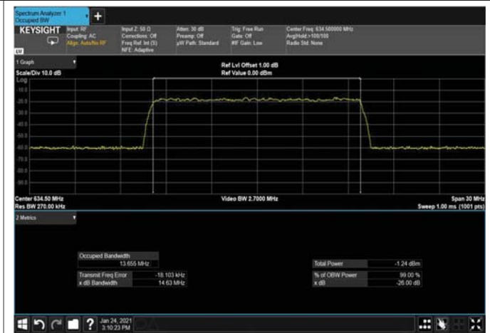
Figure 303: 64QAM 15MHz B.W; 634.5MHz, 30kHz Input
