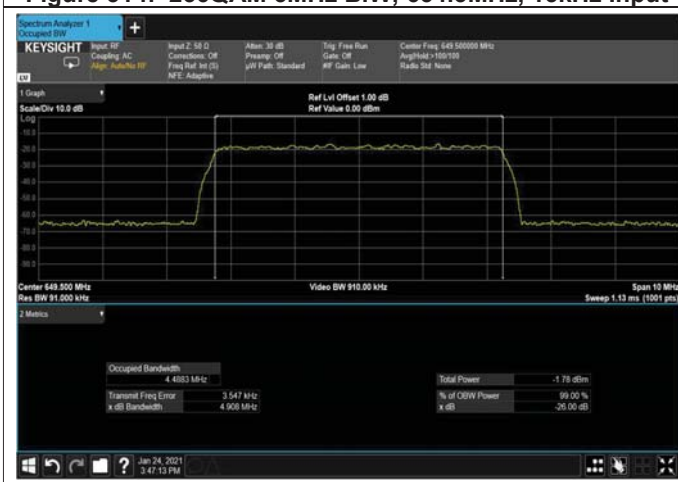
Figure 316: 256QAM 5MHz B.W; 649.5MHz, 15kHz Input
