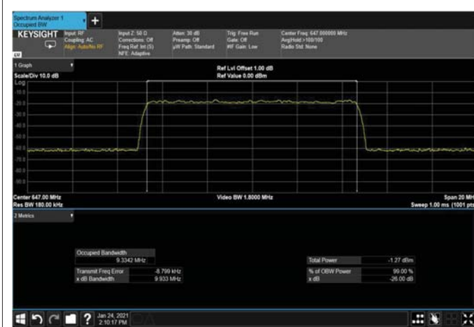
Figure 298: 64QAM 10MHz B.W; 647.0MHz, 15kHz Input
