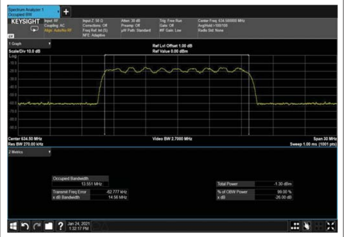
Figure 279: 16QAM 15MHz B.W; 634.5MHz, 30kHz Input
