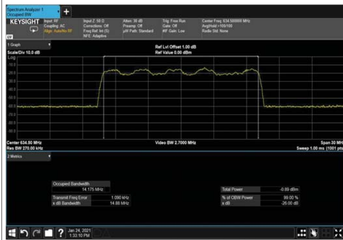
Figure 278: 16QAM 15MHz B.W; 634.5MHz, 15kHz Input
