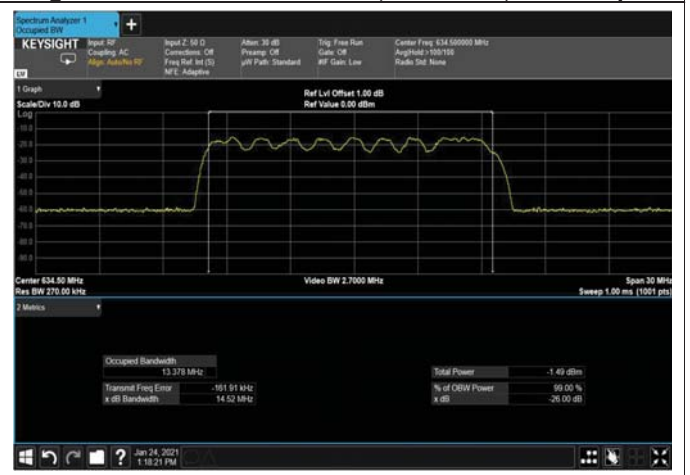
Figure 351: QPSK 15MHz B.W; 634.5MHz, 30kHz Input
