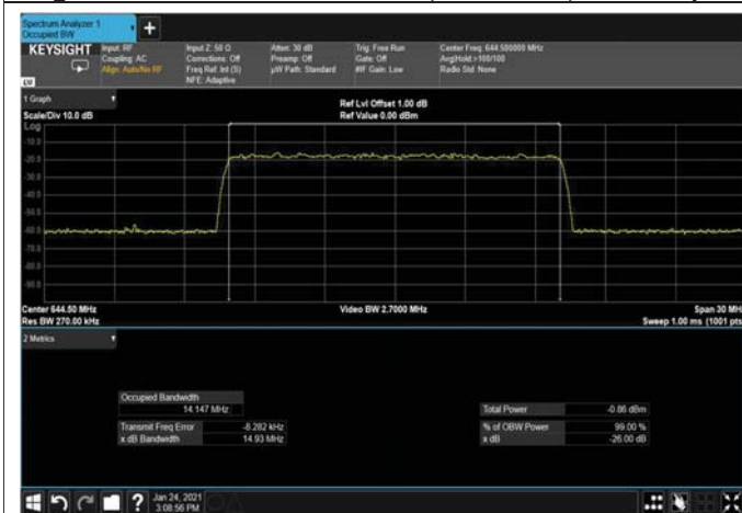
Figure 304: 64QAM 15MHz B.W; 644.5MHz, 15kHz Input
