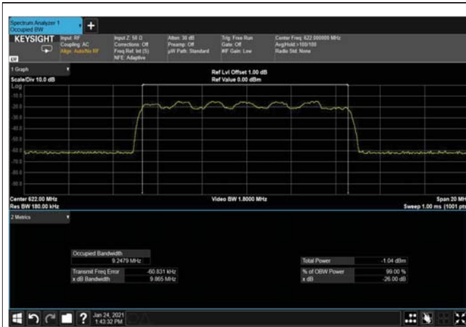
Figure 270: 16QAM 10MHz B.W; 622.0MHz, 15kHz Input
