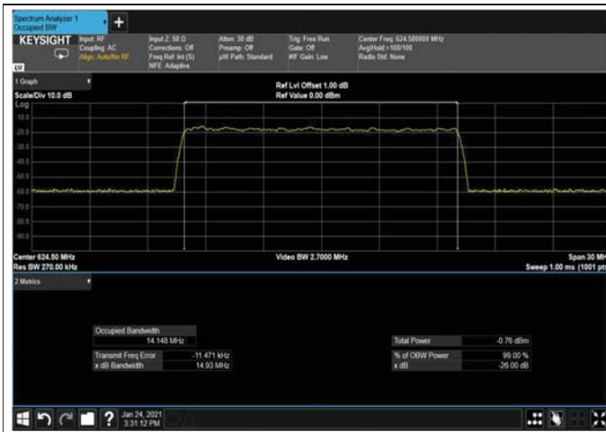
Figure 324: 256QAM 10MHz B.W; 624.5MHz, 15kHz Input
