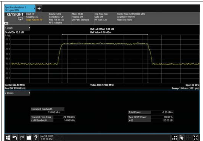
Figure 301: 64QAM 15MHz B.W; 624.5MHz, 30kHz Input
