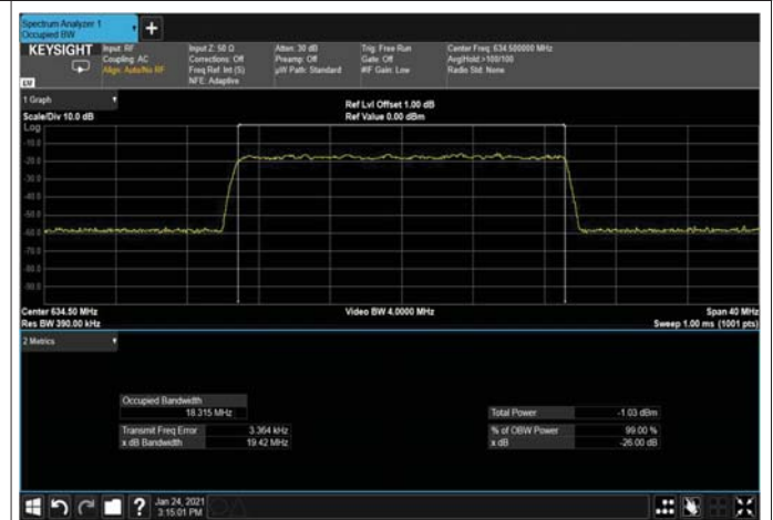
Figure 309: 64QAM 20MHz B.W; 634.5MHz, 30kHz Input
