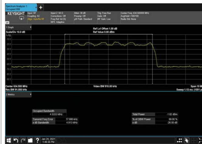
Figure 266: 16QAM 5MHz B.W; 634.5MHz, 15kHz Input
