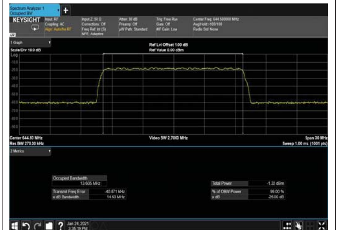
Figure 329: 256QAM 15MHz B.W; 644.5MHz, 30kHz Input
