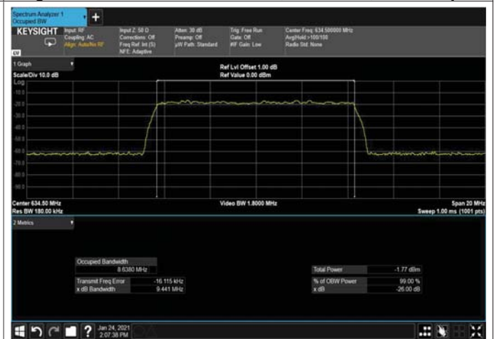
Figure 297: 64QAM 10MHz B.W; 634.5MHz, 30kHz Input
