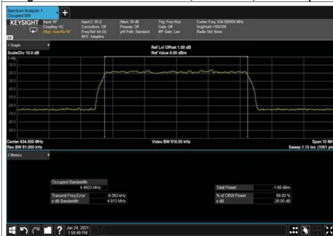
Figure 290: 64QAM 5MHz B.W; 634.5MHz, 15kHz Input
