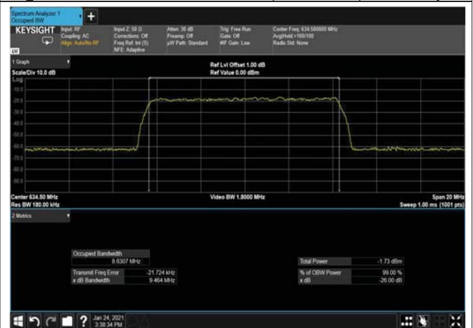
Figure 321: 256QAM 10MHz B.W; 634.5MHz, 30kHz Input
