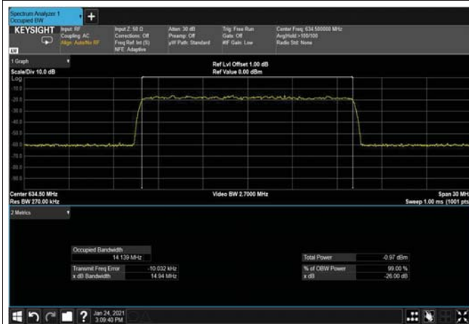
Figure 302: 64QAM 15MHz B.W; 634.5MHz, 15kHz Input
