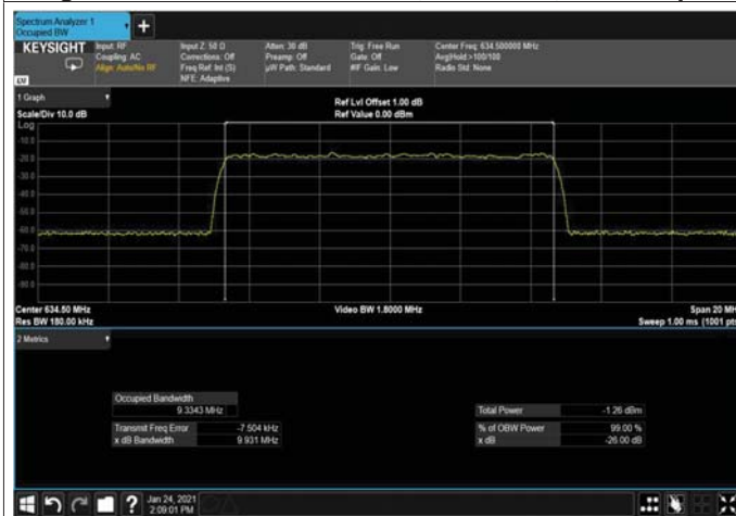
Figure 296: 64QAM 10MHz B.W; 634.5MHz, 15kHz Input
