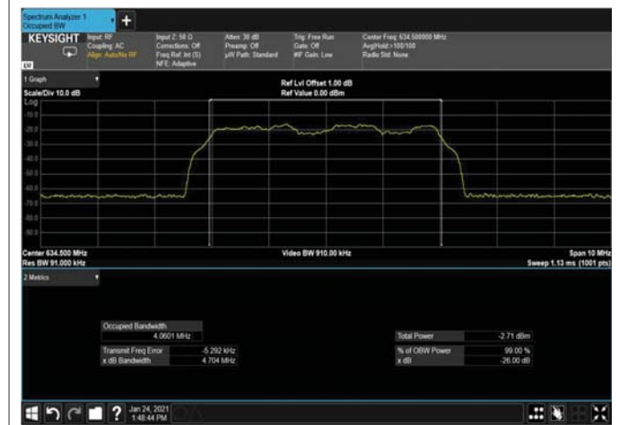
Figure 267: 16QAM 5MHz B.W; 634.5MHz, 30kHz Input
