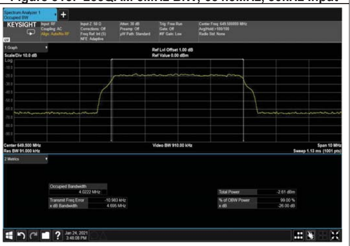
Figure 317: 256QAM 5MHz B.W; 649.5MHz, 30kHz Input
