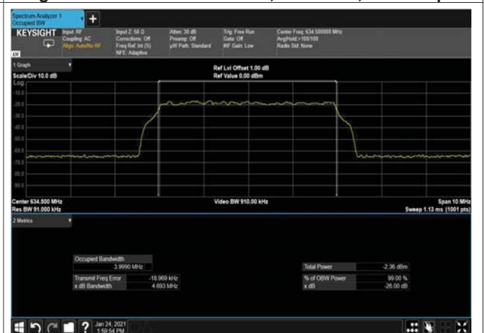
Figure 291: 64QAM 5MHz B.W; 634.5MHz, 30kHz Input
