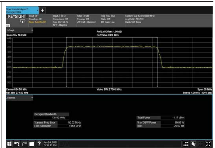
Figure 325: 256QAM 15MHz B.W; 624.5MHz, 30kHz Input
