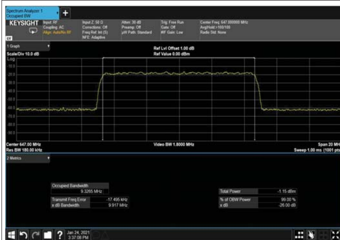
Figure 322: 256QAM 10MHz B.W; 647.0MHz, 15kHz Input
