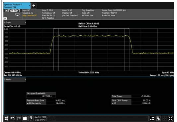
Figure 333: 256QAM 20MHz B.W; 634.5MHz, 30kHz Input
