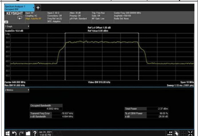
Figure 293: 64QAM 5MHz B.W; 649.5MHz, 30kHz Input
