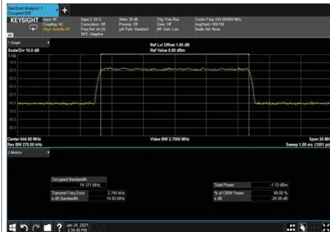
Figure 328: 256QAM 15MHz B.W; 644.5MHz, 15kHz Input
