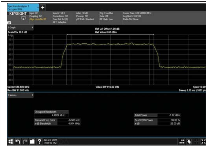
Figure 288: 16QAM 5MHz B.W; 619.5MHz, 15kHz Input
