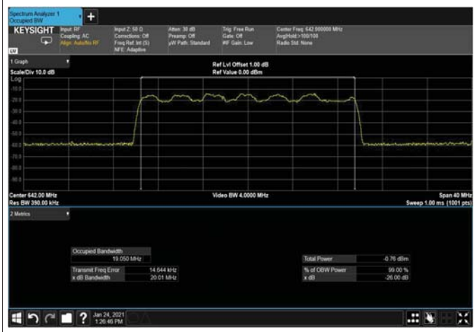
Figure 286: 16QAM 20MHz B.W; 642.0MHz, 15kHz Input
