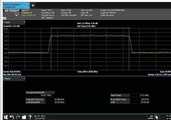
Figure 332: 256QAM 20MHz B.W; 634.5MHz, 15kHz Input
