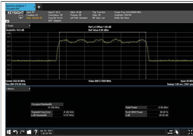
Figure 276: 16QAM 15MHz B.W; 624.5MHz, 15kHz Input
