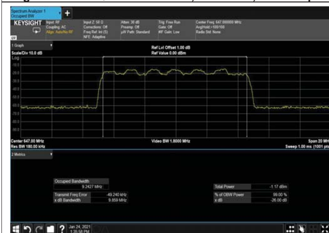
Figure 274: 16QAM 10MHz B.W; 647.0MHz, 15kHz Input
