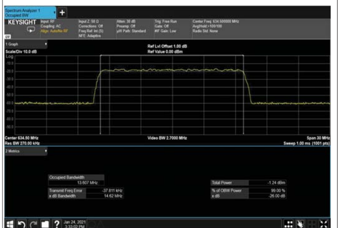
Figure 327: 256QAM 15MHz B.W; 634.5MHz, 30kHz Input
