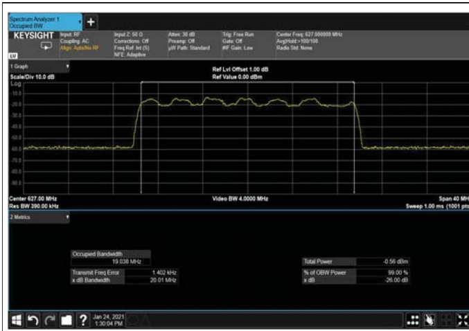
Figure 282: 16QAM 20MHz B.W; 627.0MHz, 15kHz Input
