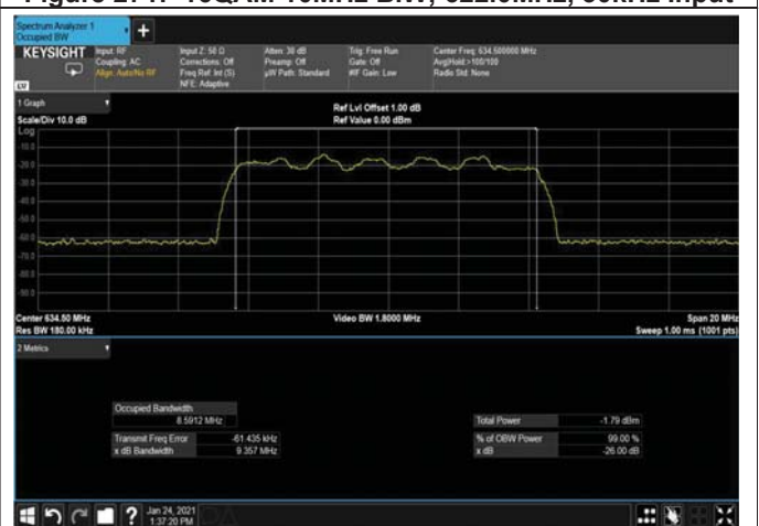
Figure 273: 16QAM 10MHz B.W; 634.5MHz, 30kHz Input
