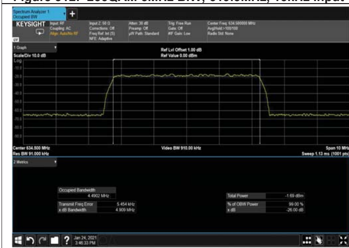
Figure 314: 256QAM 5MHz B.W; 634.5MHz, 15kHz Input
