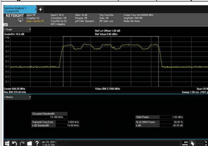
Figure 352: QPSK 15MHz B.W; 644.5MHz, 15kHz Input
