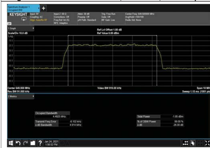
Figure 292: 64QAM 5MHz B.W; 649.5MHz, 15kHz Input
