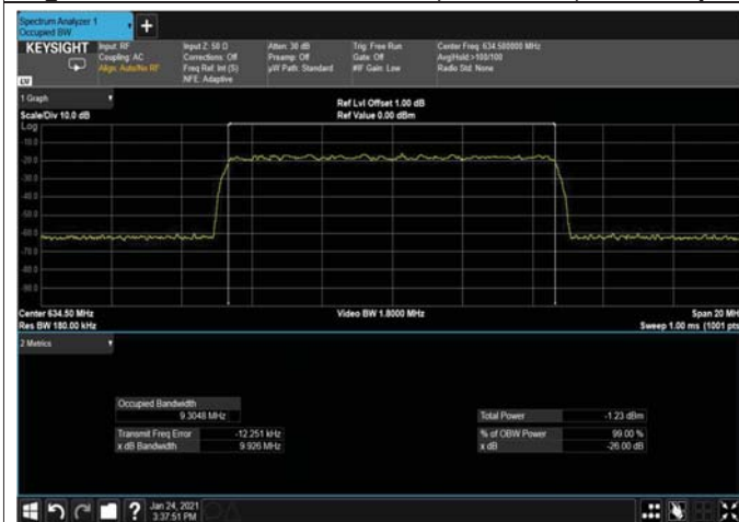
Figure 320: 256QAM 10MHz B.W; 634.5MHz, 15kHz Input
