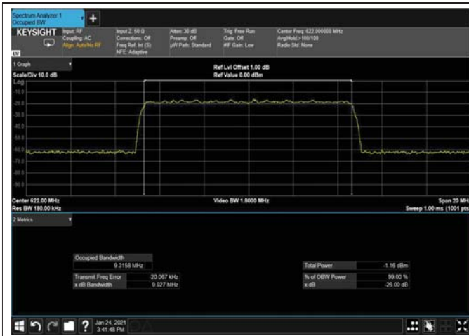
Figure 318: 256QAM 10MHz B.W; 622.0MHz, 15kHz Input
