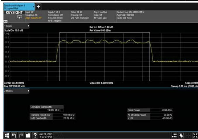
Figure 284: 16QAM 20MHz B.W; 634.5MHz, 15kHz Input
