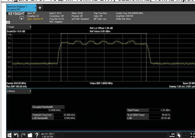
Figure 272: 16QAM 10MHz B.W; 634.5MHz, 15kHz Input
