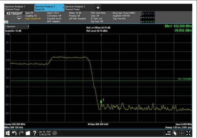
Figure 161: QPSK 15MHz B.W.; 644.5MHz, 15kHz Upper Edge
