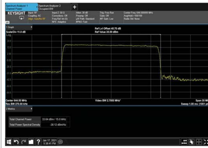
Figure 48: 64QAM 15MHz B.W; 644.5MHz, 15kHz
