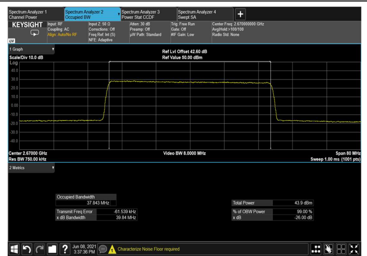
Figure 159: output 64QAM 40MHz B.W.; 2670.0MHz, 30kHz
