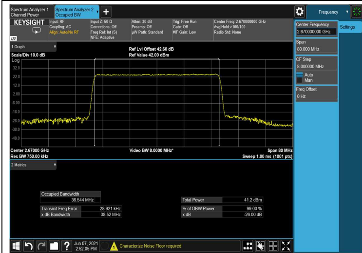
Figure 160: output 64QAM 40MHz B.W.; 2670.0MHz, 60kHz
