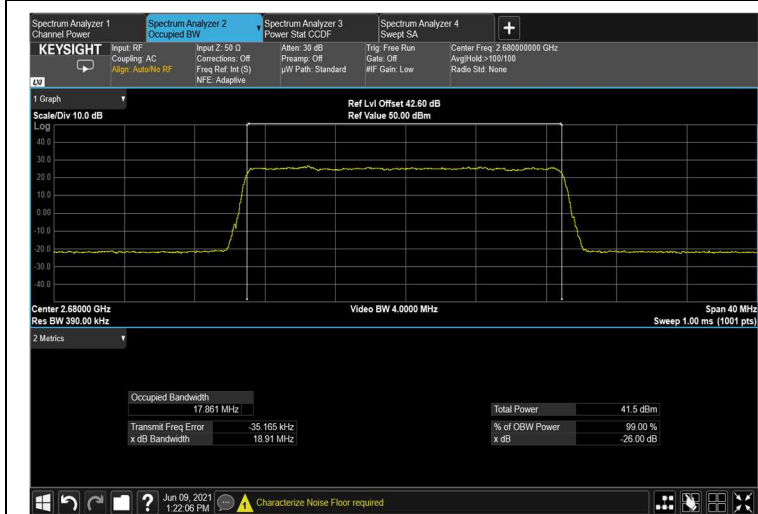
Figure 199: 16QAM 20MHz B.W.; 2680.0MHz OUTPUT
