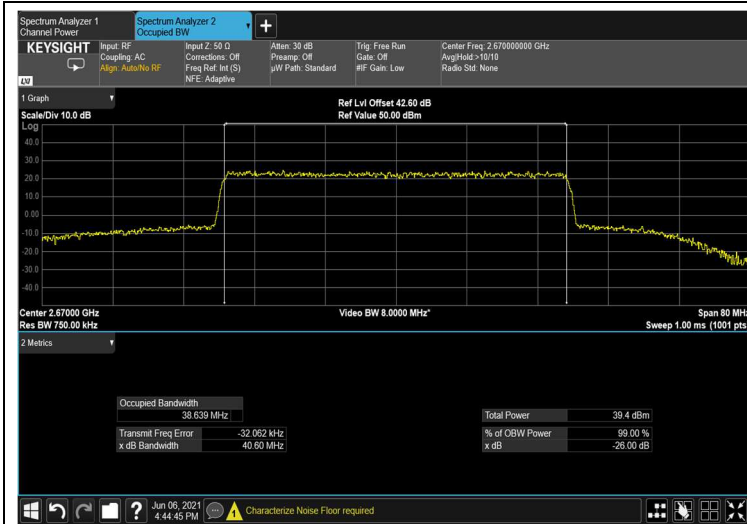
Figure 188: output QPSK 40MHz B.W.; 2670.0MHz, 15kHz
