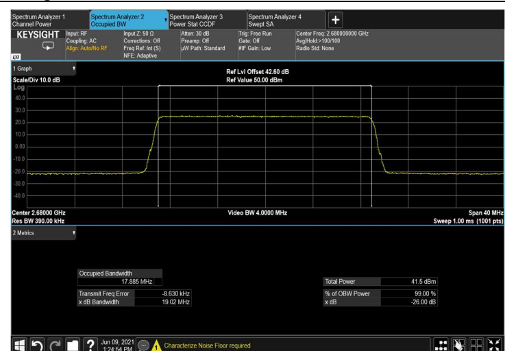
Figure 202: 64QAM 20MHz B.W.; 2680.0MHz OUTPUT
