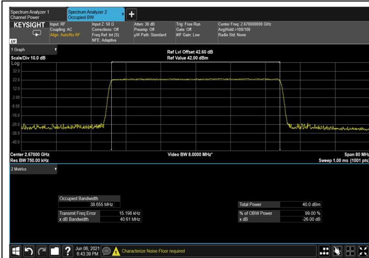
Figure 158: output 64QAM 40MHz B.W.; 2670.0MHz, 15kHz
