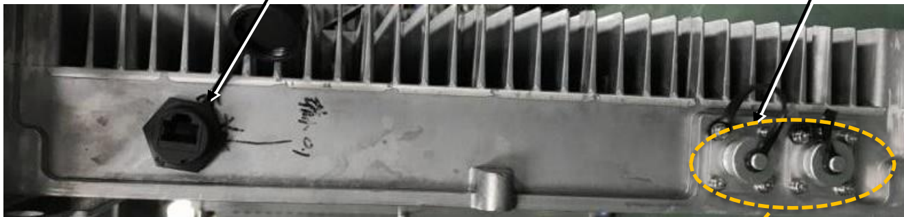
DRY CONTACT (8 pin) and external alarm interface (6pin)
