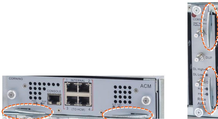
Figure 8: Module Captive Screws and Ejectors
