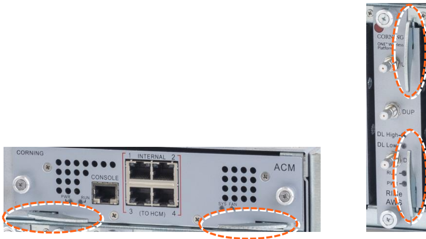
Figure 5: Module Captive Screws and Ejectors
