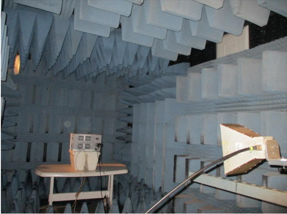
**Radiated Emission Test 1.0 - 9.0GHz**
