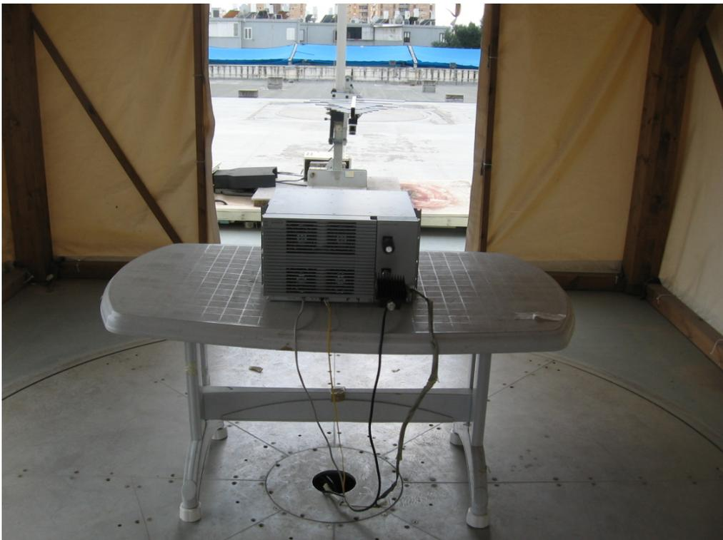
**Radiated Emission Test 200 - 1000MHz**
