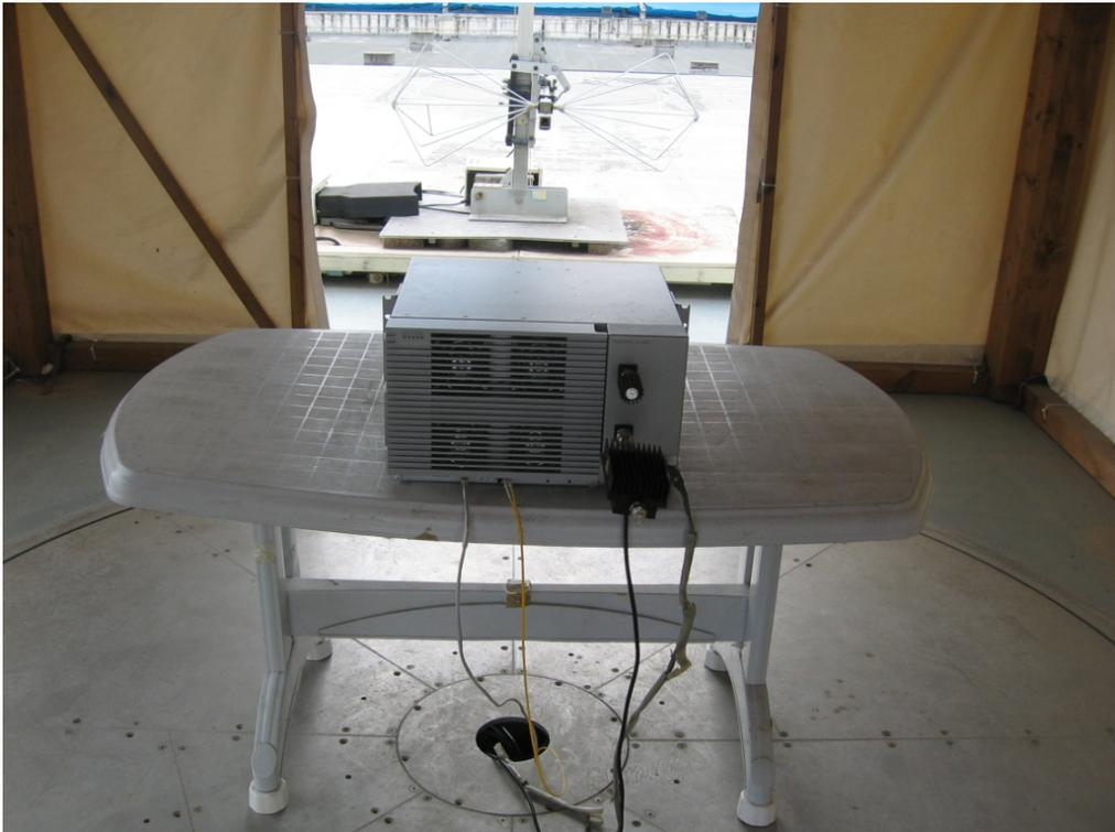
**Radiated Emission Test 30 - 200 MHz**
