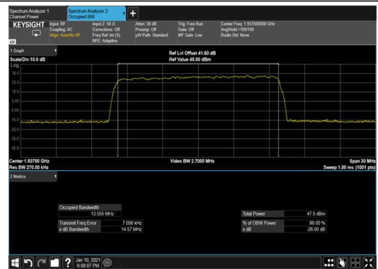
Figure 300: 256QAM 15MHz B.W.; 1937.5MHz, 30kHz Output
