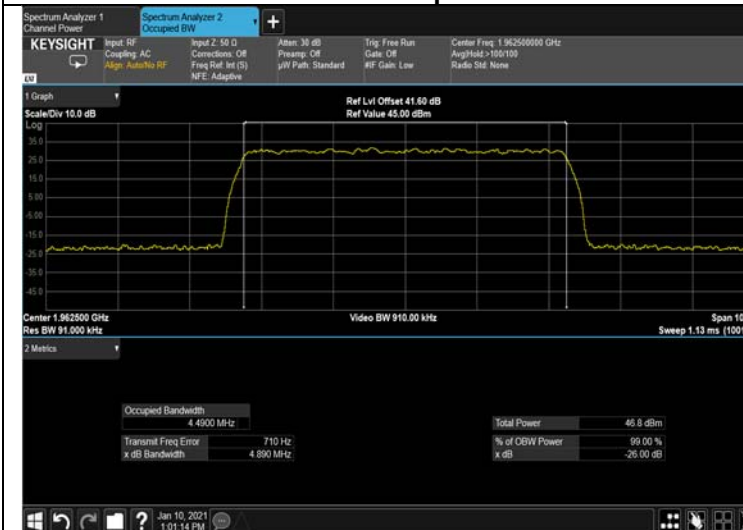
Figure 289: 256QAM 5MHz B.W.; 1962.5MHz, 15kHz Output
