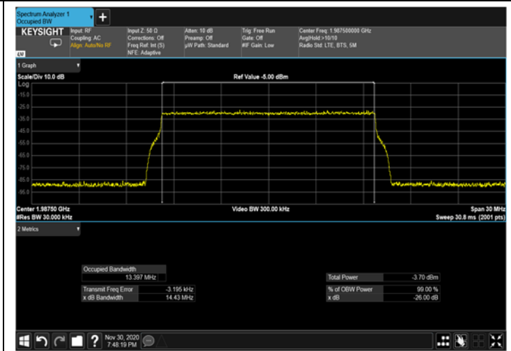
Figure 343: 64QAM 15MHz B.W.; 1987.5MHz Input – 4G
