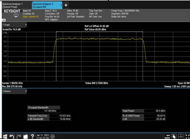
Figure 283: 64QAM 15MHz B.W.; 1962.5MHz, 15kHz Output
