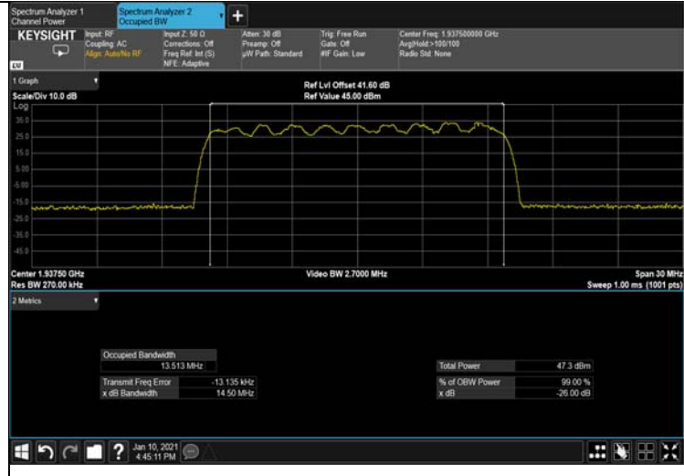
Figure 264: 16QAM 15MHz B.W.; 1937.5MHz, 30kHz Output
