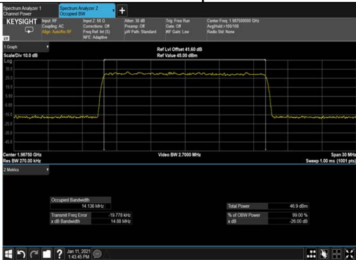
Figure 285: 64QAM 15MHz B.W.; 1987.5MHz, 15kHz Output
