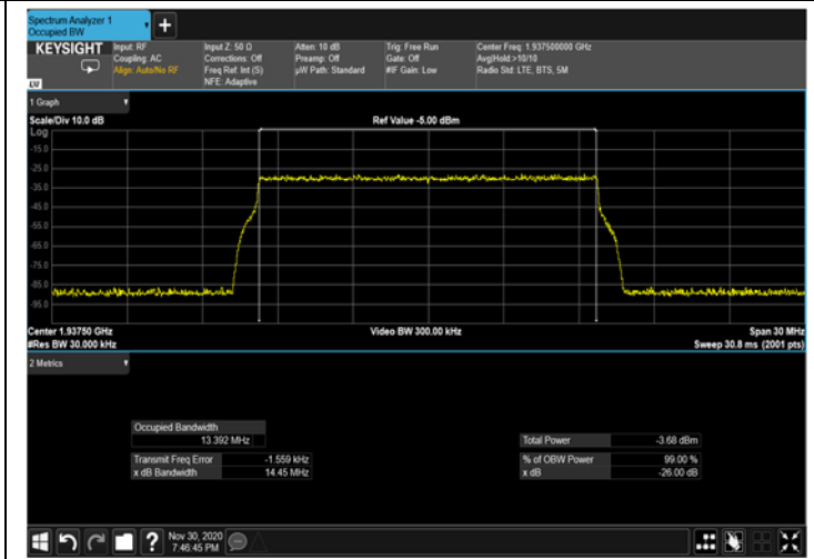
Figure 341: 64QAM 15MHz B.W.; 1937.5MHz Input – 4G
