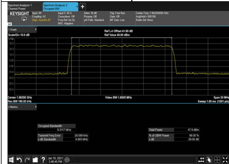
Figure 295: 256QAM 10MHz B.W.; 1962.5MHz, 15kHz Output
