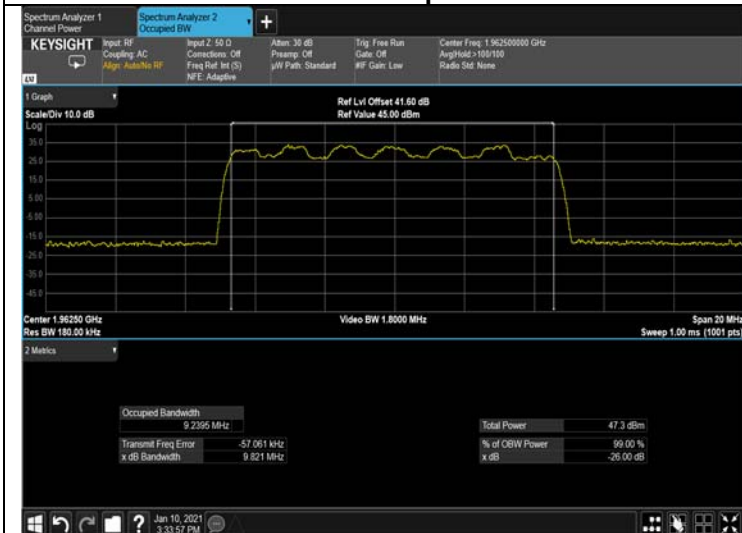
Figure 259: 16QAM 10MHz B.W.; 1962.5MHz, 15kHz Output
