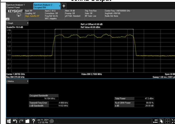
Figure 267: 16QAM 15MHz B.W.; 1990.0MHz, 15kHz Output
