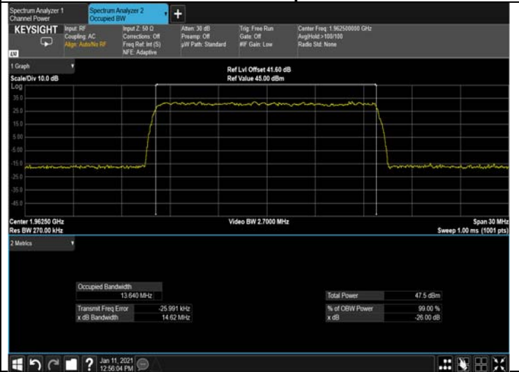
Figure 284: 64QAM 15MHz B.W.; 1962.5MHz, 30kHz Output
