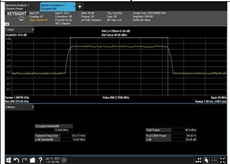
Figure 286: 64QAM 15MHz B.W.; 1987.5MHz, 30kHz Output
