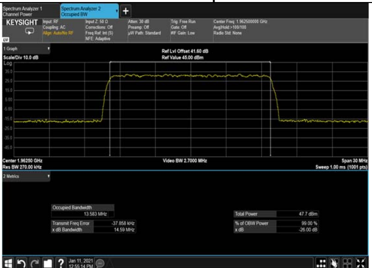
Figure 302: 256QAM 15MHz B.W.; 1962.5MHz, 30kHz Output
