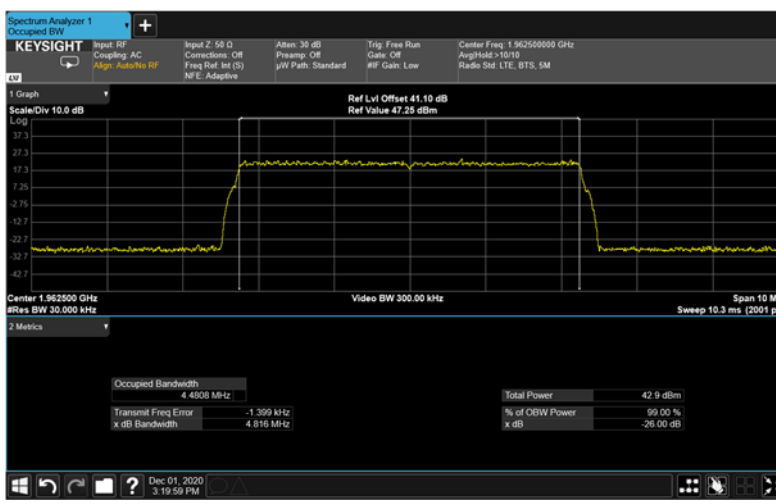
Figure 366: 64QAM 5MHz B.W.; 1962.5MHz Output – 4G
