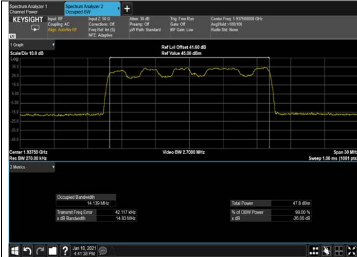
Figure 317: QPSK 15MHz B.W.; 1937.5MHz, 15kHz Output
