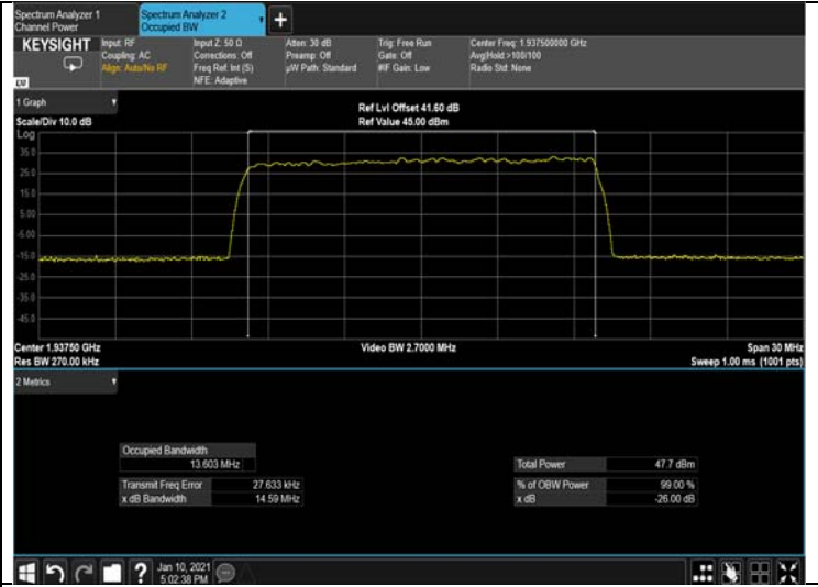
Figure 282: 64QAM 15MHz B.W.; 1937.5MHz, 30kHz Output
