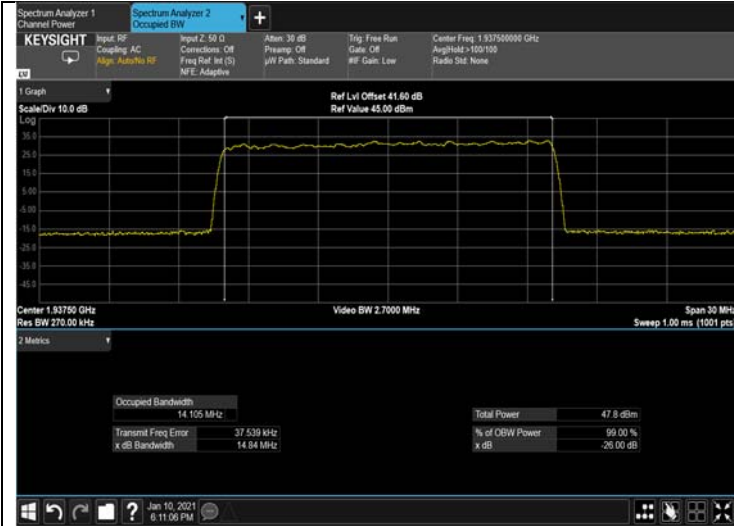
Figure 299: 256QAM 15MHz B.W.; 1937.5MHz, 15kHz Output
