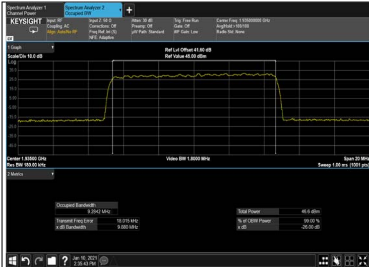
Figure 293: 256QAM 10MHz B.W.; 1935.0MHz, 15kHz Output
