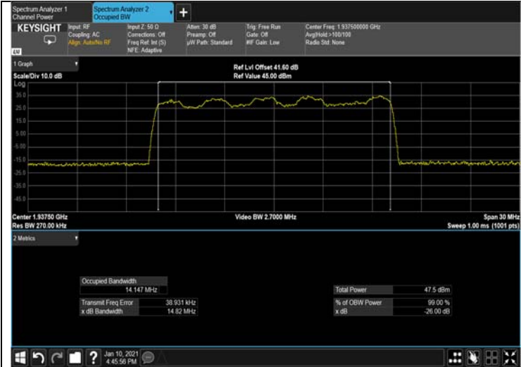
Figure 263: 16QAM 15MHz B.W.; 1937.5MHz, 15kHz Output
