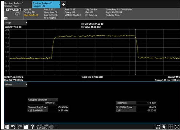
Figure 281: 64QAM 15MHz B.W.; 1937.5MHz, 15kHz Output
