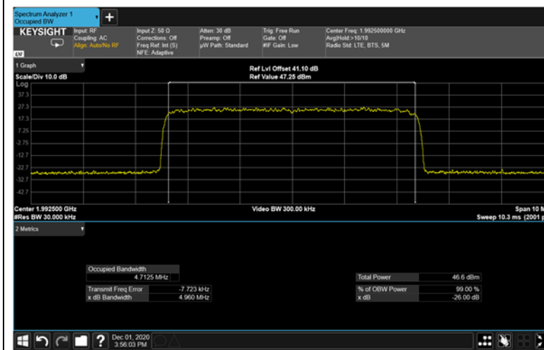
Figure 358: 16QAM 5MHz B.W.; 1992.5MHz Output – 4G
