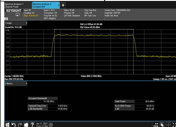
Figure 301: 256QAM 15MHz B.W.; 1962.5MHz, 15kHz Output
