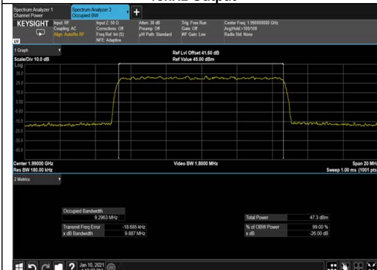
Figure 297: 256QAM 10MHz B.W.; 1990.0MHz, 15kHz Output
