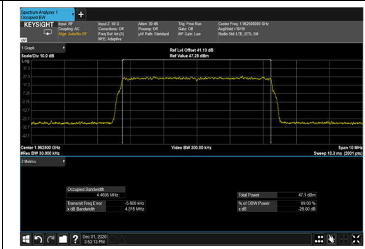
Figure 357: 16QAM 5MHz B.W.; 1962.5MHz Output – 4G
