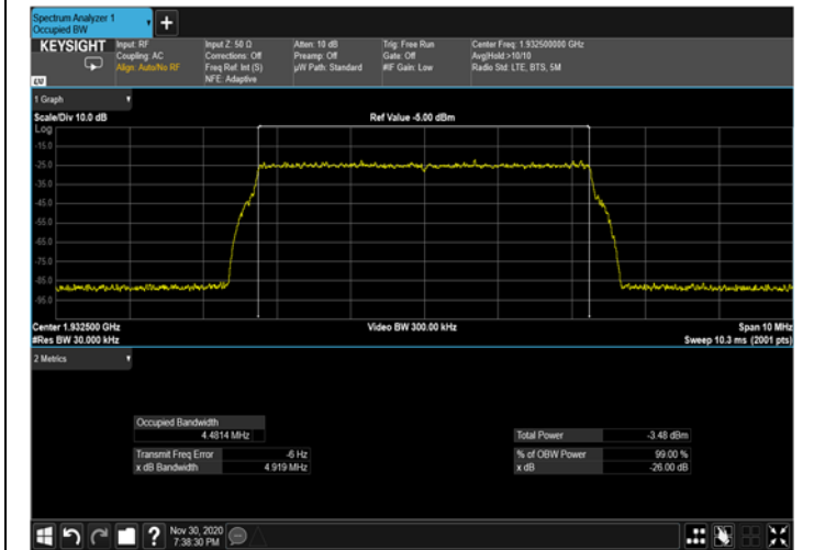
Figure 335: 64QAM 5MHz B.W.; 1932.5MHz Input – 4G
