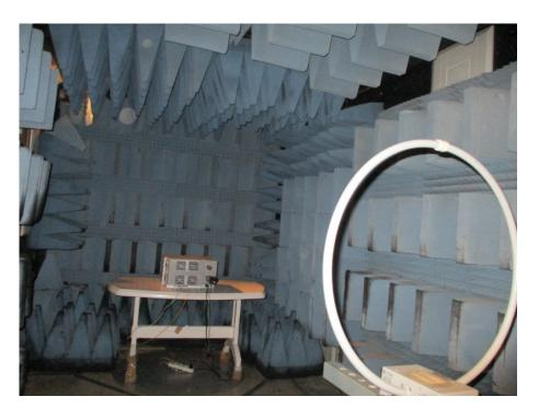
Radiated Emission Test 9kHz - 30MHz
