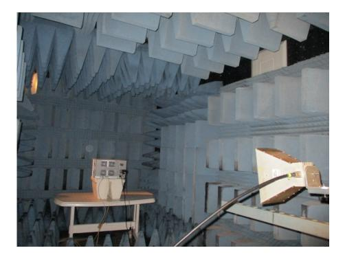
Radiated Emission Test 1.0 - 9.0GHz
