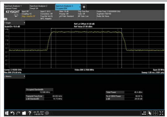
Figure 302: 256QAM 15MHz B.W; 2192.5MHz, 30kHz OUTPUT
