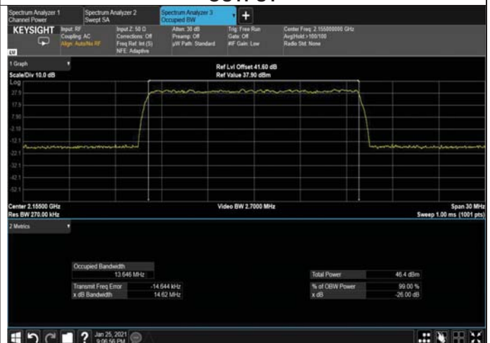
Figure 282: 64QAM 15MHz B.W; 2155.0MHz, 30kHz OUTPUT
