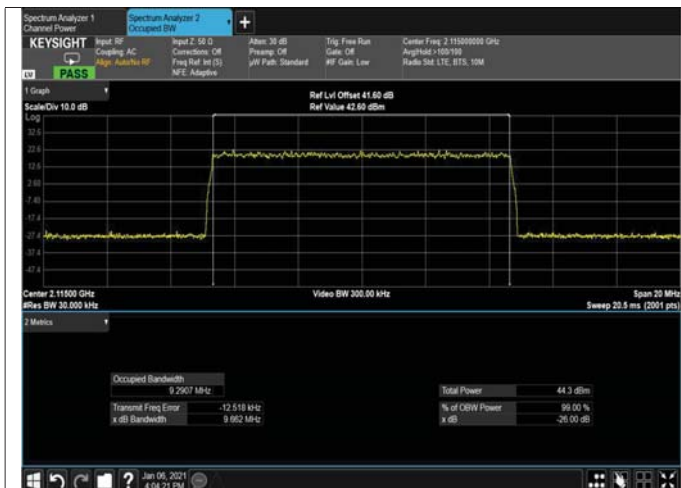
Figure 273: 64QAM 10MHz B.W; 2115.0MHz, 15kHz OUTPUT
