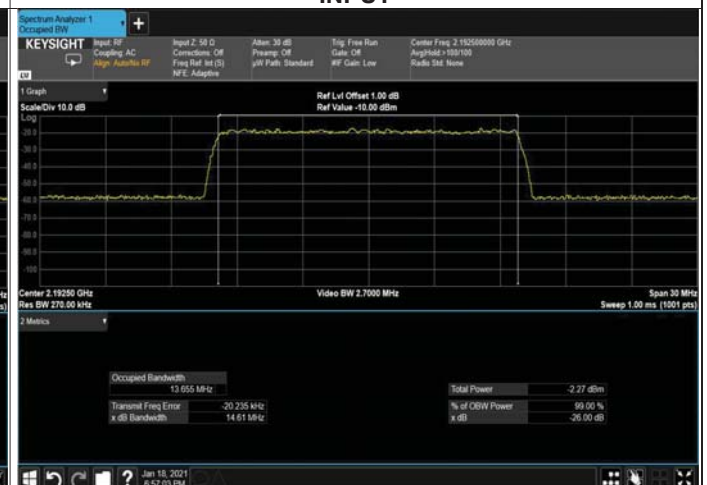
Figure 212: 64QAM 15MHz B.W; 2192.5MHz, 30kHz INPUT
