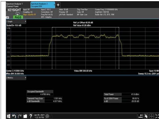
Figure 249: 16QAM 5MHz B.W; 2112.5MHz, 15kHz OUTPUT
