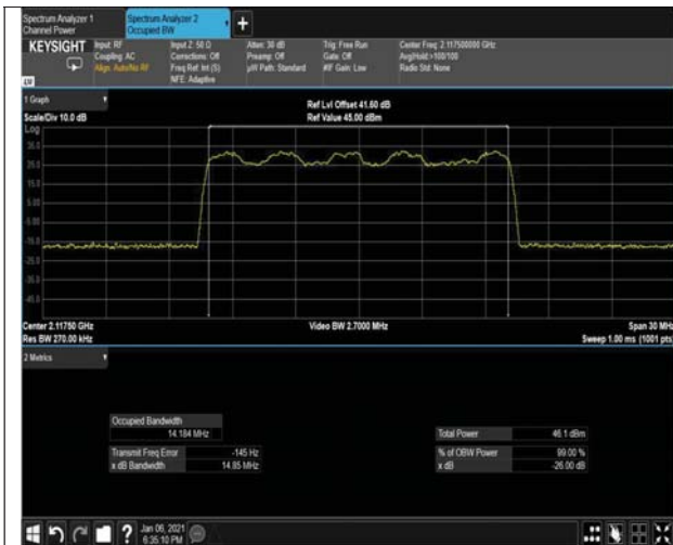
Figure 261: 16QAM 15MHz B.W; 2117.5MHz, 15kHz OUTPUT
