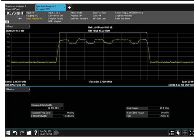
Figure 315: QPSK 15MHz B.W; 2117.5MHz, 15kHz OUTPUT
