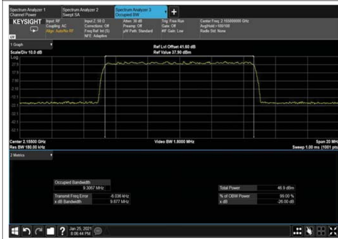
Figure 293: 256QAM 10MHz B.W; 2155MHz, 15kHz OUTPUT
