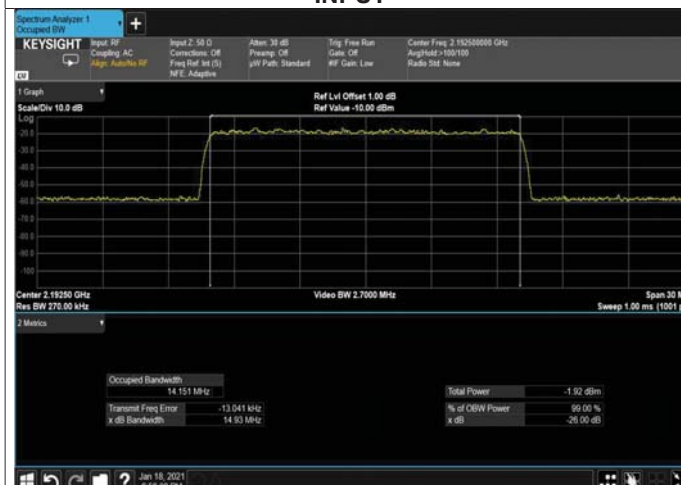
Figure 211: 64QAM 15MHz B.W; 2192.5MHz, 15kHz INPUT
