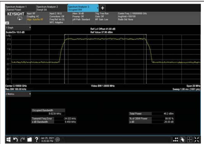
Figure 296: 256QAM 10MHz B.W; 2195MHz, 30kHz OUTPUT
