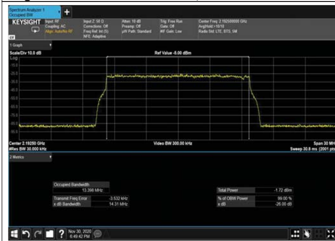
Figure 332: 16QAM 15MHz B.W; 2192.5MHz – 4G INPUT
