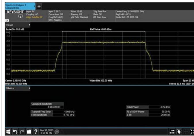
Figure 338: 64QAM 10MHz; 2195MHz – 4G INPUT
