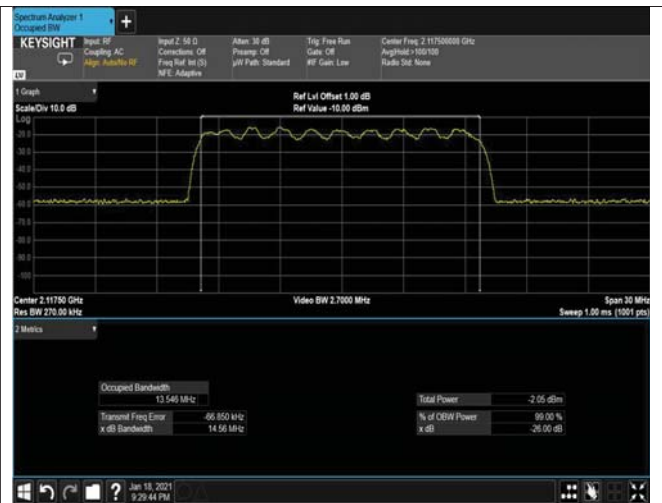
Figure 190: 16QAM 15MHz B.W; 2117.5MHz, 30kHz INPUT
