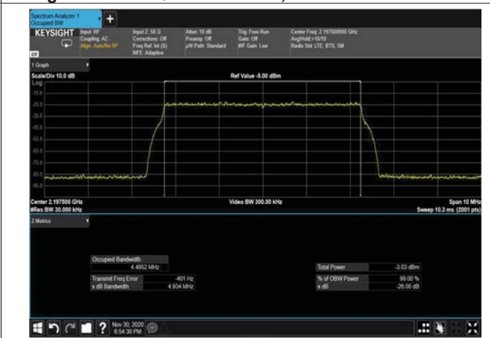
Figure 335: 64QAM 5MHz B.W; 891.5MHz – 4G INPUT
