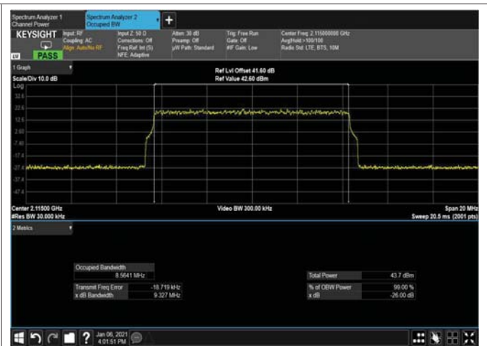
Figure 292: 256QAM 10MHz B.W; 2115MHz, 30kHz OUTPUT
