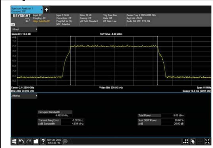
Figure 333: 64QAM 5MHz B.W; 2112.5MHz – 4G INPUT
