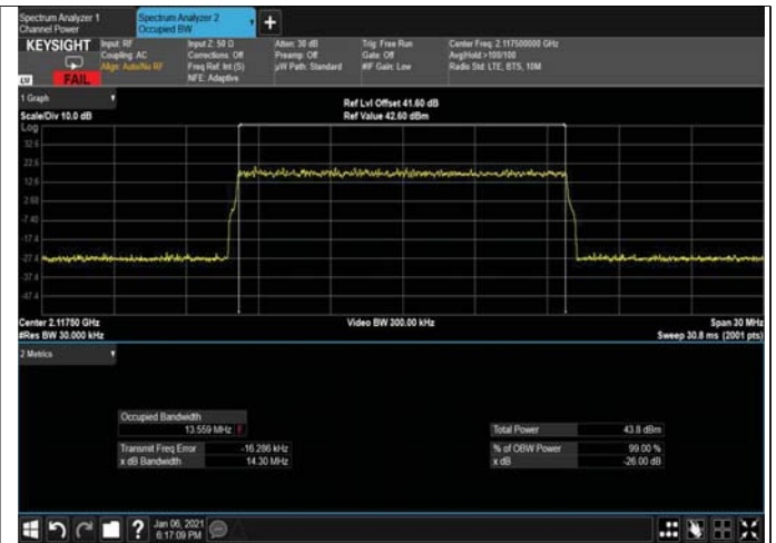
Figure 280: 64QAM 15MHz B.W; 2117.5MHz, 30kHz OUTPUT
