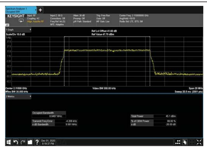
Figure 357: 16QAM 10MHz B.W; 2115MHz – 4G OUTPUT
