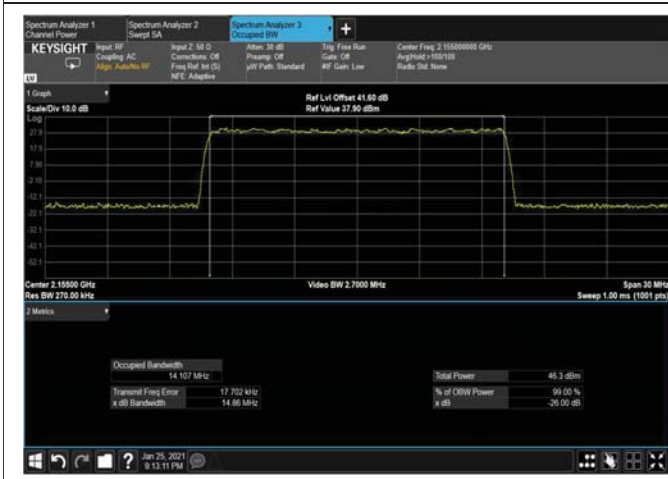
Figure 299: 256QAM 15MHz B.W; 2155MHz, 15kHz OUTPUT
