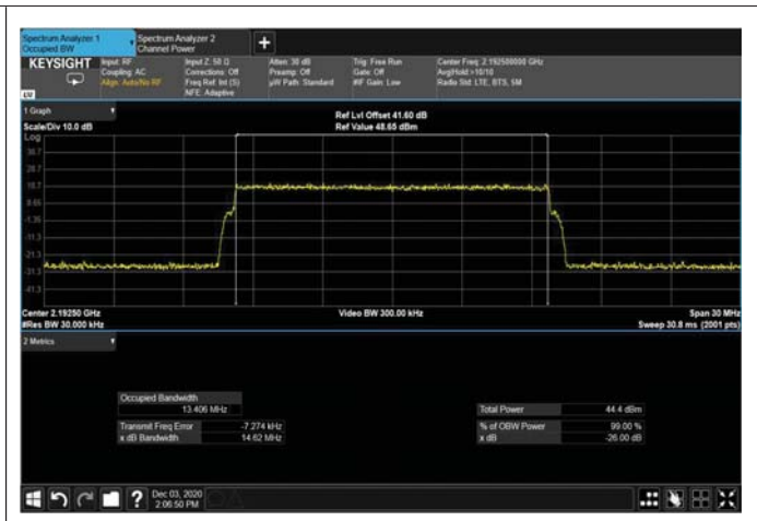
Figure 371: 64QAM 64MHz B.W; 2192.5MHz – 4G OUTPUT
