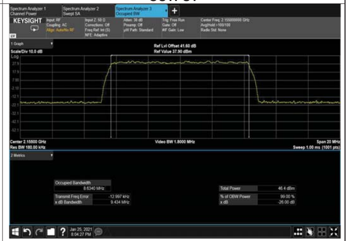
Figure 276: 64QAM 10MHz B.W; 2155.0MHz, 30kHz OUTPUT
