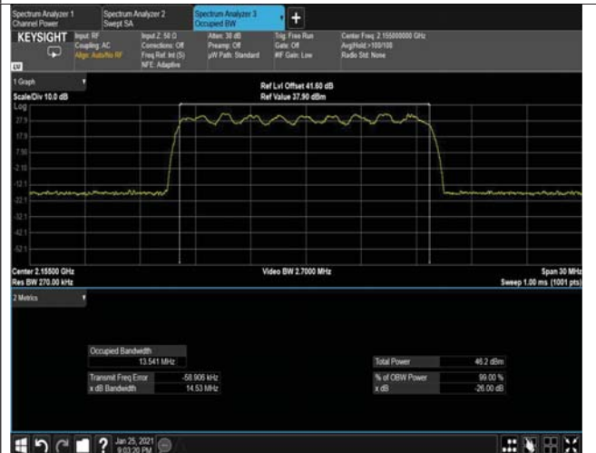
Figure 264: 16QAM 15MHz B.W; 2155.0MHz, 30kHz OUTPUT
