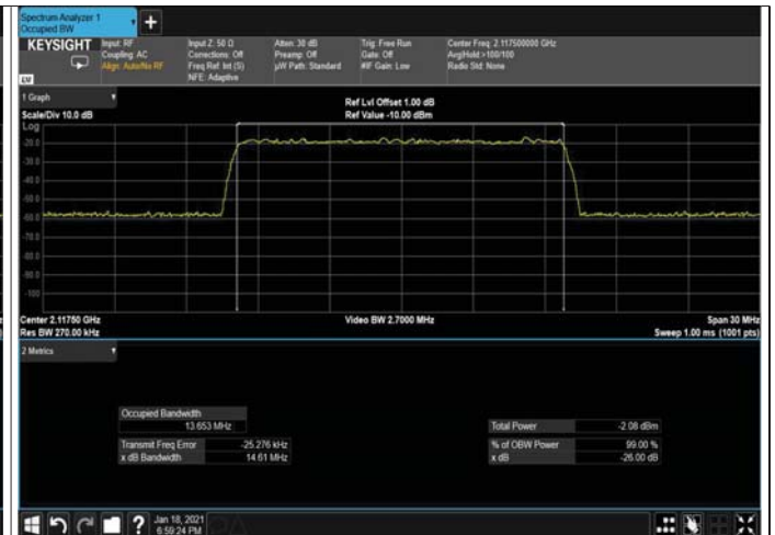
Figure 208: 64QAM 15MHz B.W; 2117.0MHz, 30kHz INPUT
