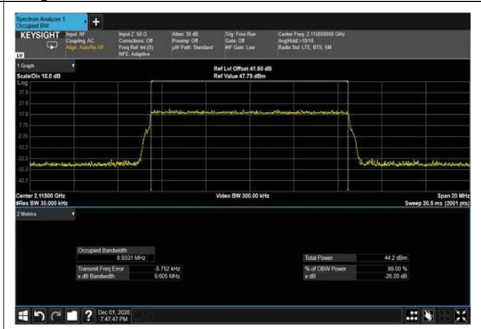
Figure 375: QPSK 10MHz B.W; 2115MHz – 4G OUTPUT
