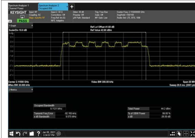
Figure 309: QPSK 10MHz B.W; 2115MHz, 15kHz OUTPUT
