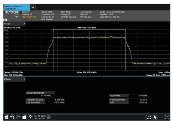
Figure 325: 16QAM 5MHz B.W; 2155MHz – 4G INPUT
