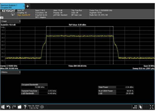
Figure 341: 64QAM 64MHz B.W; 2192.5MHz – 4G INPUT
