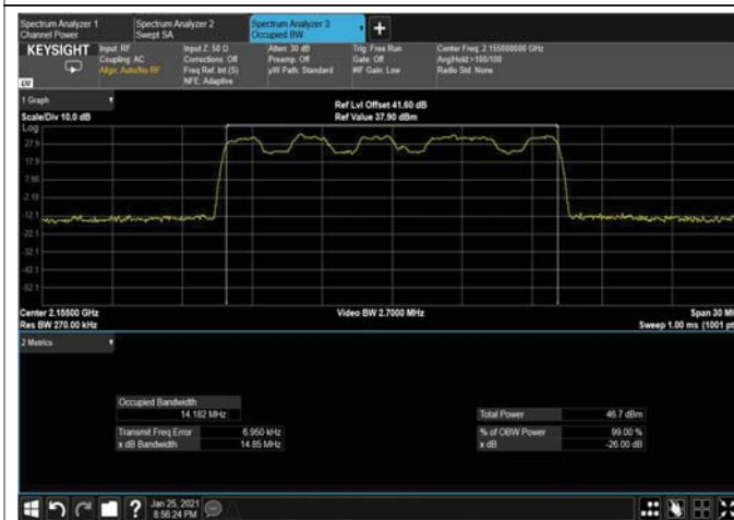
Figure 317: QPSK 15MHz B.W; 2155MHz, 15kHz OUTPUT
