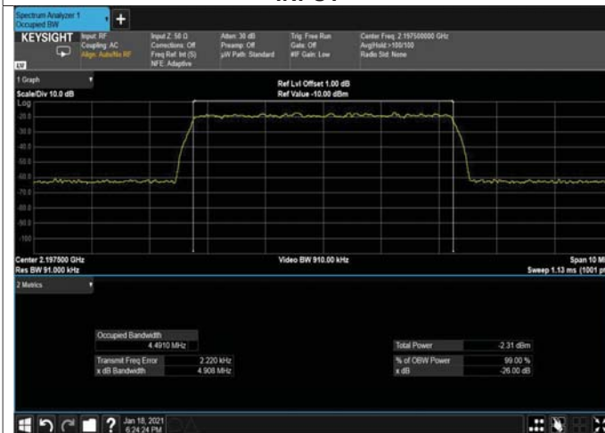
Figure 217: 256QAM 5MHz B.W; 2197.5MHz, 15kHz INPUT
