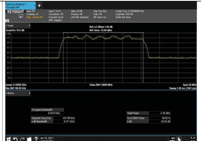
Figure 186: 16QAM 10MHz B.W; 2155.0MHz, 30kHz INPUT
