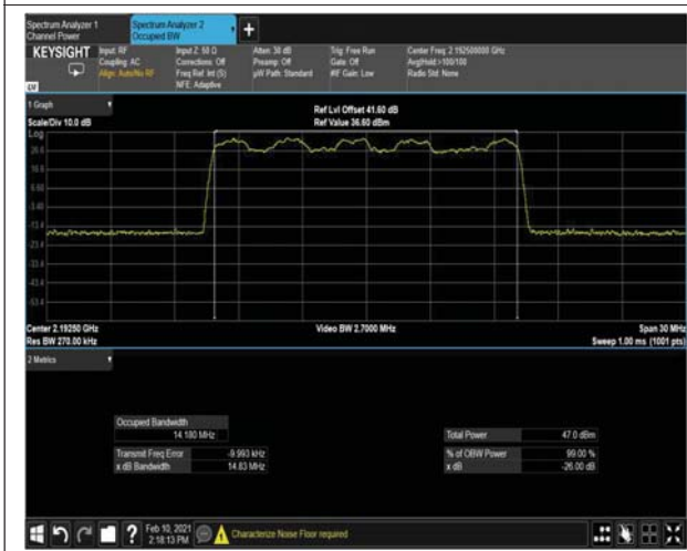
Figure 265: 16QAM 15MHz B.W; 2192.5 MHz, 15kHz OUTPUT
