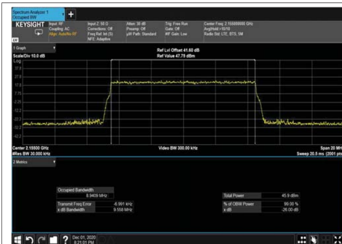
Figure 358: 16QAM 10MHz; 2155MHz – 4G OUTPUT
