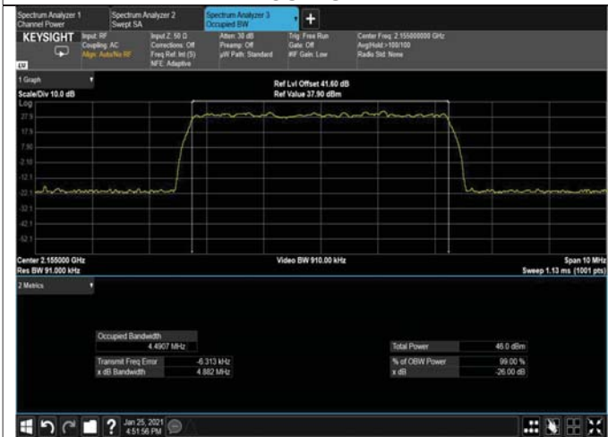
Figure 269: 64QAM 5MHz B.W; 2155.0MHz, 15kHz OUTPUT
