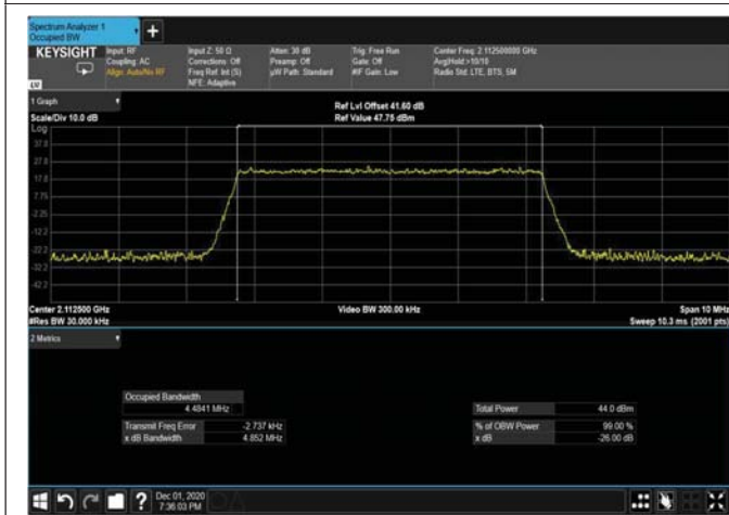
Figure 372: QPSK 5MHz B.W; 2112.5MHz – 4G OUTPUT
