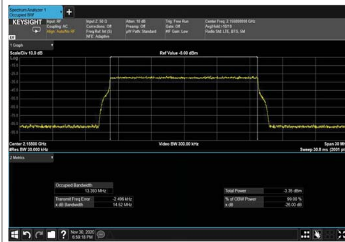
Figure 340: 64QAM 15MHz B.W; 2155MHz – 4G INPUT
