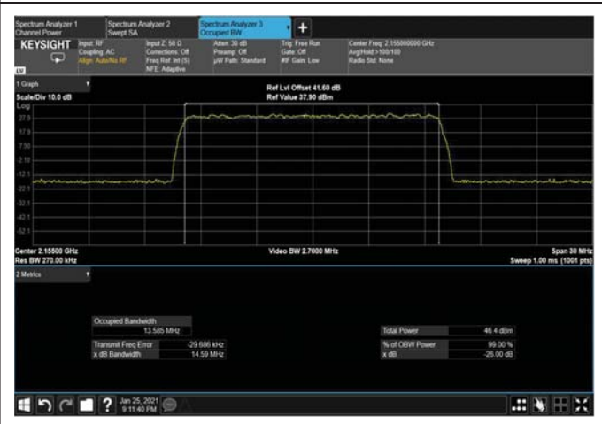
Figure 300: 256QAM 15MHz B.W; 2155MHz, 30kHz OUTPUT
