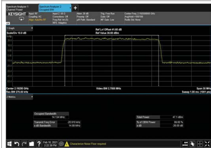
Figure 283: 64QAM 15MHz B.W; 2192.5MHz, 15kHz OUTPUT
