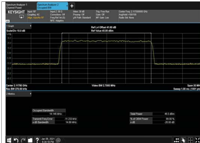
Figure 279: 64QAM 15MHz B.W; 2117.5MHz, 15kHz OUTPUT
