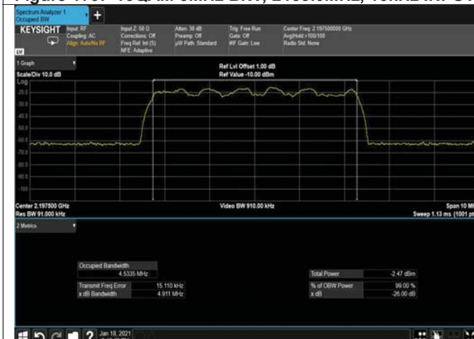
Figure 181: 16QAM 5MHz B.W; 2197.0MHz, 15kHz INPUT
