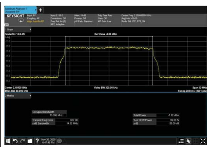
Figure 331: 16QAM 15MHz B.W; 2155MHz – 4G INPUT
