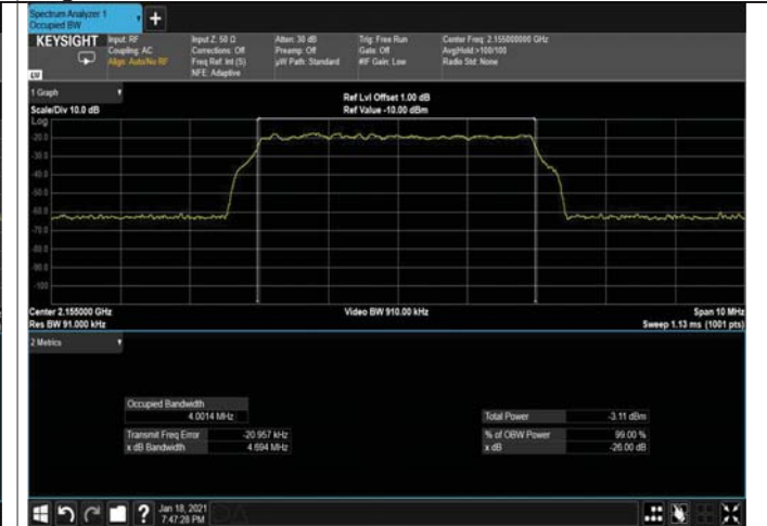
Figure 198: 64QAM 5MHz B.W; 2155.0MHz, 30kHz INPUT
