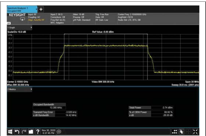
Figure 349: QPSK 15MHz B.W; 2155MHz – 4G INPUT
