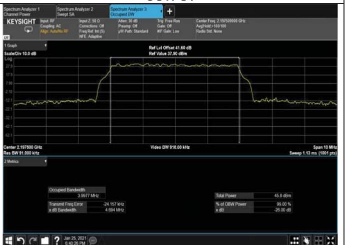
Figure 272: 64QAM 5MHz B.W; 2197.5MHz, 30kHz OUTPUT
