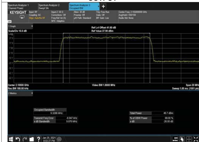
Figure 275: 64QAM 10MHz B.W; 2155.0MHz, 15kHz OUTPUT
