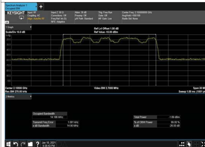
Figure 245: QPSK 15MHz B.W; 2155.0MHz, 15kHz INPUT
