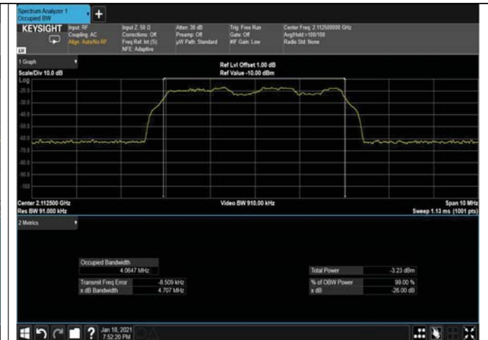
Figure 178: 16QAM 5MHz B.W; 2112.5MHz, 30kHz INPUT
