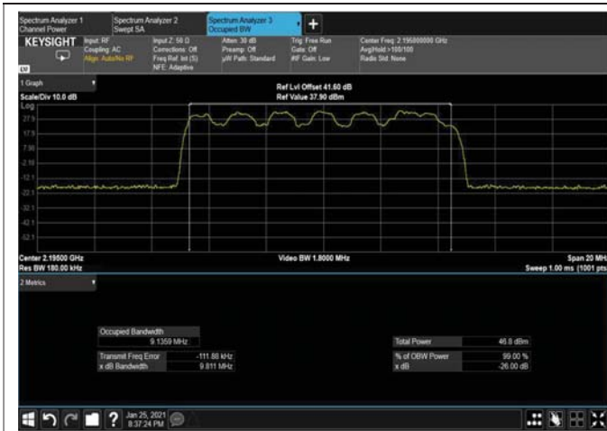
Figure 313: QPSK 10MHz B.W; 2195MHz, 15kHz OUTPUT
