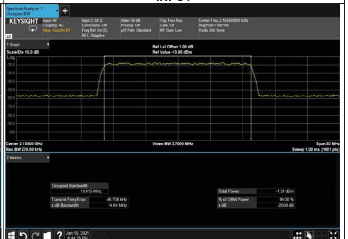
Figure 228: 256QAM 15MHz B.W; 2155.0MHz, 30kHz INPUT
