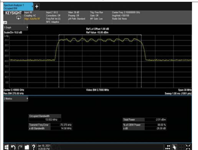
Figure 192: 16QAM 15MHz B.W; 2155.0MHz, 30kHz INPUT
