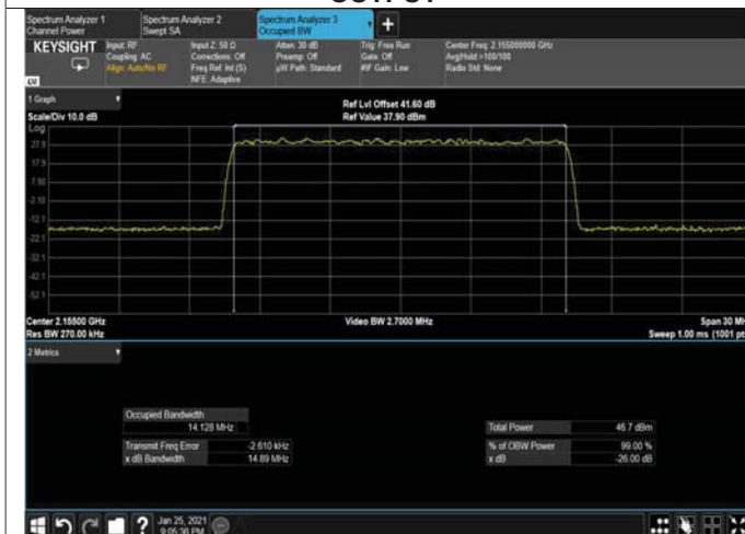
Figure 281: 64QAM 15MHz B.W; 2155.0MHz, 15kHz OUTPUT
