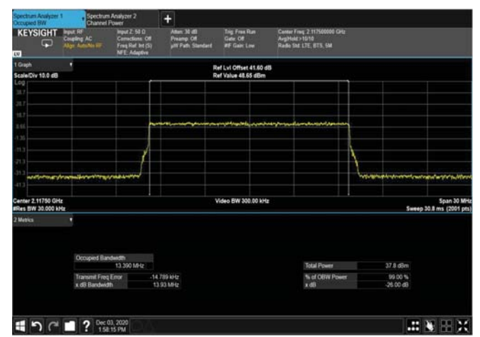
Figure 369: 64QAM 15MHz B.W; 2117.5MHz – 4G OUTPUT
