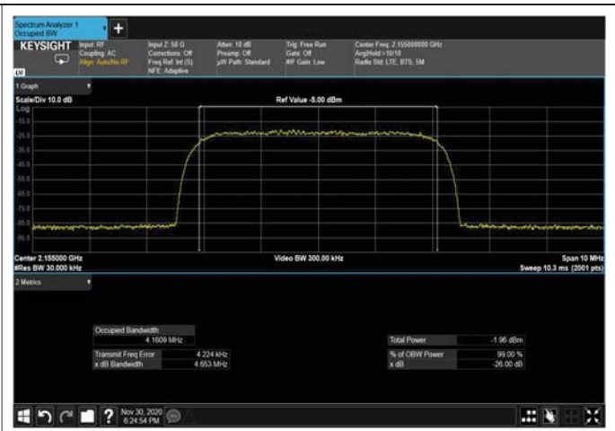
Figure 322: WCDMA 5MHz B.W; 2155.0MHz – 3G INPUT
