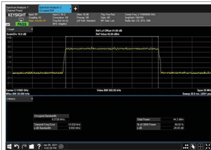
Figure 291: 256QAM 10MHz B.W; 2115MHz, 15kHz OUTPUT
