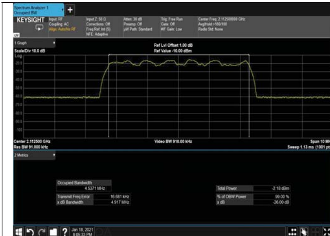
Figure 177: 16QAM 5MHz B.W; 2112.5MHz, 15kHz INPUT
