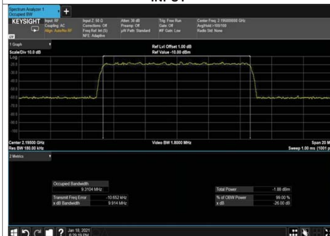
Figure 223: 256QAM 10MHz B.W; 2195.0MHz, 15kHz INPUT
