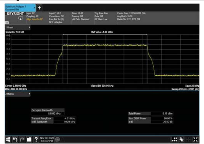
Figure 327: 16QAM 10MHz B.W; 2115MHz – 4G INPUT
