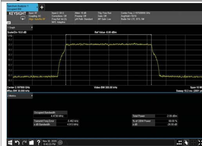
Figure 326: 16QAM 5MHz B.W; 2197.5MHz – 4G INPUT
