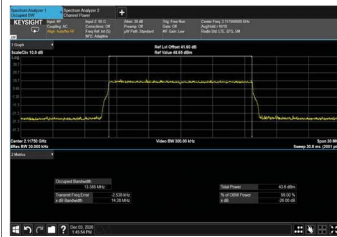
Figure 378: QPSK 15MHz B.W; 2117.5MHz – 4G OUTPUT
