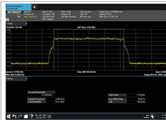
Figure 330: 16QAM 15MHz B.W; 2117.5MHz – 4G INPUT
