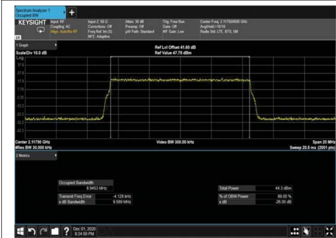
Figure 366: 64QAM 10MHz B.W; 2115MHz – 4G OUTPUT
