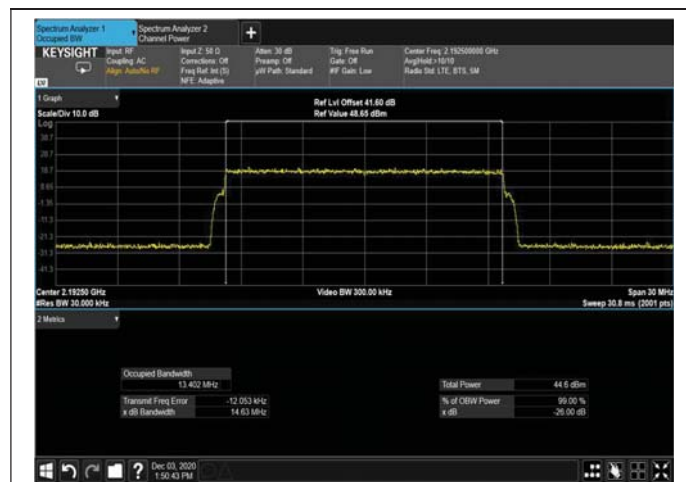
Figure 380: QPSK 15MHz B.W; 2192.5MHz – 4G OUTPUT
