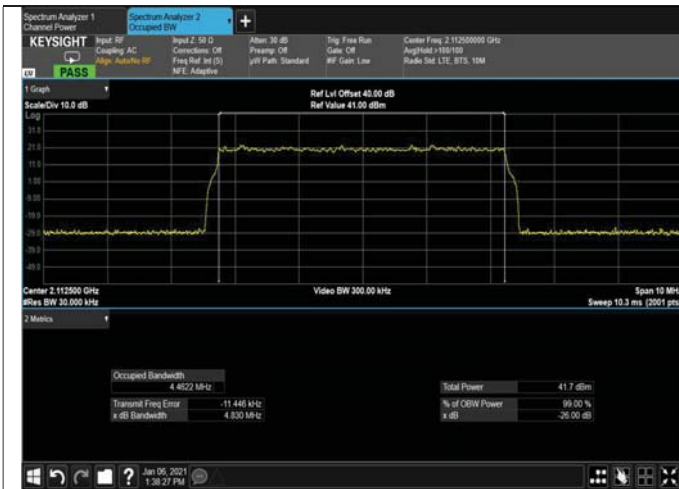
Figure 267: 64QAM 5MHz B.W; 2112.5MHz, 15kHz OUTPUT
