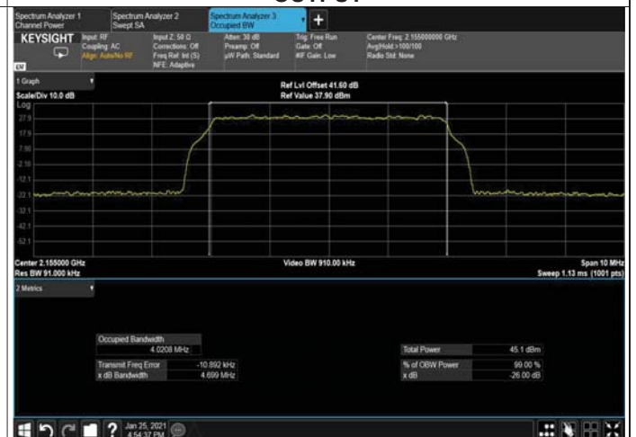
Figure 288: 256QAM 5MHz; 2155.0MHz B.W, 30kHz OUTPUT
