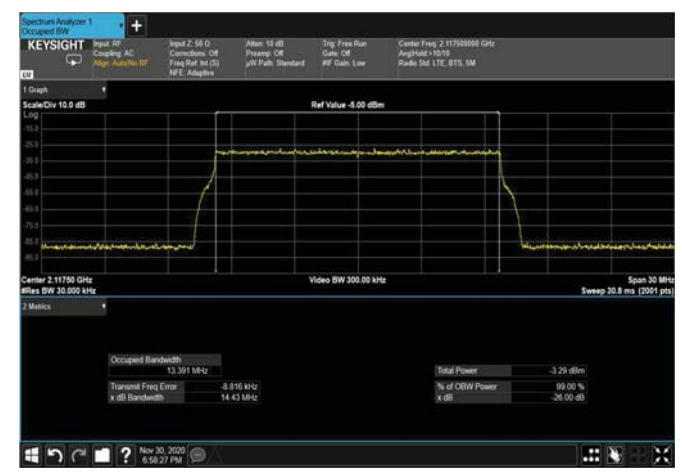
Figure 339: 64QAM 15MHz B.W; 2117.5MHz – 4G INPUT
