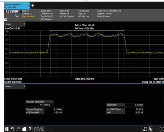
Figure 193: 16QAM 15MHz B.W; 2192.5MHz, 15kHz INPUT
