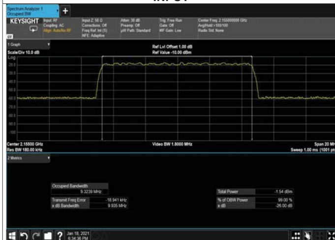
Figure 221: 256QAM 10MHz B.W; 2155.0MHz, 15kHz INPUT
