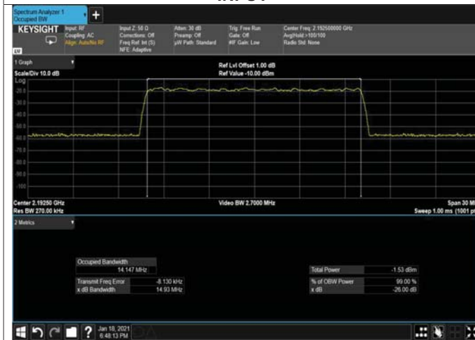
Figure 229: 256QAM 15MHz B.W; 2192.5MHz, 15kHz INPUT
