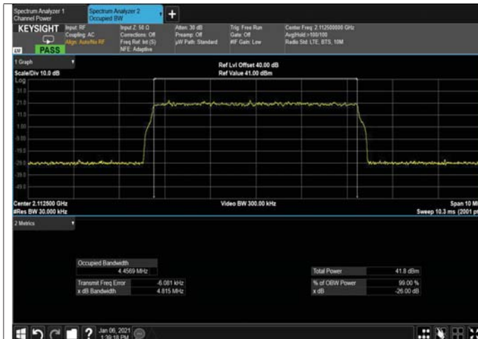
Figure 285: 256QAM 5MHz B.W; 2112.5MHz, 15kHz OUTPUT
