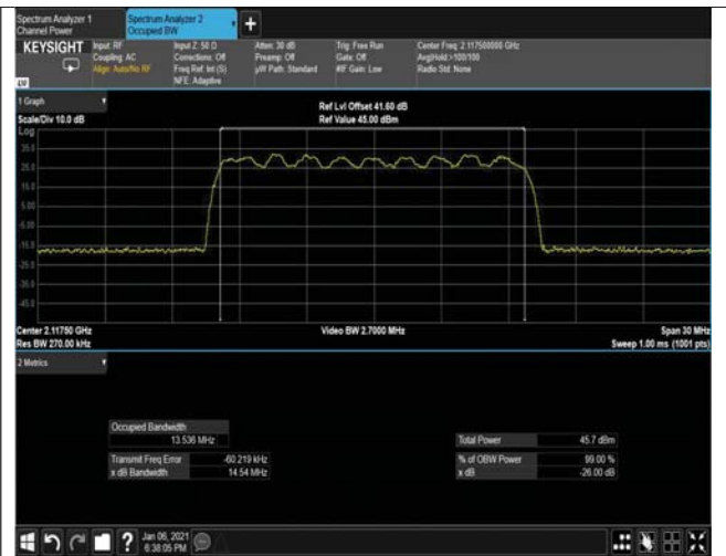
Figure 262: 16QAM 15MHz B.W; 2117.5MHz, 30kHz OUTPUT
