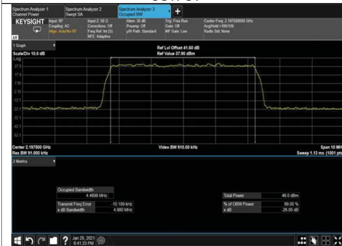
Figure 271: 64QAM 5MHz B.W; 2197.5MHz, 15kHz OUTPUT
