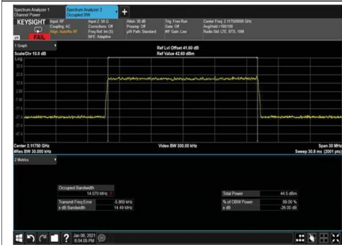
Figure 297: 256QAM 15MHz B.W; 2117.5MHz, 15kHz OUTPUT
