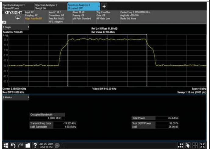
Figure 270: 64QAM 5MHz B.W; 2155.0MHz, 30kHz OUTPUT
