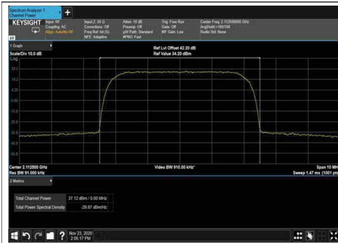
Figure 81: WCDMA 5MHz B.W; 2112.5MHz – 3G
