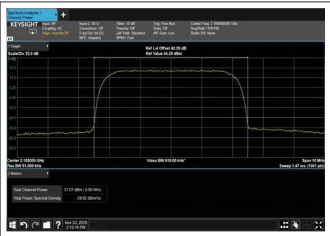
Figure 82: WCDMA 5MHz B.W; 2155.0MHz – 3G
