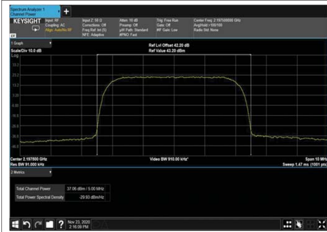
Figure 83: WCDMA 5MHz B.W; 2197.5MHz – 3G
