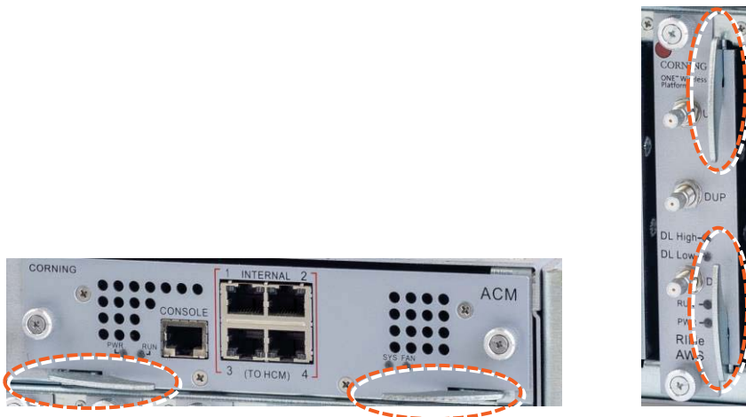
Figure 5: Module Captive Screws and Ejectors
