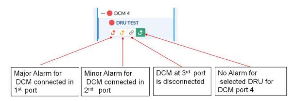
Figure 16: Example – alarms for connected DCMs
