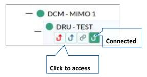
The number of arrows is the number of DCMs the DRU is connected to. The user may skip between the DRU's connected DCMs by clicking the arrow of the desired DCM.
