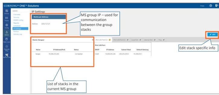
All HCMs in the MS-group are automatically updated when one stack in the group is updated. The update is done using the Multicast Address which is used for communication between the stacks in the group.
