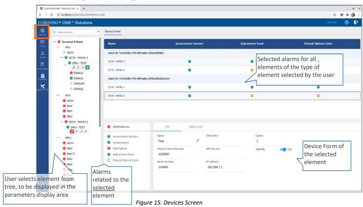
Note: The same DRU may appear in the system tree multiple times if it is connected to different DCMs.
