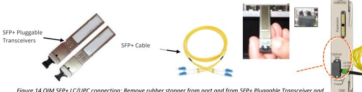
Figure 14 OIM SFP+ LC/UPC connection: Remove rubber stopper from port and from SFP+ Pluggable Transceiver and insert the SFP+ Pluggable Transceivers (hot-pluggable optical transceiver module) into the port.
