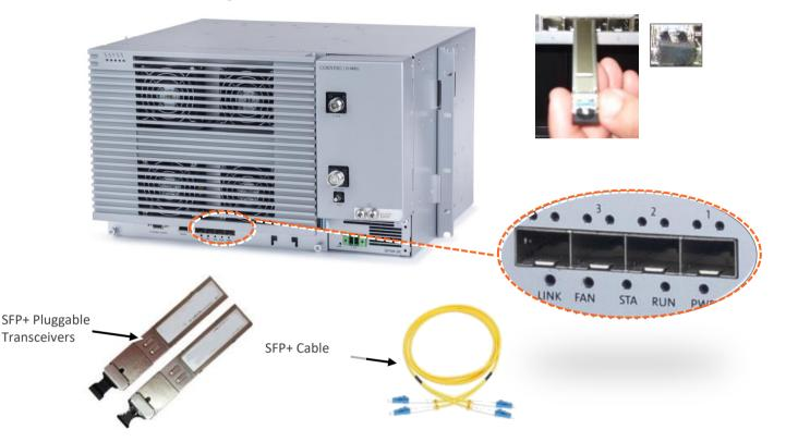
Figure 8 Remove rubber stopper from port and from SFP+ Pluggable Transceiver and insert the SFP+ Pluggable Transceivers (hot-pluggable optical transceiver module) into the port.
