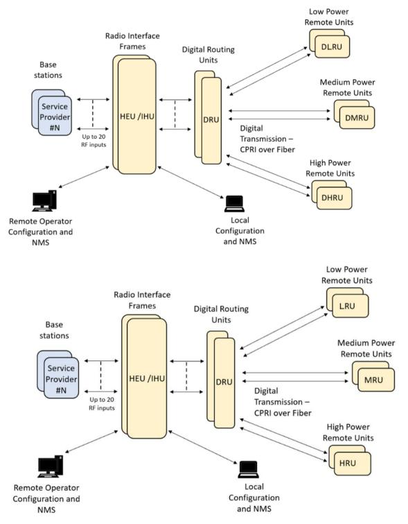
Corning Everon<sup>™</sup> 6000 allows combining between Optical Network Evolution (ONE) platform, and the fully digital Corning Building Wireless System (BWS) platform, which incorporates the digital distribution units – Digital Router Unit (DRU) and remotes.
