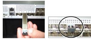
Figure 2 Remove rubber stopper from port and from SFP+ Pluggable Transceiver
