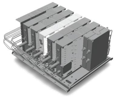
The HRU is a high power modular remote antenna unit which provides 43 dBm output RF power per service module, and native support of 2x2 MIMO antenna scheme. The HRU modular structure enables set ups of up to 8 service modules in 600/700 MHz Low/700 MHz High/FirstNet, 800/850 MHz, EAWS, PCS, WCS and 2.5GHz TDD.
