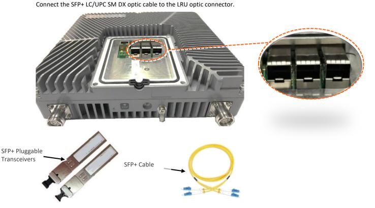
Figure 3 Remove rubber stopper from port and from SFP+ Pluggable Transceiver and insert the SFP+ Pluggable Transceivers (hot-pluggable optical transceiver module) into the port.
