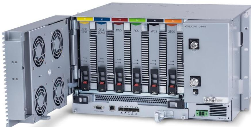
The MRU is a medium power modular remote antenna unit with a single antenna port. The output power for the lower bands: 600/700 MHz Low/700 MHz High/FirstNet, 800/850 MHz is 33 dBm and the output power for the medium bands EAWS, PCS, WCS and 2.5GHz TDD is 37dBm.
