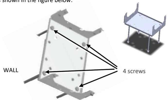
2. For a single unit: mount the LRU on the bracket, using 4 screws
