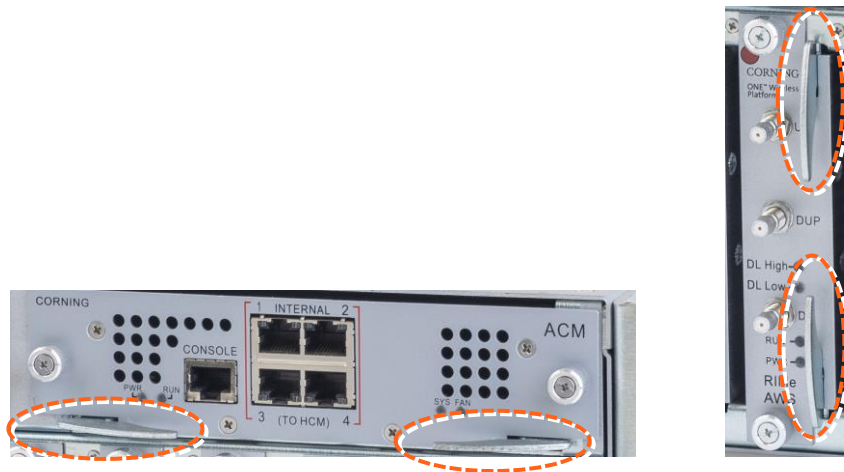
Figure 13: Module Captive Screws and Ejectors
