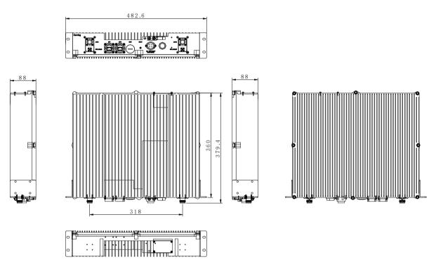
Figure 71. dMRU Dimensions - Without Fan
