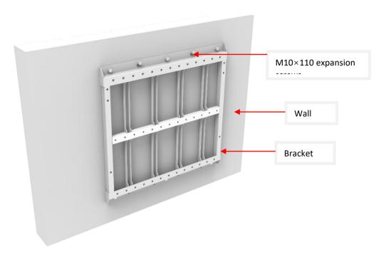
Figure 95. Wall mounted installation
