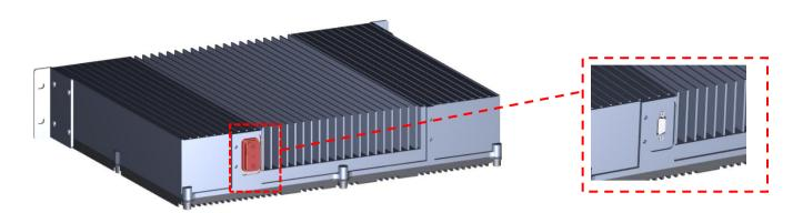
Figure 77. Fan Connection
