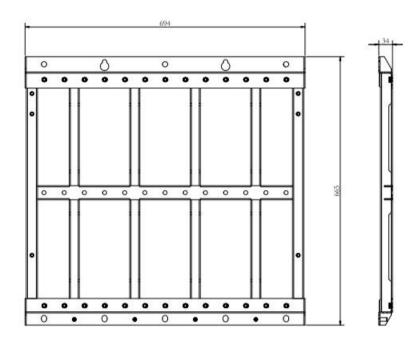
Figure 88.dHRU Bracket Dimension
