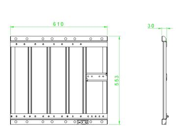
Figure 81.dMRU bracket dimensions
