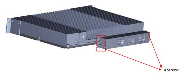
Figure 79. Fan Installation
