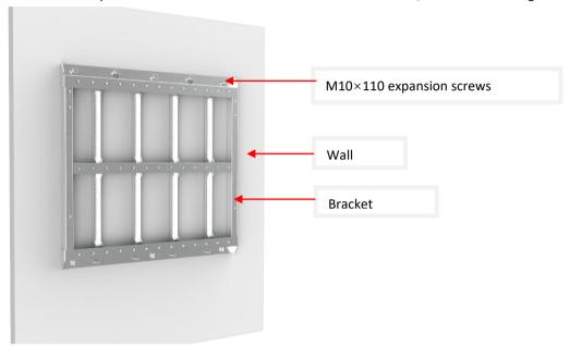
Figure 110. Wall mounted installation
