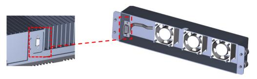
Figure 78. Fan Connection with DB15
