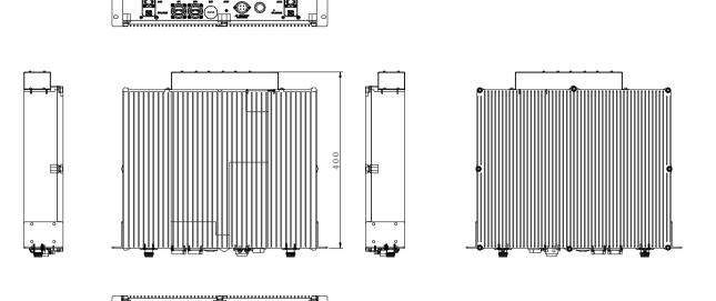
Figure 72. dMRU Dimensions - with Fan
