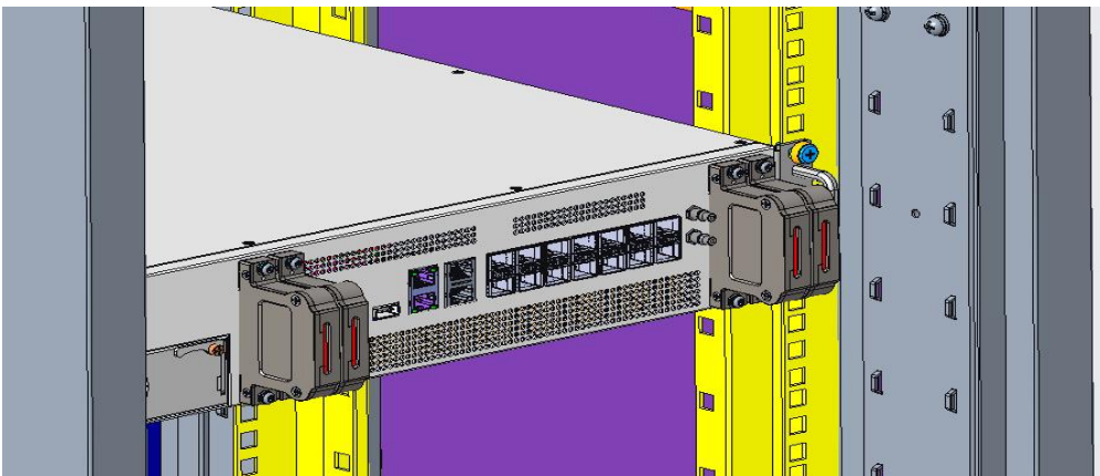
Figure 37. DCU RF Cable Plug Installation
