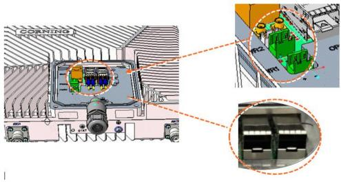
Figure 40. Power Socket/optical ports in dLRU
