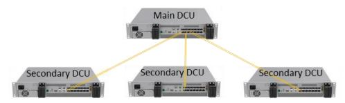
Figure 12. DCU Star Connection
