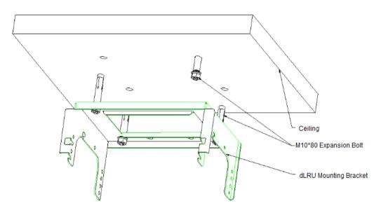
Figure 48. Mounting Bracket Installation Diagram
