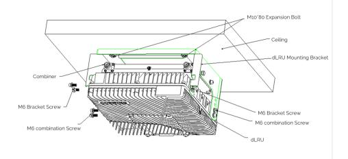
Figure 50. Low-Band dLRU Installation
