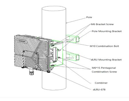
Figure 56. Installation Diagram of dLRU Pole
