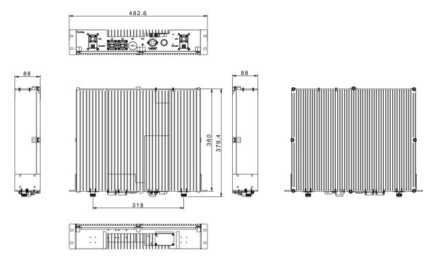
Figure 67. dMRU Dimensions - Without a Fan
