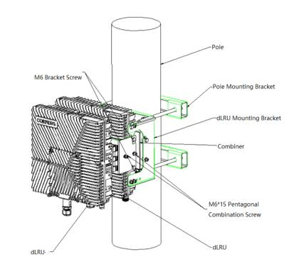
Figure 57. Dual Unit Installation Diagram
