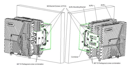
Figure 52. dLRU Installation Diagram
