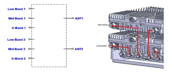
Figure 65. The Entire System Connection
