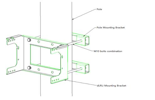
Figure 53. Pole-Mounting Diagram
