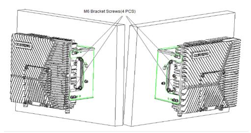
Figure 51. M6 Bracket Screw Holes
