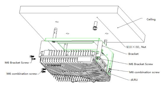
Figure 45. Single Unit Ceiling Installation
