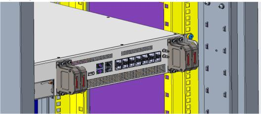
Figure 34. DCU RF Cable Plug Installation
