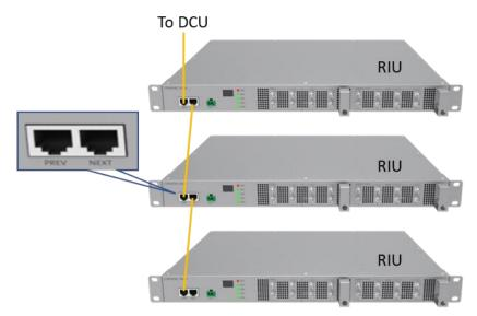
Figure 6. RIU-TDD Monitoring Diagram
