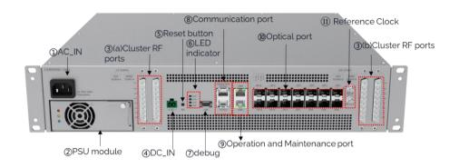
Figure 13. DCU Interface (front view)
