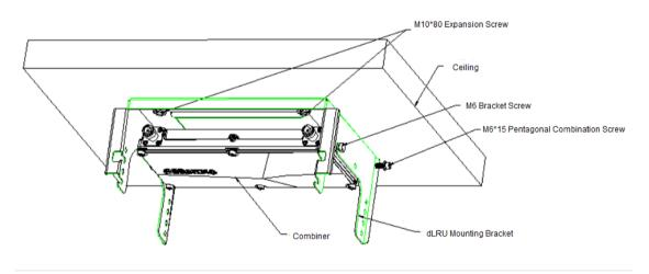
Figure 49. Combiner Installation Diagram
