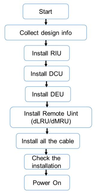
Figure 25. The Installation Process
