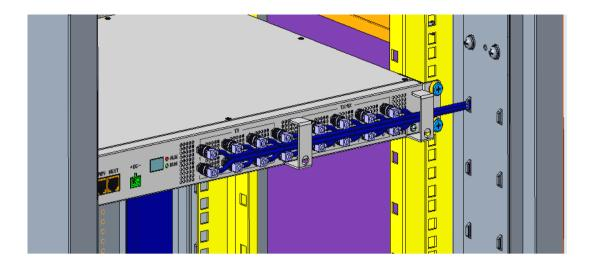
Figure 29. RIU Rack Installation with Cables
