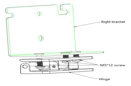
Figure 46. Right Bracket and Hinge Installation
