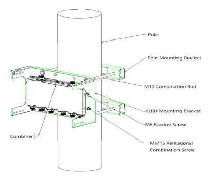
Figure 55. Installation Diagram of the Combiner
