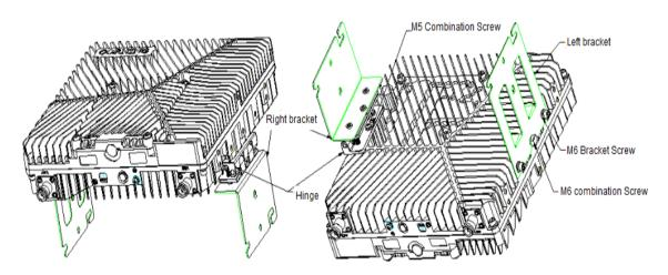
Figure 47. Installation of the Left and Right Brackets and Device Bracket
