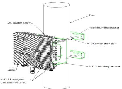
Figure 54. Diagram of Pole Installation for Single Unit
