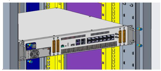
Figure 33. Installation Diagram of DCU in the Rack
