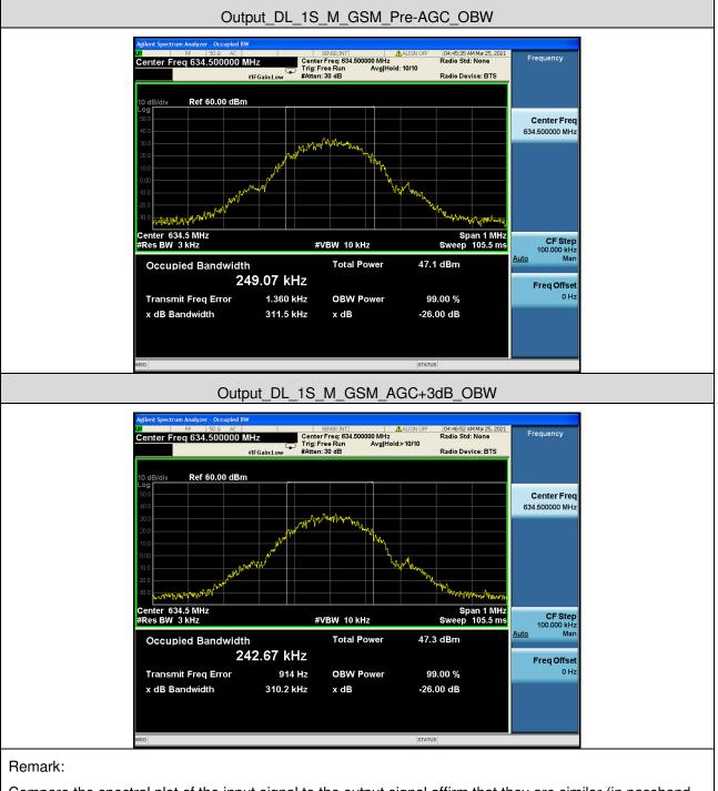
Compare the spectral plot of the input signal to the output signal affirm that they are similar (in passband and roll off characteristic features and relative spectral locations). The test result complies with the requirement.
