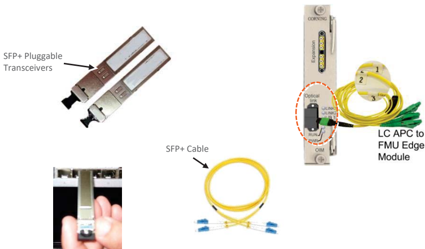
Figure 6 OIM SFP+ LC/APC connection: Remove rubber stopper from port and from SFP+ Pluggable Transceiver and insert the SFP+ Pluggable Transceivers (hot-pluggable optical transceiver module) into the port.
