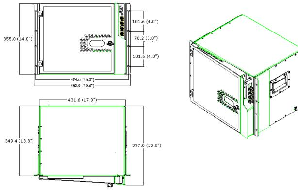
The following figure provides the dimensions for the MA2000 Rack Model.
