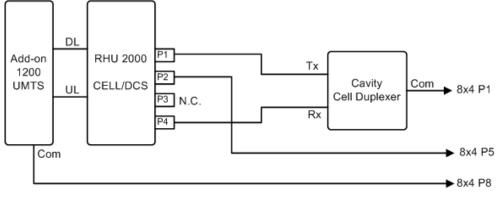
Figure 5-5. Cell/DCS and UMTS Configuration
