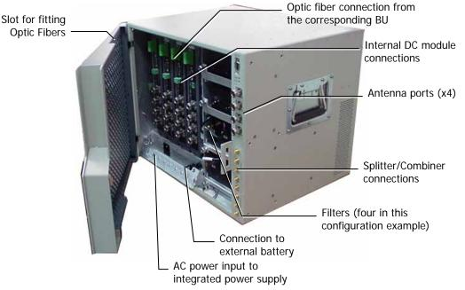
Figure 2-2. MA2000 MRC Open Cabinet View (without internal connections)
