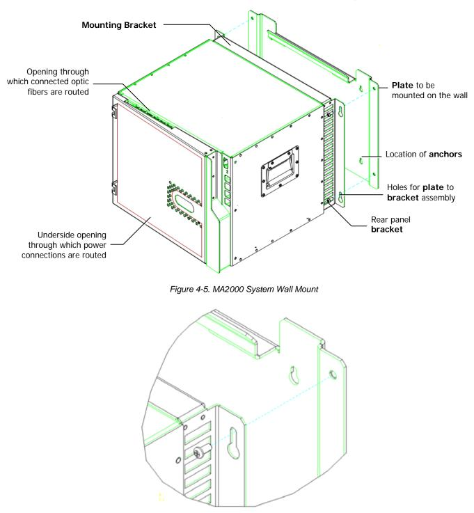
The wall installation MA2000 Remote Cabinet is supplied with a plate that is to be mounted on the wall and a bracket that is assembled on the rear of the MA2000 system.
