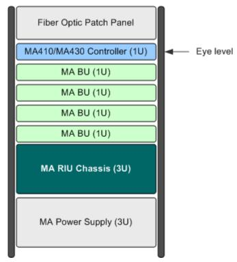
The following figure shows a typical installation for a two field design.
