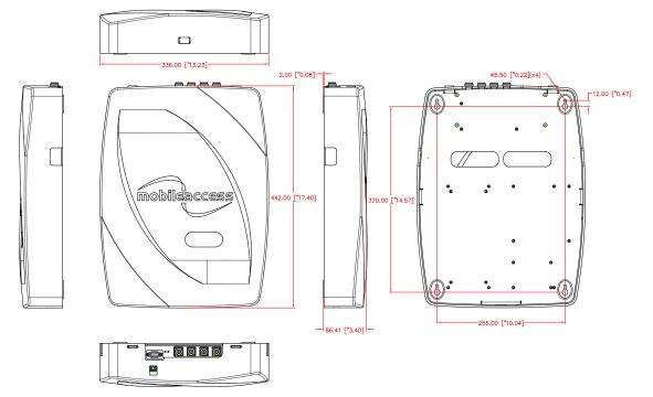
The following figure shows the RIU Lite mechanical drawing
