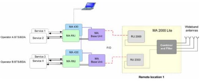
Figure 1-4. Example of MA2000-Lite Architecture
