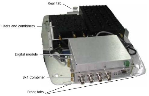
Figure 2-5. MA2000-Lite Internal Units
