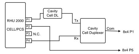
Figure 5-2. Single Cell/PCS Connections
