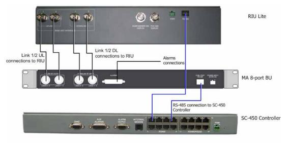
Figure 4-3. BU Rear Panel Connections
