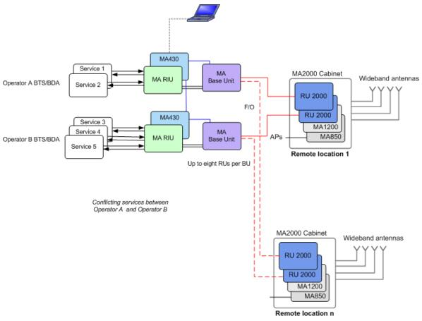
Figure 1-3. Example of MA2000 Cabinet Architecture
