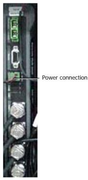
Figure 4-10. MA2000 RU Fiber Optic and internal power connections
