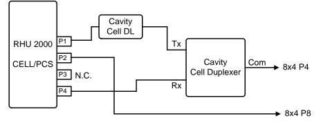
Figure 5-3. Additional Cell/PCS Connections
