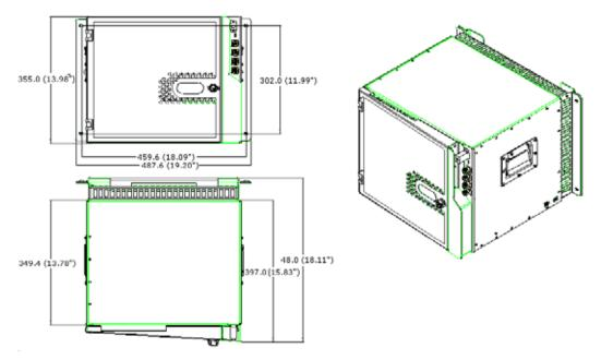
Figure 4-4. MA2000 Cabinet Wall Mount Dimensions
