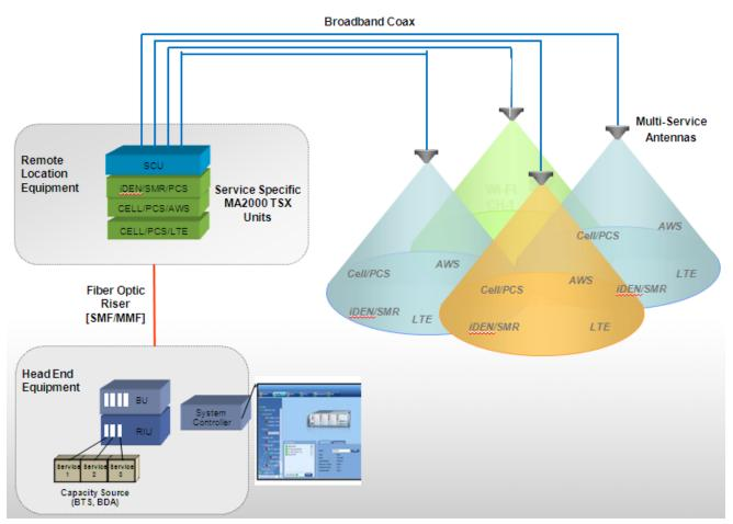
For end-to-end control, controllers installed at the head-end provide direct interface to the MA elements and through them, control over the remote end elements.
