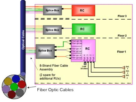
The following figure illustrates fiber optic routing to Remote Cabinets.
