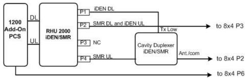
Figure 5-1. iDEN/SMR and PCS Connections
