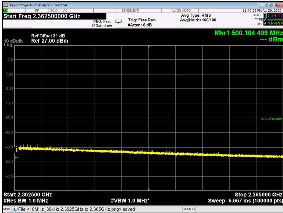
Figure 57: Spurious Emissions at Antenna Terminal 16QAM, 2355.0MHz, B.W. 10MHz, Sub Carrier 60kHz
