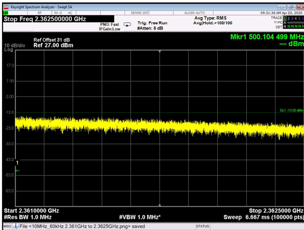
Figure 40: Spurious Emissions at Antenna Terminal 16QAM, 2355.0MHz, B.W. 10MHz, Sub Carrier 15kHz
