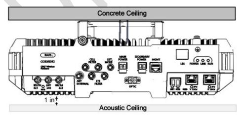
Figure 4-1.Example of (Concrete) Ceiling Installation of Mounting Bracket (RAU5x without External Antenna)
