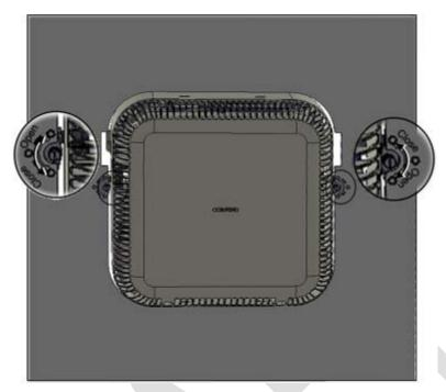
Figure 4-12. Closing Rotary Knobs
