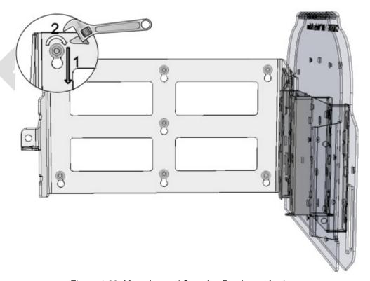
Figure 4-20. Mounting and Securing Bracket to Anchors
