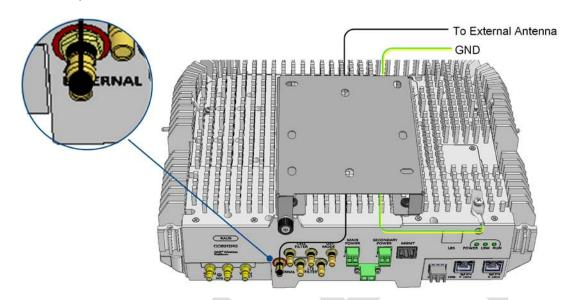
Figure 4-25. RAU5/RAU5x External Antenna Connection
