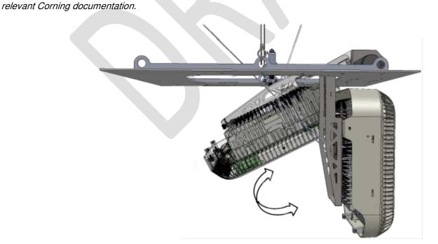
Figure 4-11 Verifying that Cable Path is not Obstructed
