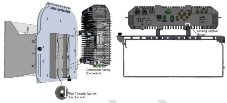
Figure 4-21. Mounting and Securing RAU5x Unit
