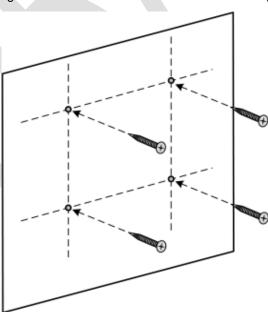
Figure 4-37. Marking and Inserting Anchors in Wall
