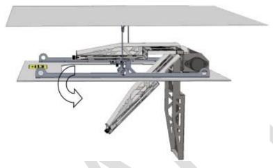
Figure 4-7. Lowering Lift Bracket
