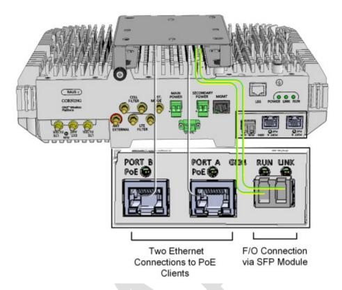
Figure 4-31. GEM Module Interfaces Connections
