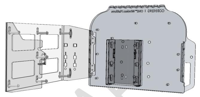
Figure 4-19. Drilling Anchors through Wall-Mount Bracket Keyholes
