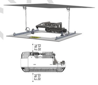
Figure 4-6. Installing "Top Bracket" Plate
