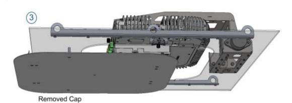
Figure 4-17. Removing Cap
