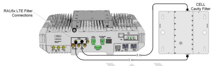
Figure 4-39. Example of RAU5x External CELL Filter Connections
