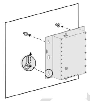
Figure 4-38. Mounting Cavity Filter on Wall
