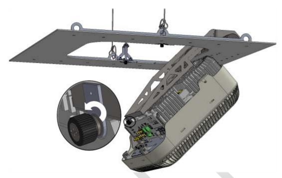
Figure 4-9 Closing Lift Bracket Captive Screw
