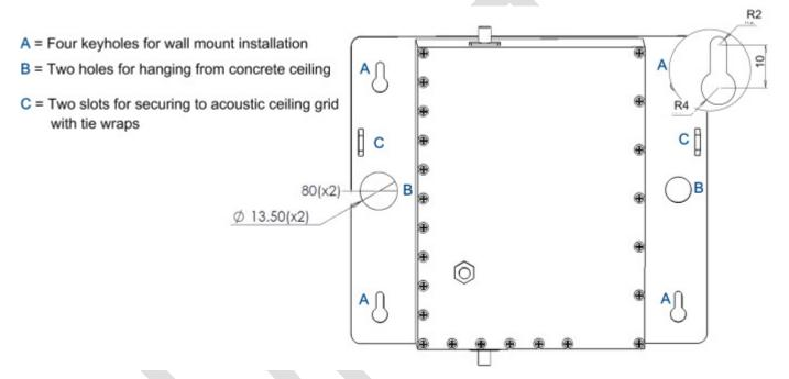
Figure 4-34. Cavity Filter Dimensions and Mounting Holes
