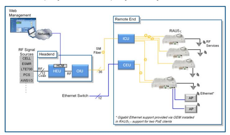
Figure 1-1. Corning ONE Basic Architecture
