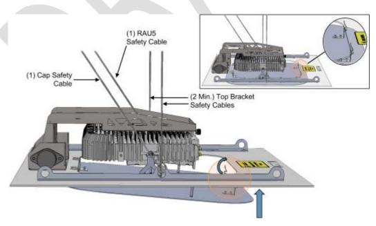
Figure 4-16. Hooking Narrow Fasteners in Place
