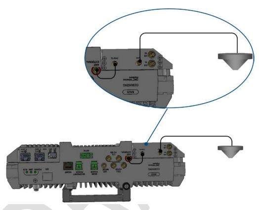
Figure 4-27. RF Connections for RAU5x with RxU2325
