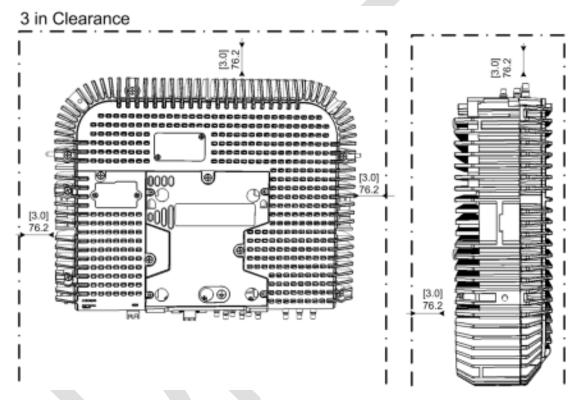
Figure 4-18. Required Three IN Clearance from Surface
