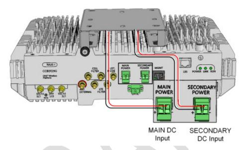
Figure 4-30. RAU5x MAIN and SECONDARY DC Input Connections
