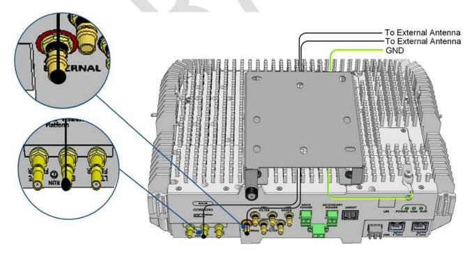
Figure 4-26. RAU5/RAU5x with RxU - External Antenna Connections
