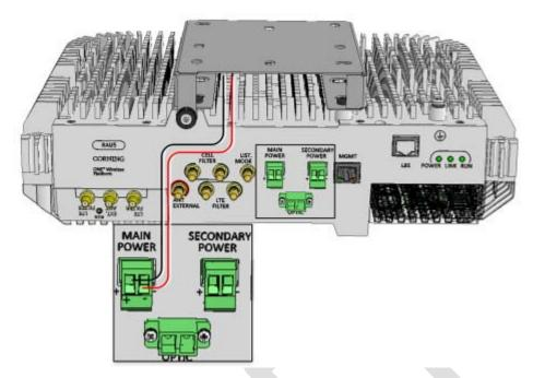
Figure 4-29 RAU5x Main Power DC Connections
