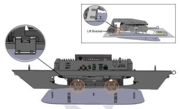
Figure 4-15. Hooking Cap to Top Bracket plate
