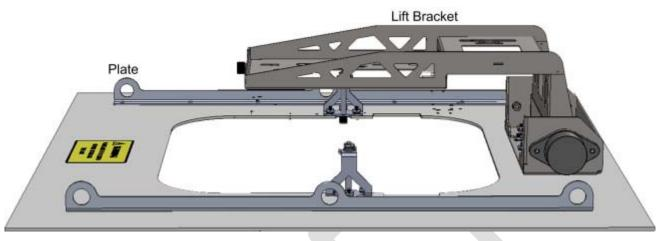
Figure 4-5. "Top Bracket" Assembly Lift Bracket and Plate
