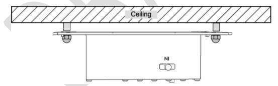
Figure 4-35. Illustration of Cavity Filter Mounted on Ceiling
