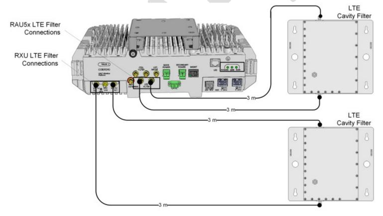
Figure 4-40. Example of RAU5x and RXU External LTE Filter Connections
