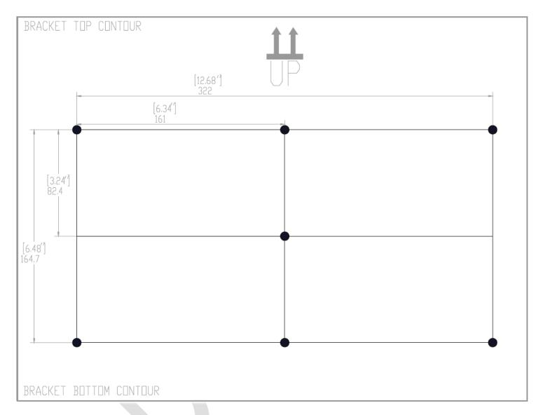
Figure 5-4. RAU5 Wall Mount Drilling Pattern Dimensions
