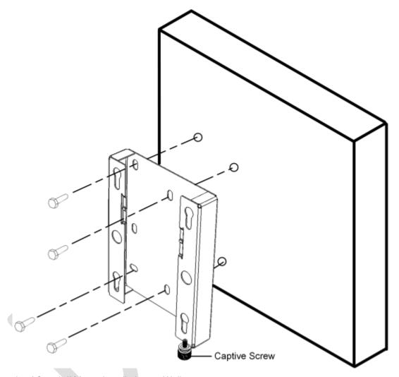
Figure 4-2. Example of Standoff Mount Installation on Wall
