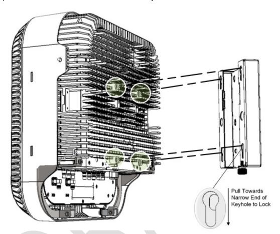
Figure 4-3. Mounting RAU5x onto Bracket
