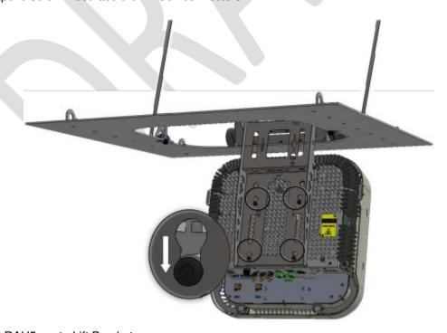
Figure 4-8. Mounting RAU5x onto Lift Bracket
