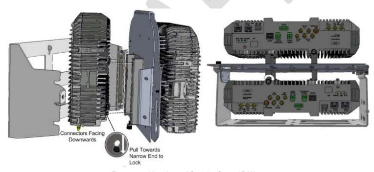
Figure 4-22. Mounting and Securing Second RAU5x
