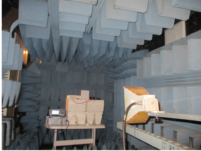
Figure 5. Radiated Emission Test 1.0 - 8.0GHz
