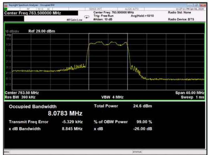
Figure 170: 16QAM 10MHz C.S; 763.5MHz, 60kHz Output
