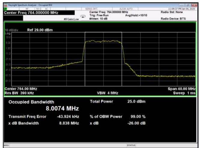
Figure 186: 64QAM 10MHz B.W.; 764.0MHz, 60kHz Output
