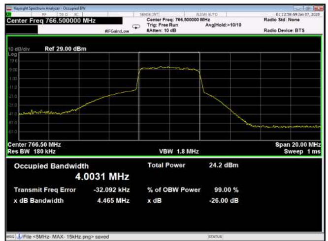
Figure 192: 256QAM 5MHz B.W.; 766.5MHz, 30kHz Output
