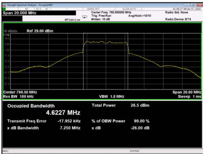
Figure 187: 256QAM 5MHz B.W.; 760.5MHz, 15kHz Output
