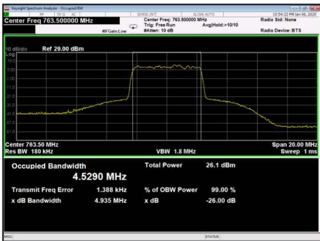
Figure 173: 64QAM 5MHz B.W.; 763.5MHz, 15kHz Output
