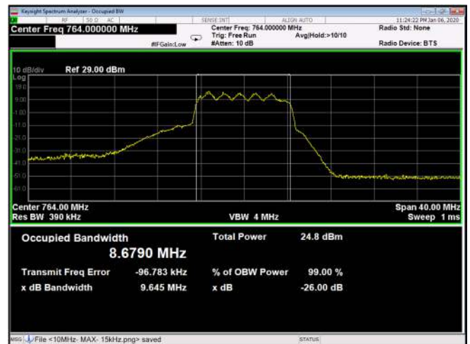
Figure 168: 16QAM 10MHz B.W.; 764.0MHz, 30Hz Output
