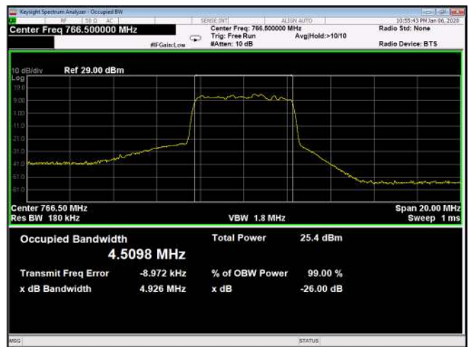
Figure 174: 64QAM 5MHz C.S; 766.5MHz, 15kHz Output
