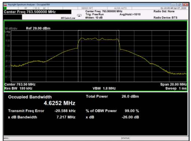
Figure 188: 256QAM 5MHz B.W.; 763.5MHz, 15kHz Output
