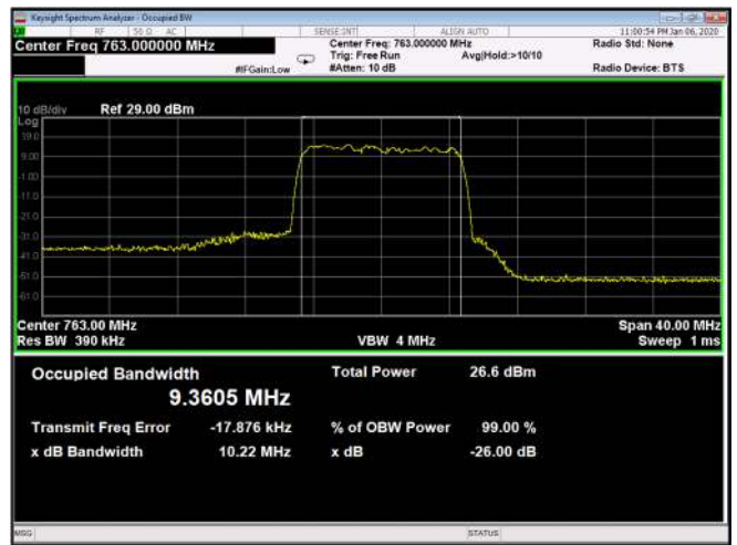
Figure 178: 64QAM 10MHz B.W.; 763.0MHz, 15kHz Output
