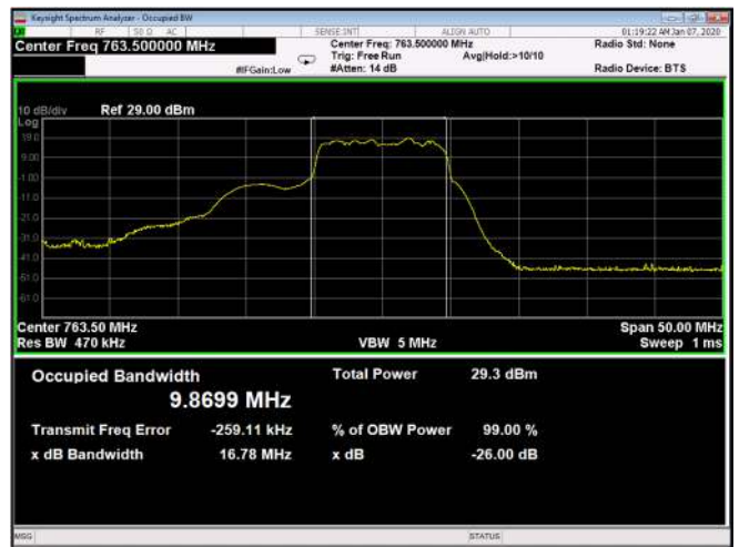
Figure 194: 256QAM 10MHz B.W.; 763.5MHz, 15kHz Output
