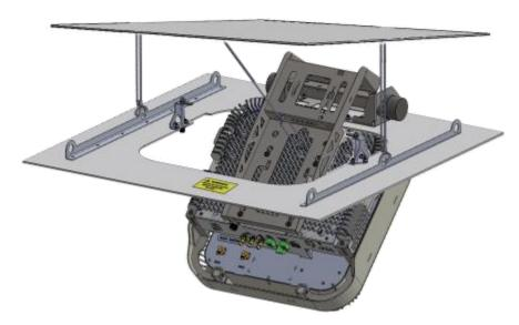
Figure 4-11. Securing RAU5x to Permanent Structure
