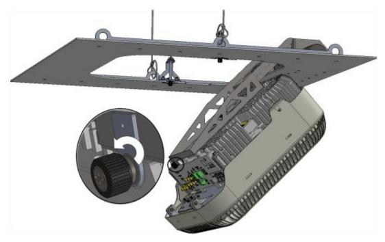
Figure 4-10 Closing Lift Bracket Captive Screw
