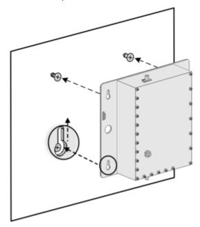
Figure 5-5. Mounting Cavity Filter on Wall
