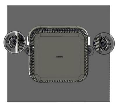
Figure 4-13. Closing Rotary Knobs
