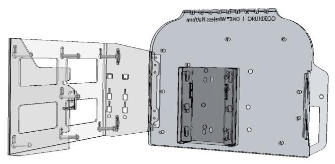
Figure 4-20. Drilling Anchors through Wall-Mountable Bracket Keyholes
