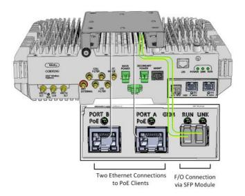
Figure 4-31. GEM Interface Connections
