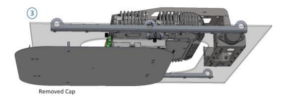
Figure 4-18. Removing Cap
