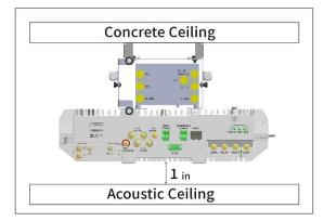
Figure 4-1.Examples of Concrete Ceiling Installation of Mounting Bracket: RAU5x without External Antenna; RAU5x with RxU67 cavity filter.
