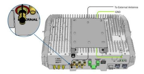
Figure 4-32.RAU5x External Antenna Connection
