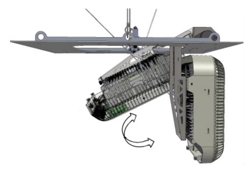
Figure 4-12 Verifying that Cable Path is not Obstructed
