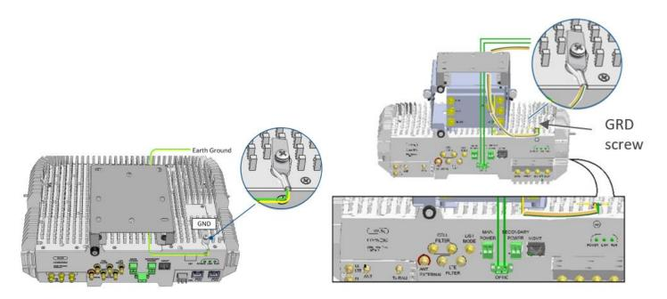
Figure 4-25. RAU5x Grounding and optical fiber pair Connection
