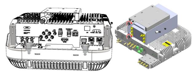
Figure 4-5. Closing Bracket Captive Screw
