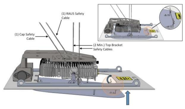
Figure 4-17. Hooking Narrow Fasteners in Place
