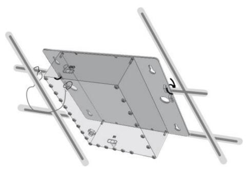
Figure 5-3. Illustration of Cavity Filter Mounted on Acoustic Ceiling Grid
