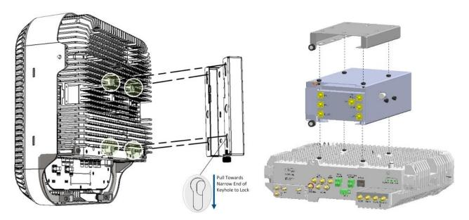
Figure 4-4. Examples of Mounting RAU5x onto Bracket: wall mount; ceiling mount with RxU67 cavity filter
