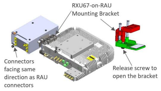
Figure 7-5. Attach cavity filter
