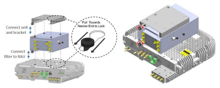
Figure 4-3. Connect Mounting Filter to RAU; Tighten spring-locker
