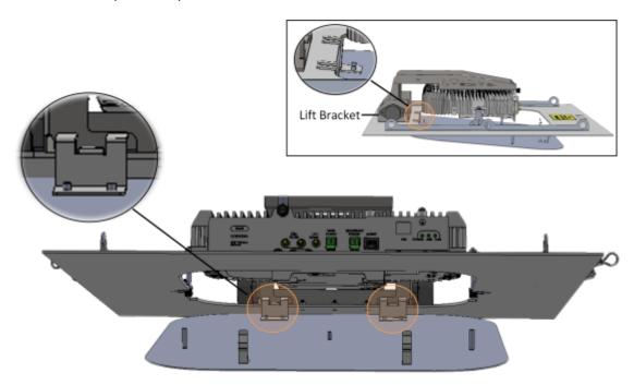
Figure 4-16. Hooking Cap to Top Bracket plate
