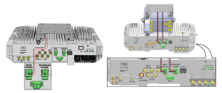
Figure 4-26 RAU5x Main Power DC Connections
