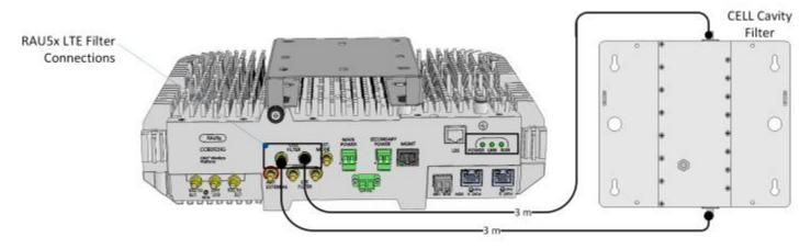
Figure 5-6. Example of RAU5x External CELL Filter Connections
