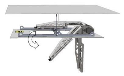
Figure 4-8. Lowering Lift Bracket
