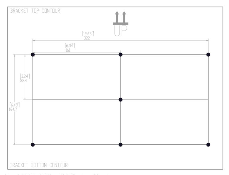
Figure 6-4. RAU5x Wall-Mountable Drilling Pattern Dimensions
