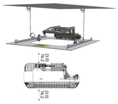
Figure 4-7. Installing "Top Bracket" Plate
