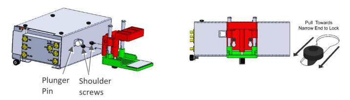
Figure 7-6. Slide bracket on shoulder screws & Secure
