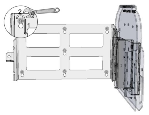
Figure 4-21. Mounting and Securing Bracket to Anchors
