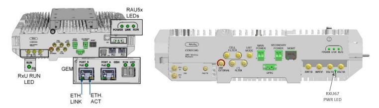
Figure 4-33. RAU5x, RxU67, RxU2325 and GEM LEDs
