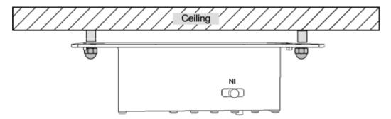
Figure 5-2. Illustration of Cavity Filter Mounted on Ceiling
