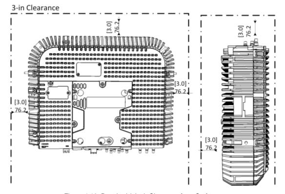
Figure 4-19. Required 3-Inch Clearance from Surface
