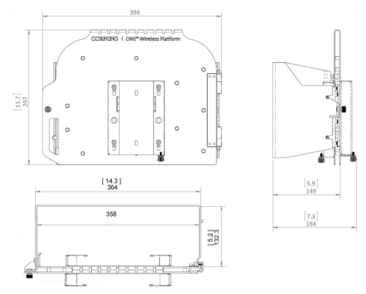
Figure 6-3. RAU5x Wall-Mountable Bracket Dimensions
