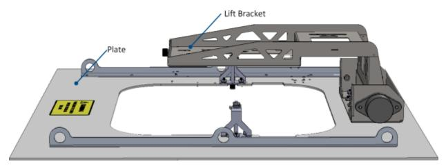
Figure 4-6. "Top Bracket" Assembly Lift Bracket and Plate
