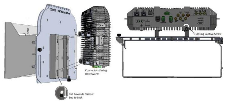
Figure 4-22. Mounting and Securing RAU5x Unit
