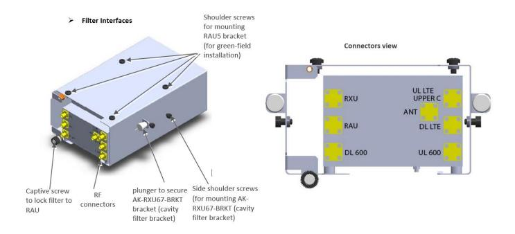
Figure 2-4. RxU67 and Filter Interfaces
