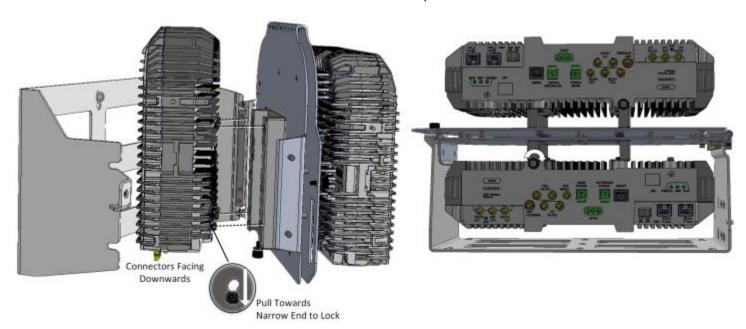
Figure 4-23. Mounting and Securing Second RAU5x
