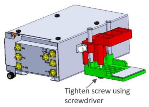
Figure 7-7. Securing Bracket assembled to Cavity filter
