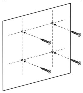
Figure 5-4. Marking and Inserting Anchors in Wall
