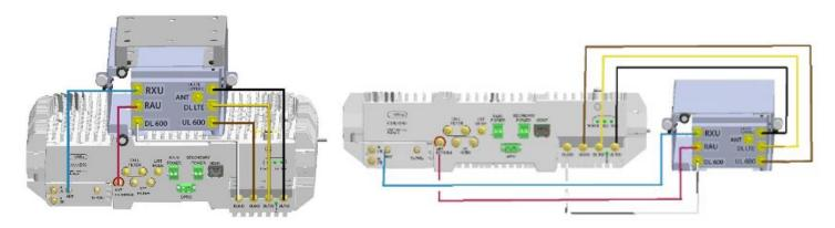
Figure 4-27. RAU5x with RxU67 - Cable Connections to filter
