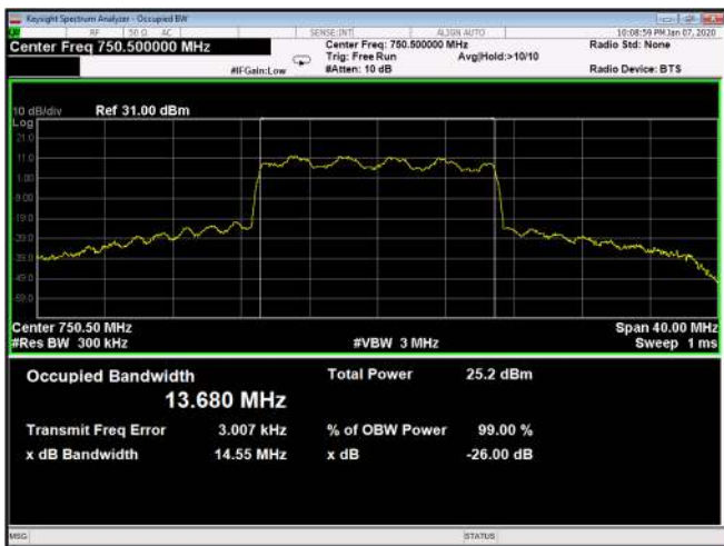
Figure 511: 16QAM 15MHz B.W.; 750.5MHz, 30kHz Output
