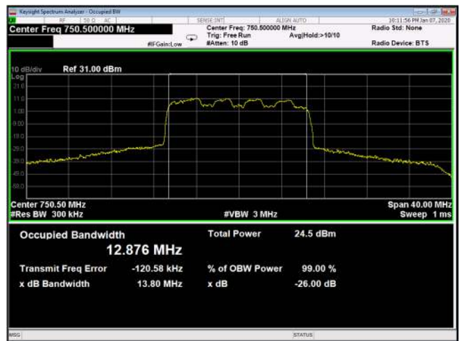
Figure 512: 16QAM 15MHz B.W.; 750.5MHz, 60kHz Output
