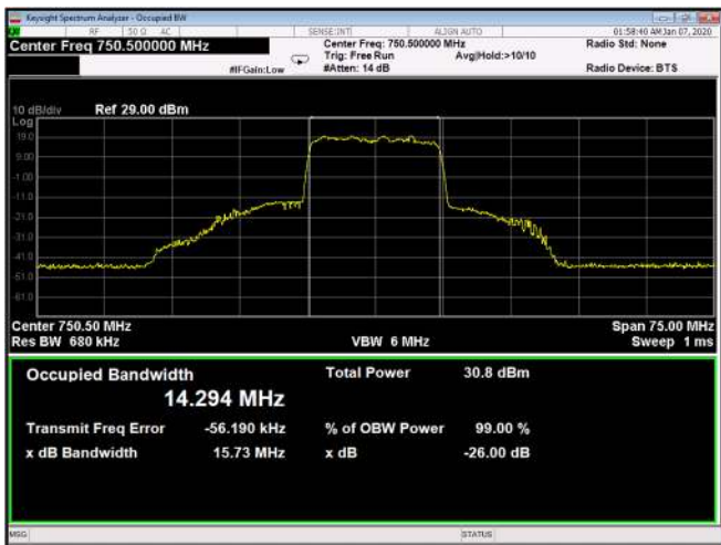
Figure 543: 64QAM 15MHz B.W.; 750.5MHz, 15kHz Output
