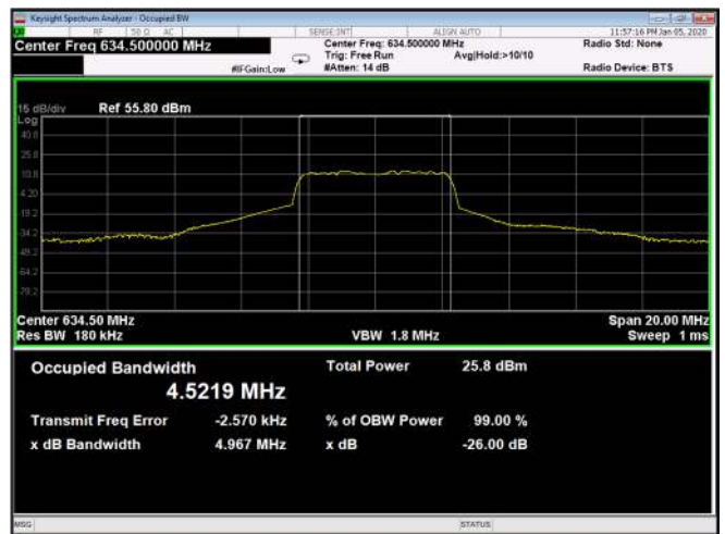
Figure 592: QPSK 5MHz B.W; 634.5MHz, 15kHz Output
