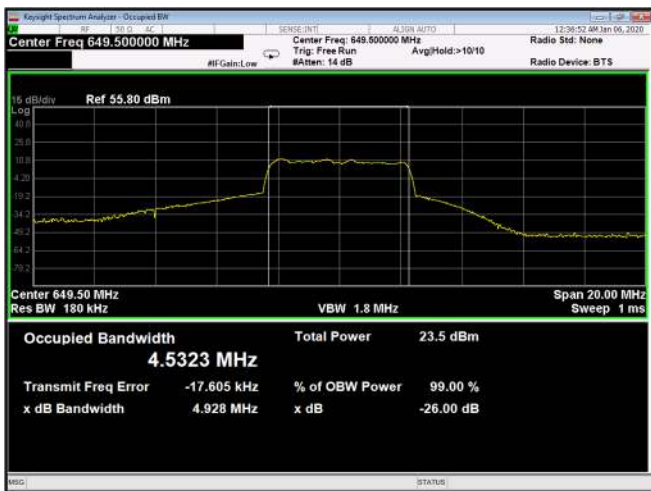
Figure 561: 256QAM 5MHz B.W; 649.5MHz, 15kHz Output
