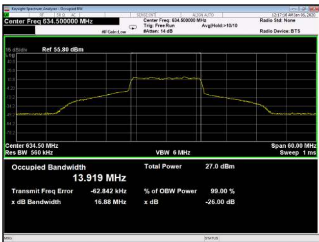
Figure 609: QPSK 15MHz B.W; 634.5MHz, 30kHz Output
