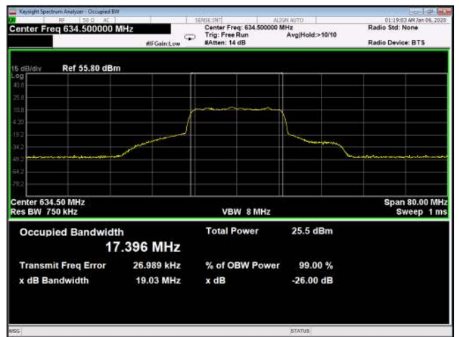
Figure 586: 256QAM 20MHz B.W; 634.4MHz, 60kHz Output
