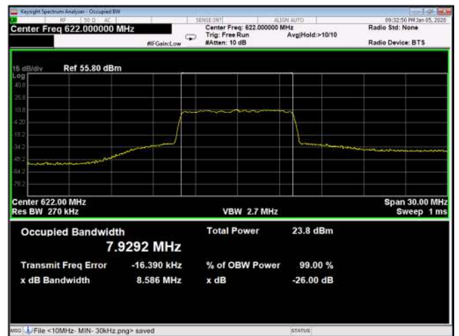
Figure 532: 64QAM 10MHz B.W; 622.0MHz, 60kHz Output
