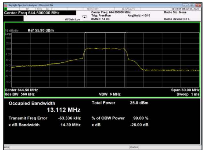
Figure 580: 256QAM 15MHz B.W; 644.5MHz, 60kHz Output
