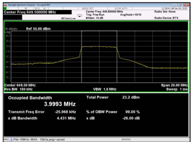
Figure 562: 256QAM 5MHz B.W; 649.5MHz, 30kHz Output
