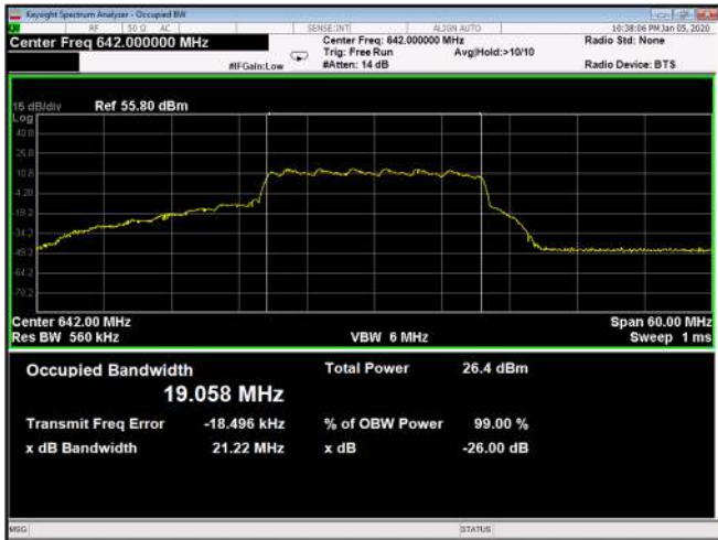
Figure 521: 16QAM 20MHz B.W; 642.0MHz, 15kHz Output
