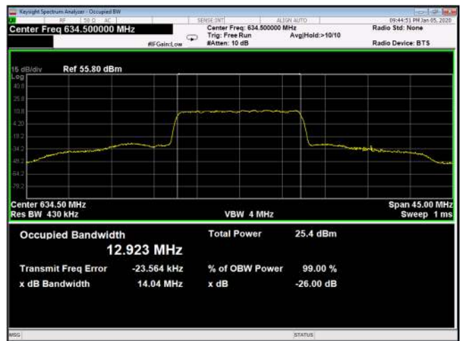
Figure 544: 64QAM 15MHz B.W; 634.5MHz, 60kHz Output
