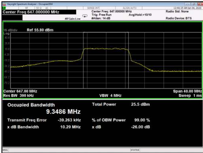
Figure 569: 256QAM 10MHz B.W; 647.0MHz, 15kHz Output
