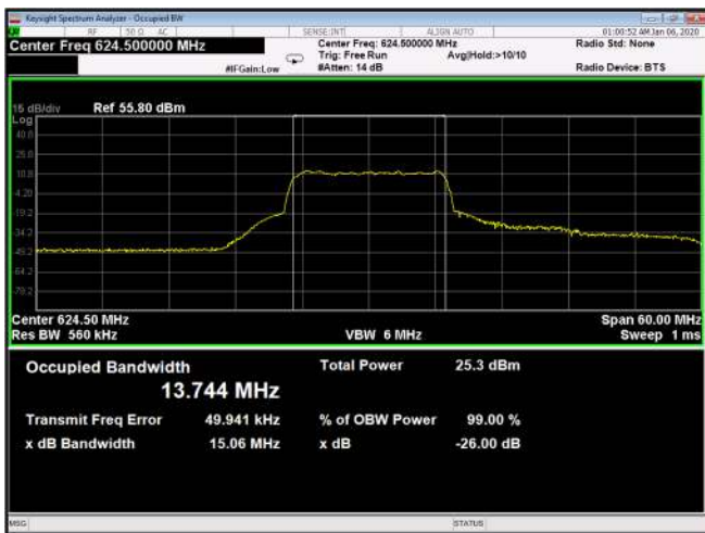
Figure 573: 256QAM 15MHz B.W; 624.5MHz, 30kHz Output
