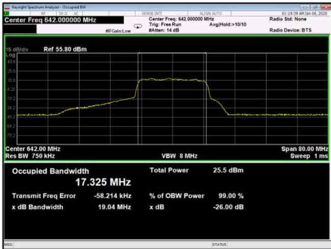
Figure 589: 256QAM 20MHz B.W; 642.0MHz, 60kHz Output
