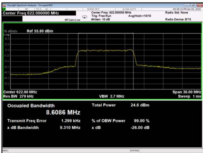
Figure 531: 64QAM 10MHz B.W; 622.0MHz, 60kHz Output
