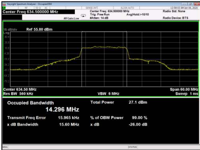
Figure 575: 256QAM 15MHz B.W; 634.5MHz, 15kHz Output
