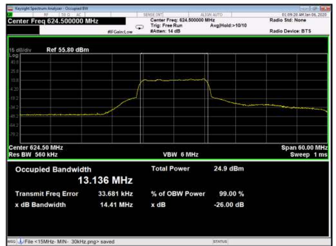
Figure 574: 256QAM 15MHz B.W; 624.5MHz, 60kHz Output
