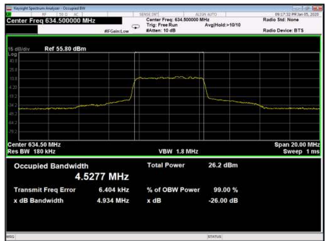
Figure 526: 64QAM 5MHz B.W; 634.5MHz, 15kHz Output
