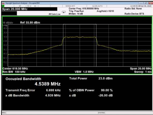
Figure 557: 256QAM 5MHz B.W; 619.5MHz, 15kHz Output
