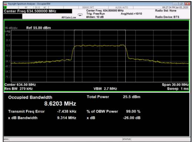
Figure 534: 64QAM 10MHz B.W; 634.5MHz, 30kHz Output
