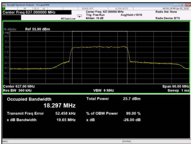
Figure 549: 64QAM 20MHz B.W; 627.0MHz, 30kHz Output
