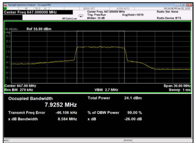
Figure 538: 64QAM 10MHz B.W; 647.0 MHz, 60kHz Output
