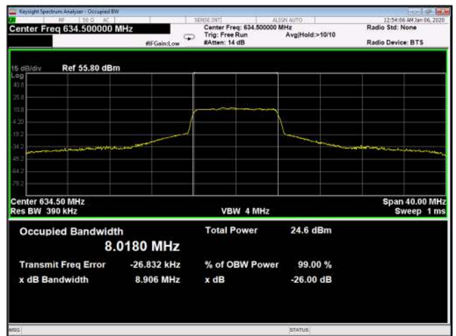
Figure 568: 256QAM 10MHz B.W; 634.5MHz, 60kHz Output
