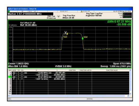
Figure 65. — Out-of-Band Rejection Plot
