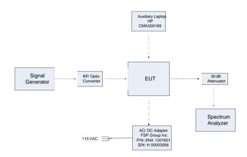
Figure 1. Test Set-Up - Conducted
