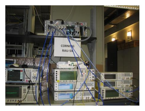
Figure 9. Intermodulated Conducted Emission Test
