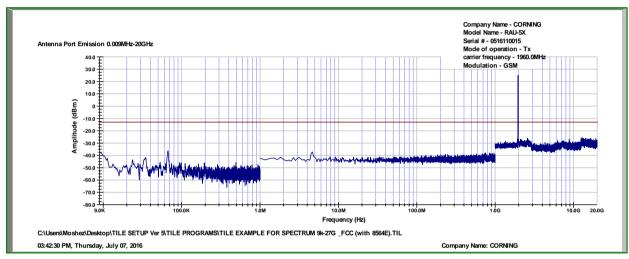
Figure 45. — GSM - 1960.0 MHz
