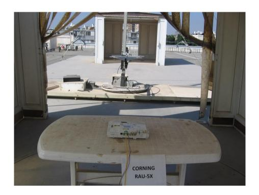
Figure 5. Radiated Emission Test
