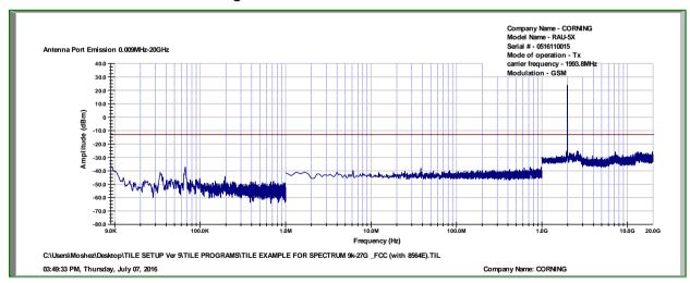
Figure 46. — GSM - 1993.8 MHz
