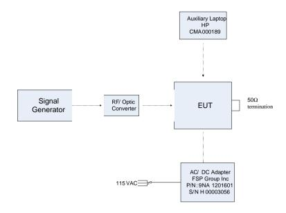
Figure 2. Test Set-Up - Radiated
