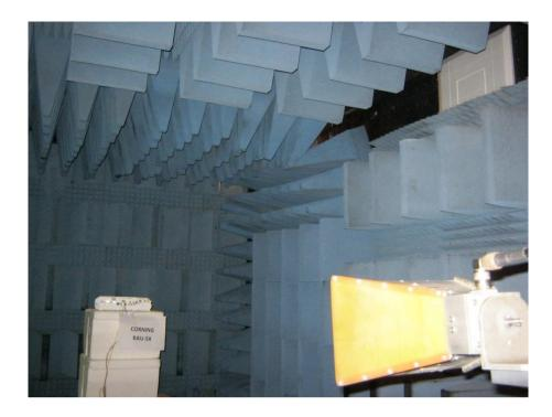
Figure 7. Radiated Emission Test
