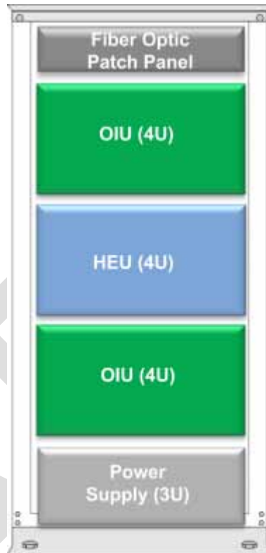
Figure 4-1. Example of Communication Rack Installation
