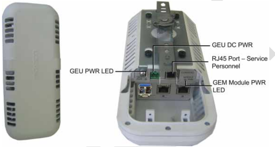
Figure 3-8. GEU Enclosure: Top (Left) and Open Underside (Right)
