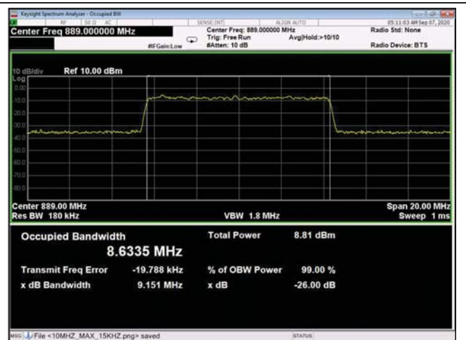
Figure 231: 64QAM 10MHz B.W.; 889.0MHz, 30kHz - Input
