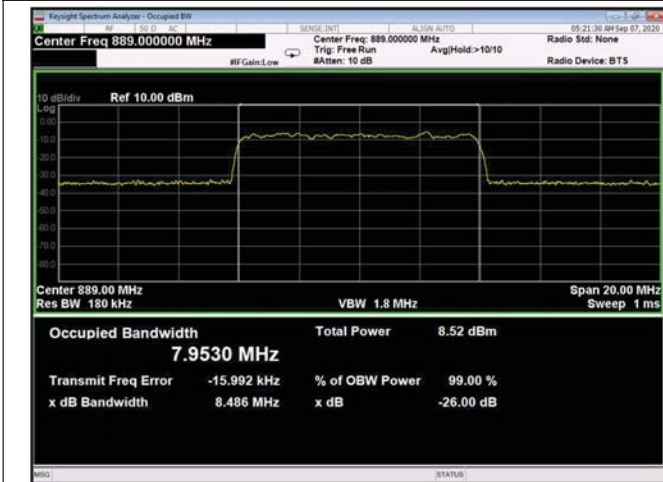
Figure 232: 64QAM 10MHz B.W.; 889.0MHz, 60kHz- Input
