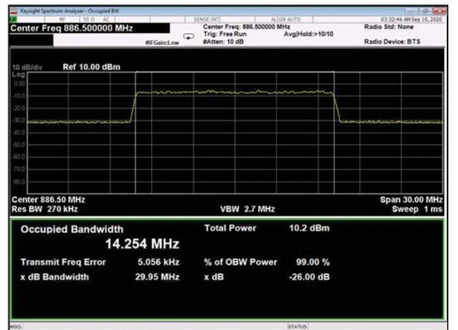
Figure 281: 256QAM 15MHz B.W.; 886.5MHz, 15kHz - Input
