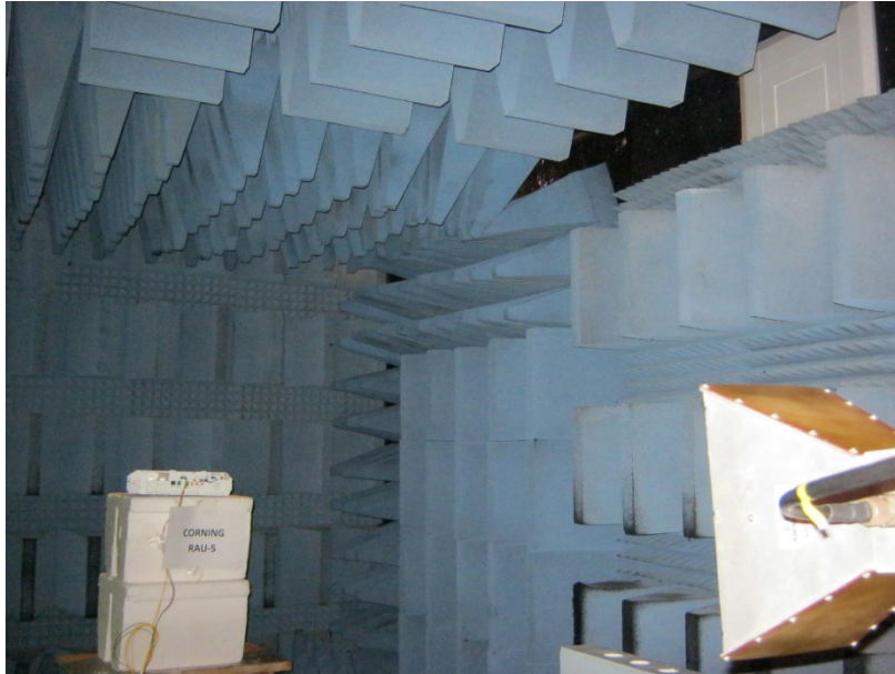
Radiated Emission Test 1-18GHz
