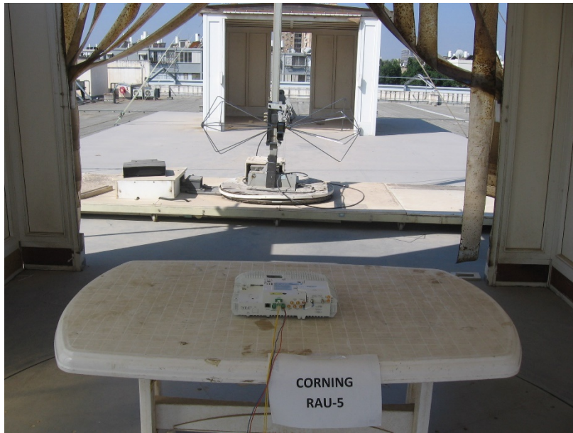
Radiated Emission Test 30 - 200 MHz
