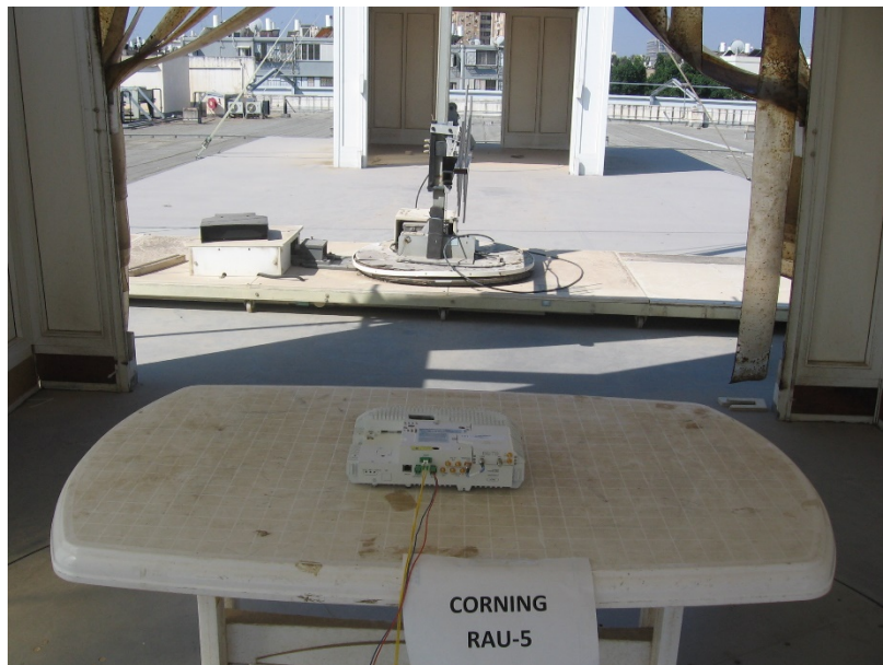
Radiated Emission Test 200 - 1000MHz
